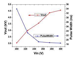
Figure 5. Output pulse amplitude and width vs different charging voltage
