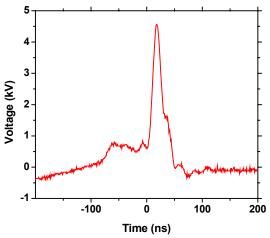
**Figure 3.** Output pulse to the cuvette load: 4.56 kV, 18.4 ns FWHM
