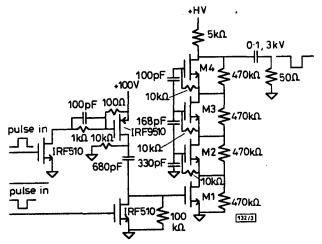
Fig. 3 Schematic diagram of 1500 V pulse generator designed using the techniques presented
