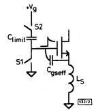
Fig. 2 Simplified schematic diagram of gate driver circuitry
