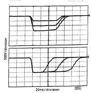
Fig. 4 Output of pulse generator with varying amplitudes and pulse widths
