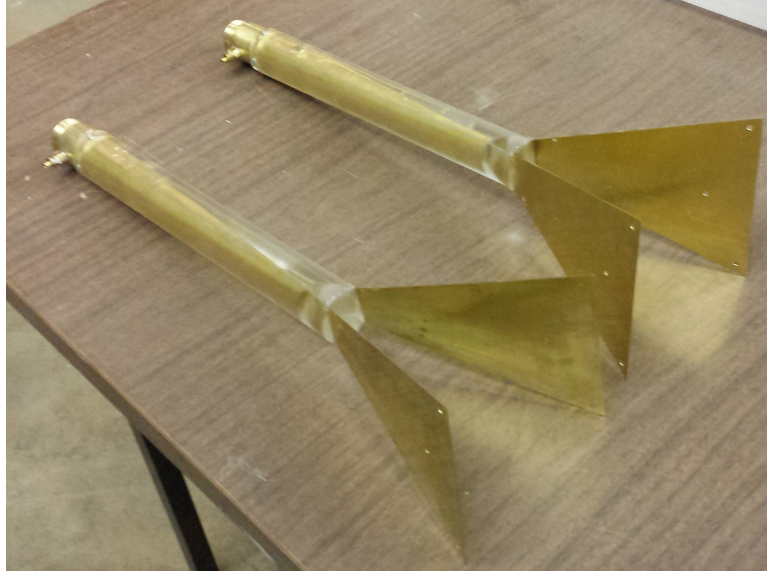
Figure 5.2: Two fabricated TEM horn antennas used for array testing.
