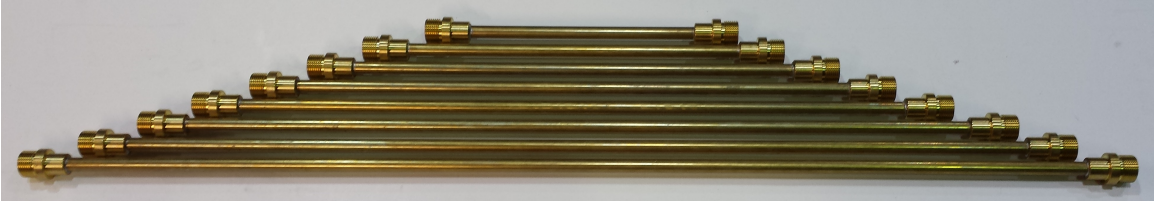
Figure 4.6: Different length shells used for line length testing
