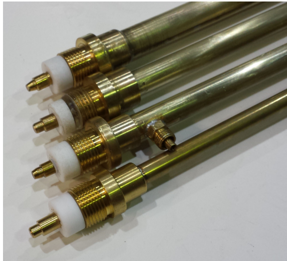
Figure 3.3: Different NLTLs: from top to bottom, EFI, Sylgard, Gas fed SF 6 , latest SF 6 .
