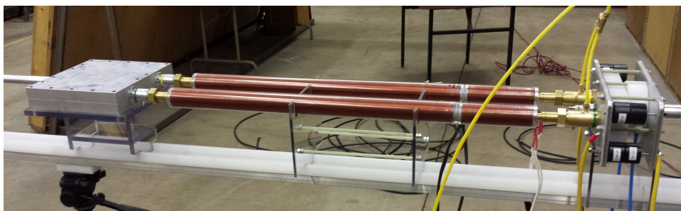
Figure 4.39: Combiner test setup.
