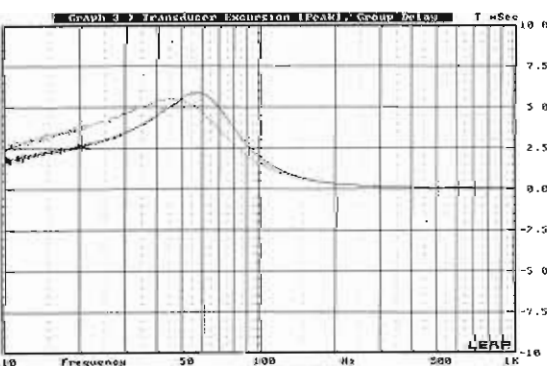
FIGURE 12.85: Comparison of group-delay curves for the 2.83V curve in Fig. 12.84.
