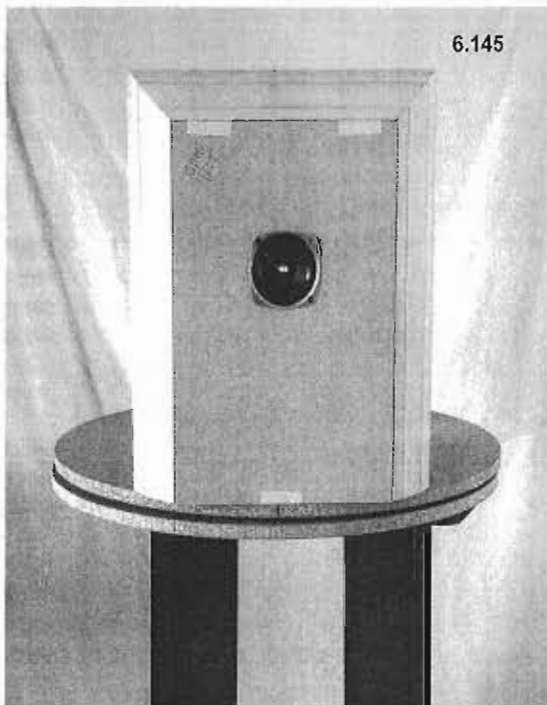
FIGURE 6.145: Picture of the compound beveled edge baffle for diffraction subjective Test #3.
