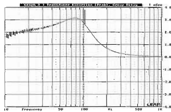
FIGURE 12.51: Group-delay curve for the 2.83V curve in Fig. 12.50.
