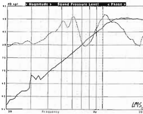
FIGURE 11.10: Comparison of free-field and closed-field frequency response measurements of speaker used for closed-field simulation in Fig. 11.8.
