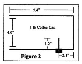
strips at a local hobby store. The tubing will slide over the N center pin. Al Ward prefers to use two pieces of tubing, one smaller than the other. The smaller piece to be soldered to the center pin and the other telescoping over and soldered to the smaller one. This will allow increasing or decreasing the length of the probe for tuning.
