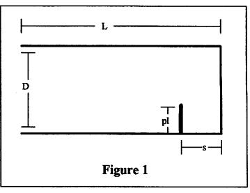
affect this distance, most notably diameter and length of the horn. My experience has been to place the radiating element about  $0.4\lambda$  from the closed end.
