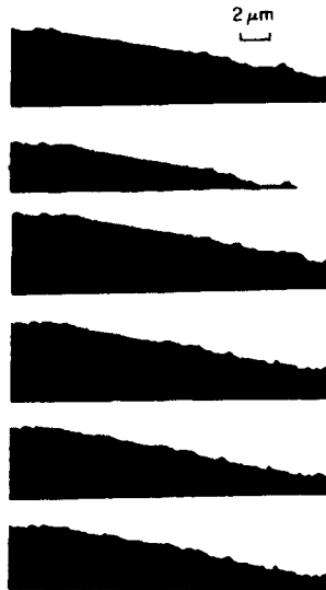
Fig 3.7 A sequence of micrographs showing how the profile of an electrode surface is progressively damaged following successive 20 μs, breakdown-inducing high voltage pulses. (From Latham and Chapman [18], with permission.)
