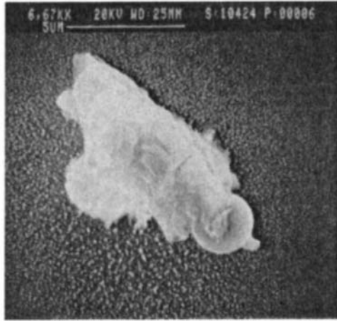
Fig 12.18 An indium particle only partially molten. There was no starburst associated with this particle.
