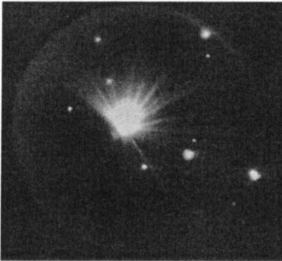
Fig 1.1 A high speed video image illustrating the "explosive" nature of a vacuum breakdown event.
