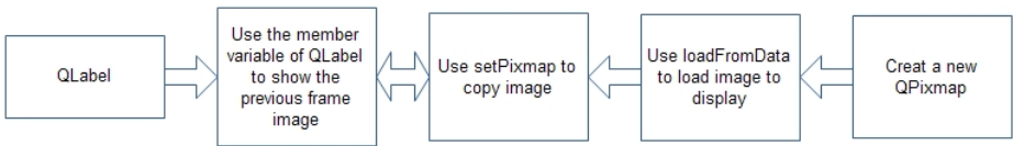
Fig. 2. Double buffering mechanism
