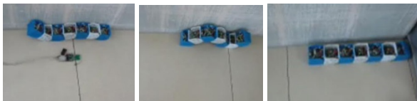
Fig. 9. Locomotion of worm-shaped configuration by optimized CPG signals
