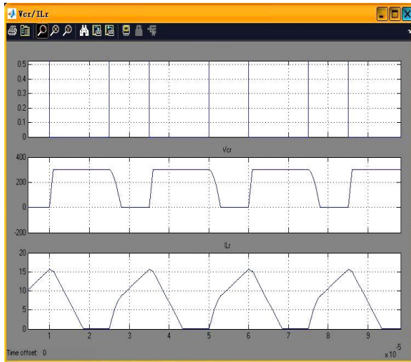
Fig. 7. The waveform analysis of capacitor voltage and inductor current
