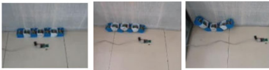
Fig. 8. Locomotion of worm-shaped configuration by pre-optimized CPG signals
