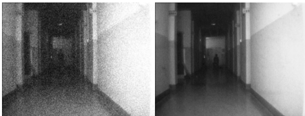
Fig. 1. LLL image and LLL image processed by time-domain recursive filtering.
