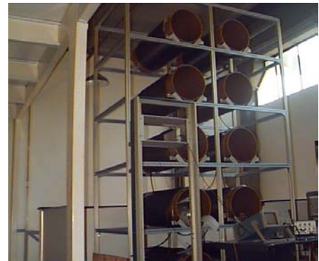
Figure 3. Picture of the pulser structure assembling.
