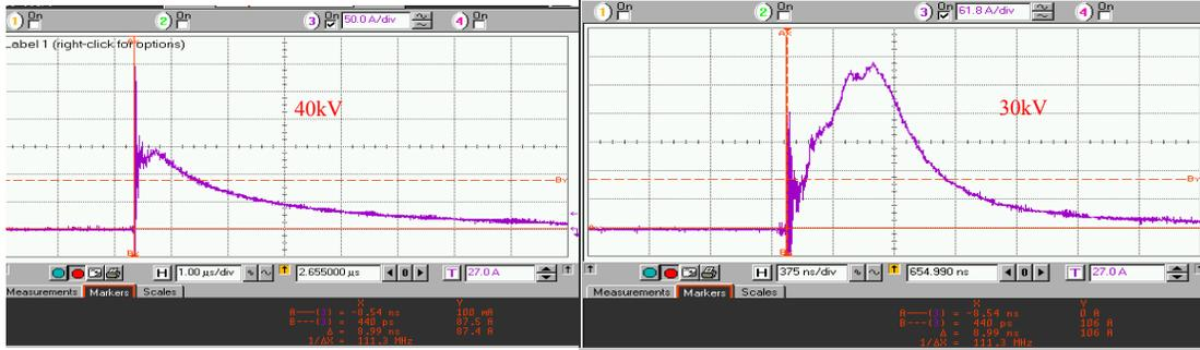
Figure C.2 - Internal break-down of HVR resistors, peak amplitude of 130 A and 350 A, respectively.
