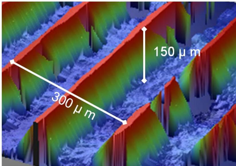
Figure 3.29 - Optical interferometer image of 150 μm depth aluminum cathode
