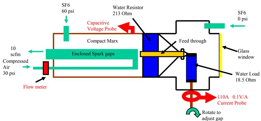
Figure 3.33 - Cross sectional view of water load setup with air inputs, various parts, and probes
