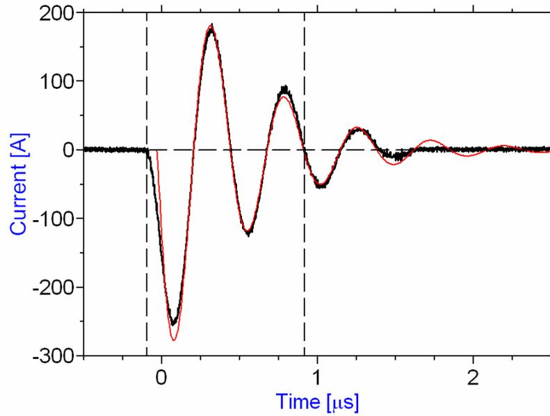
Figure 4.11 - Matching of P-Spice model to experimental waveform of 20 stage CMG into short
