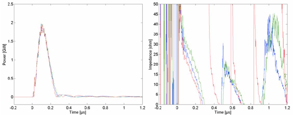
Figure 4.21 – Power and impedance of HPM system at 21 kV charging using a Vircator load with 9mm (green), 10mm (blue), and 11mm (red) AK-gap.
