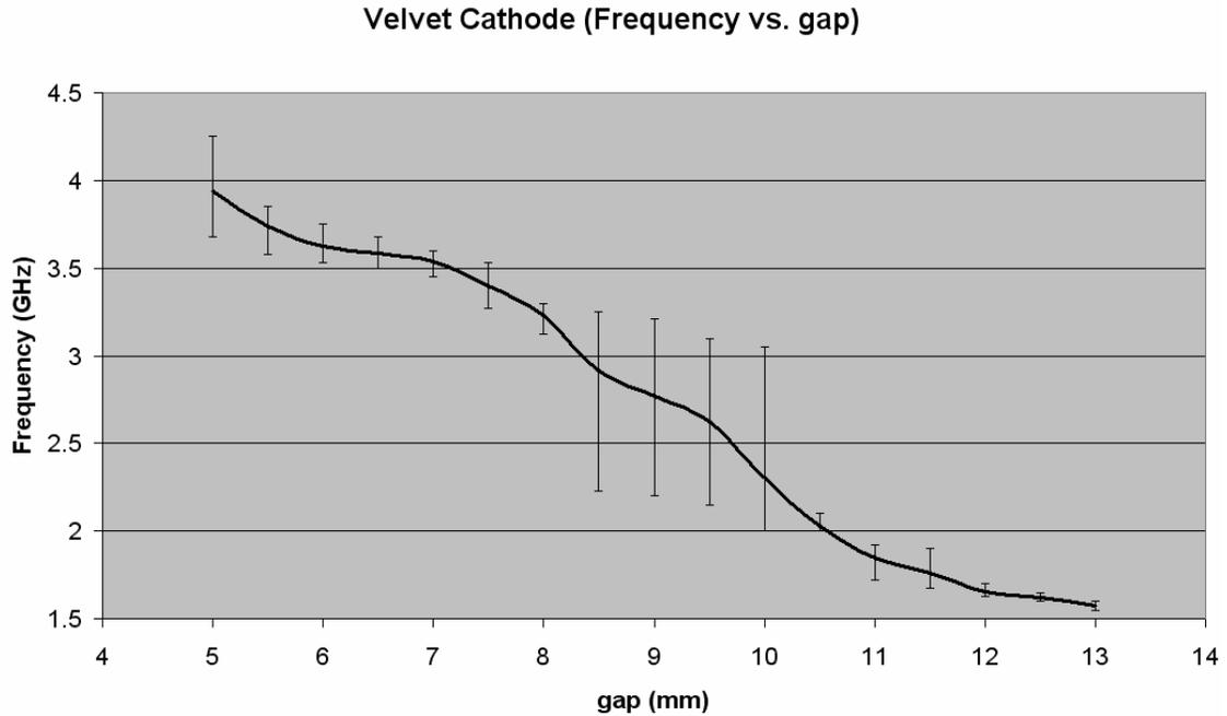
Figure 4.30 – Microwave frequency vs. gap distance of velvet cathode over 4 sets of data.
