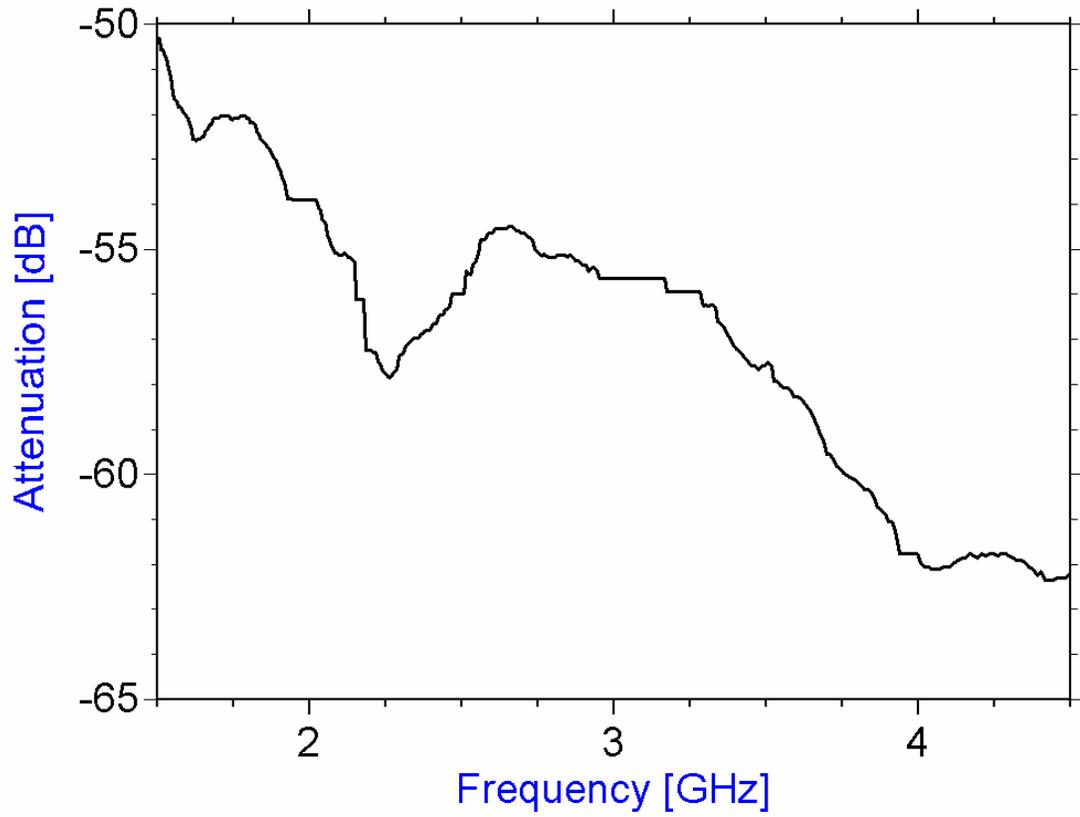
Figure F.1 - Attenuation of 10 m section of RG58 coaxial cable
