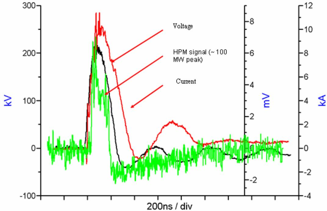
Figure 4.19 – Voltage, current, and HPM from 20 kV charging, single shot with Vircator set at 10mm gap.
