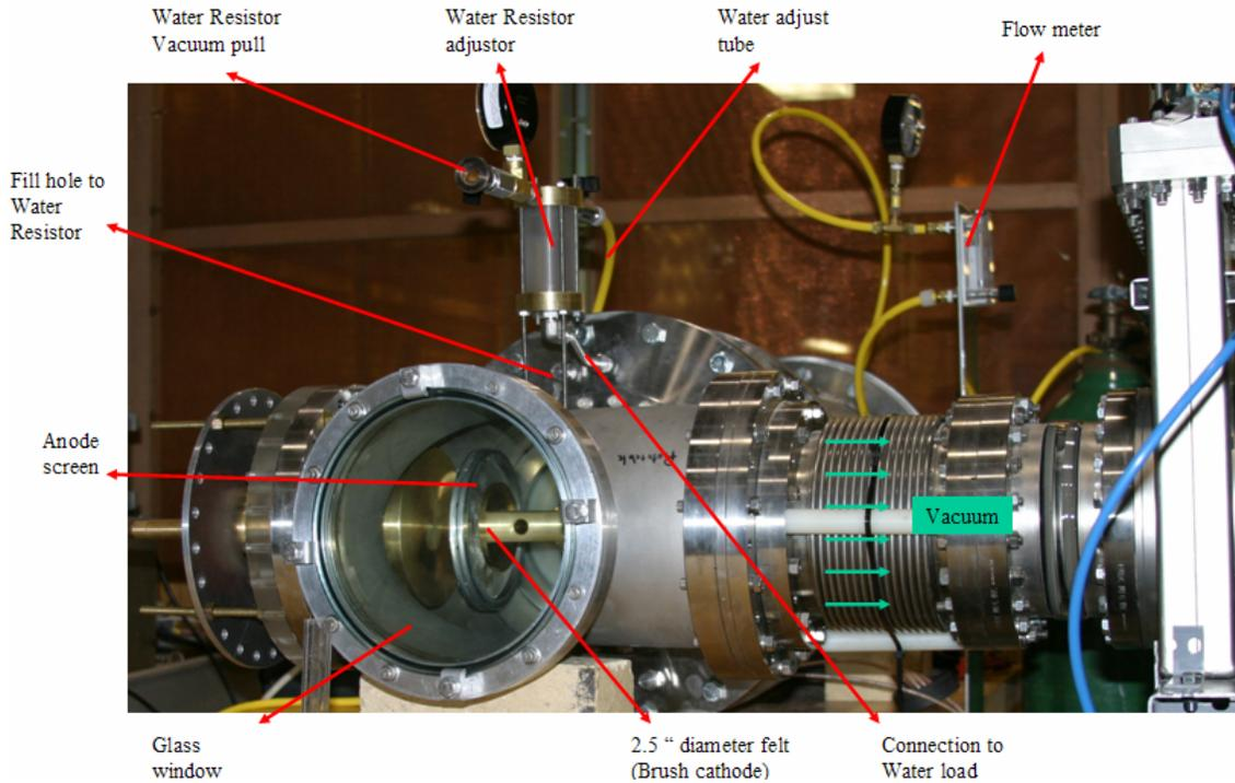
Figure 3.37 - Front view of HPM system with Vircator operation setup.
