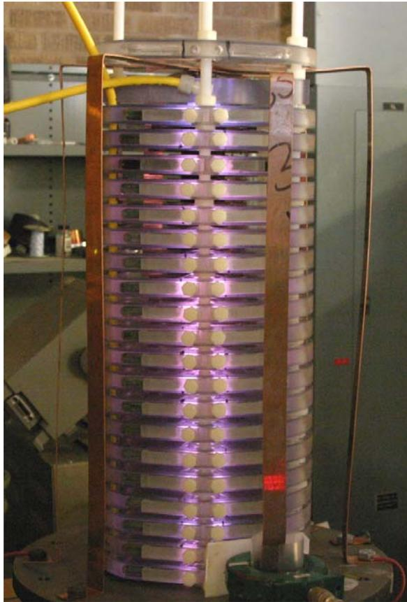
Figure 4.9 - 20 stage CMG fired into short at low charging voltages.
