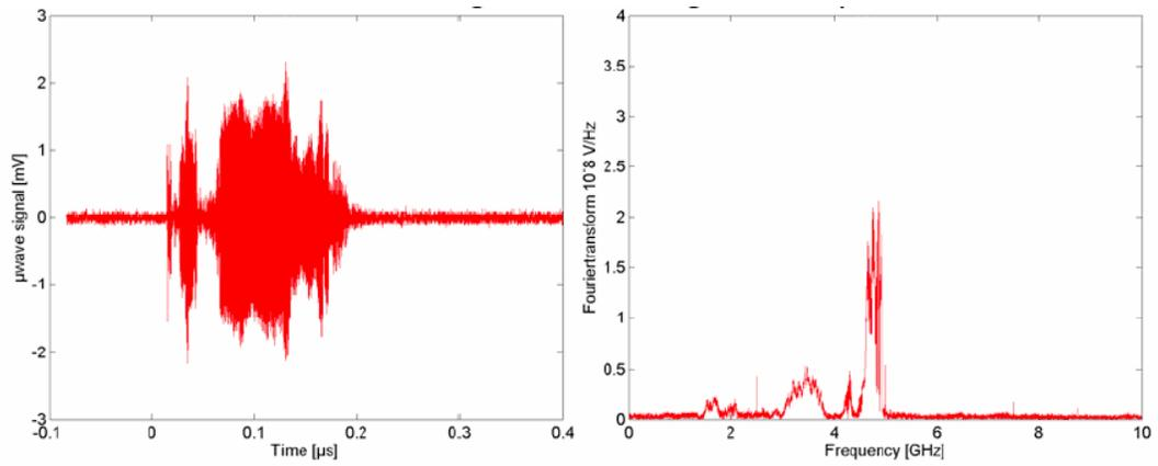
Figure 4.22 – Microwave signal and FFT of HPM system at 21 kV charging with 9 mm A-K gap.
