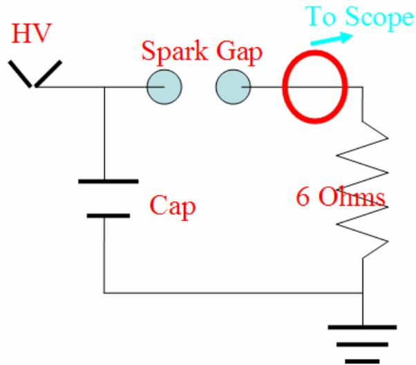
Figure 4.1 - Capacitor testing setup
