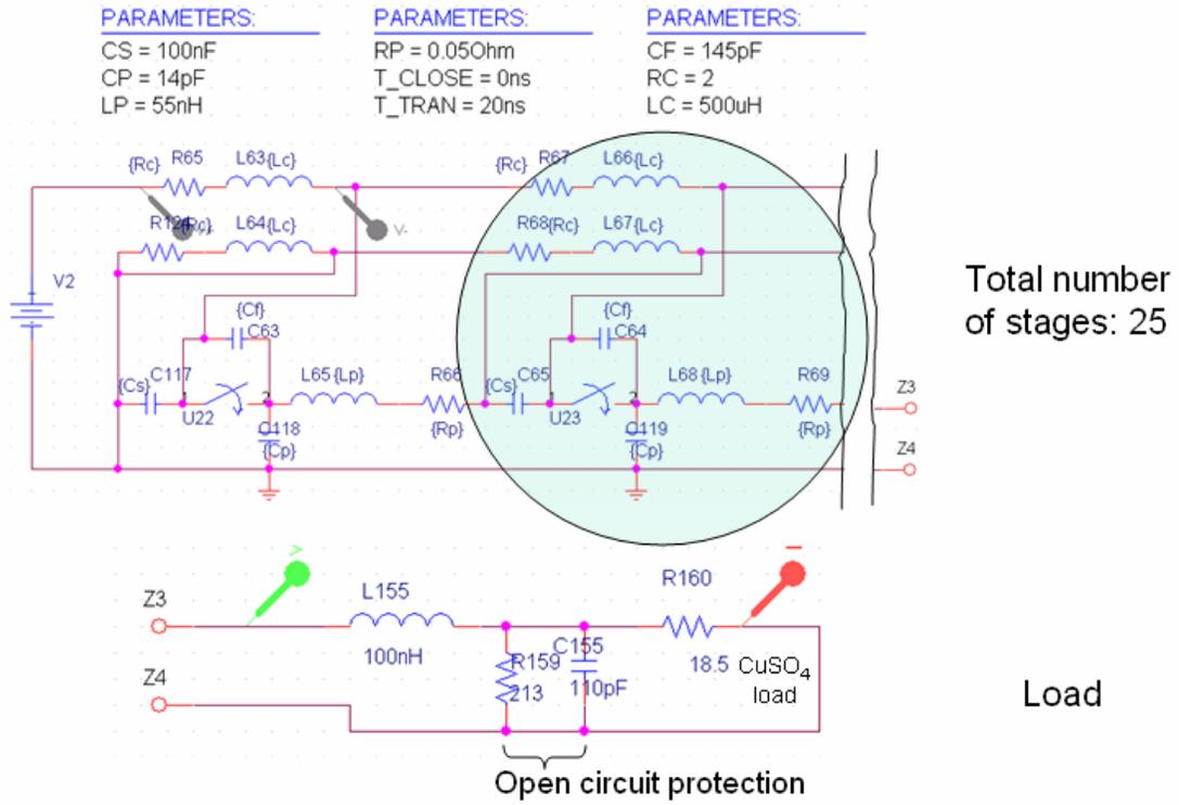
Figure 4.17 - P-spice modeling of the electrical characteristic of the full 25-stage CMG model fired into an 18.5  $\Omega$  water load
