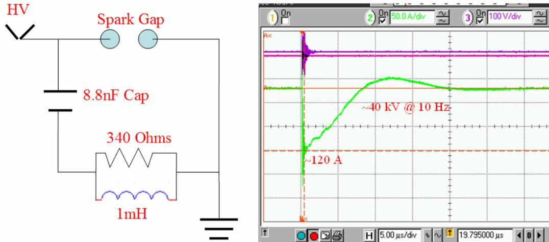
Figure 4.3 – Inductor Testing setup and waveform
