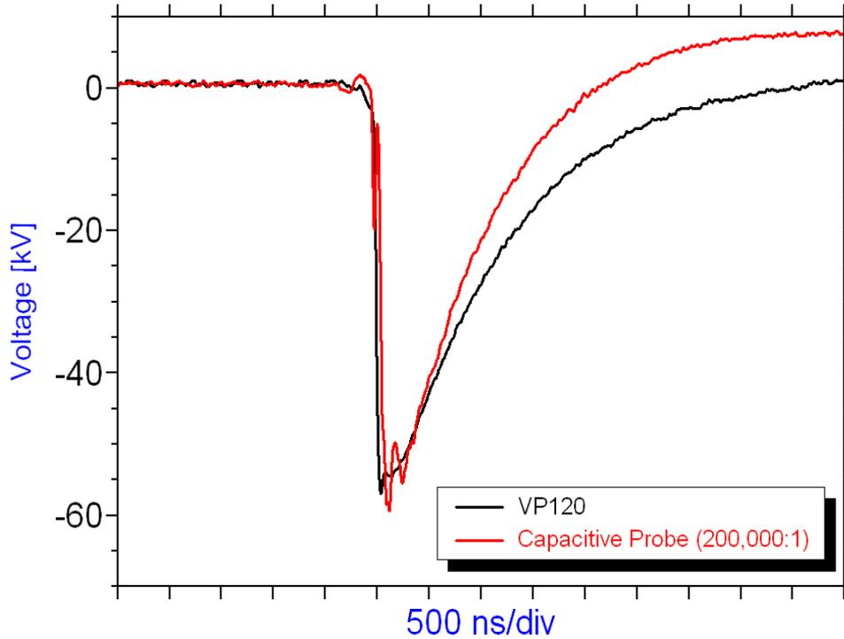
Figure 3.14 – Wave form matching between VP120 probe and the capacitive voltage probe.
