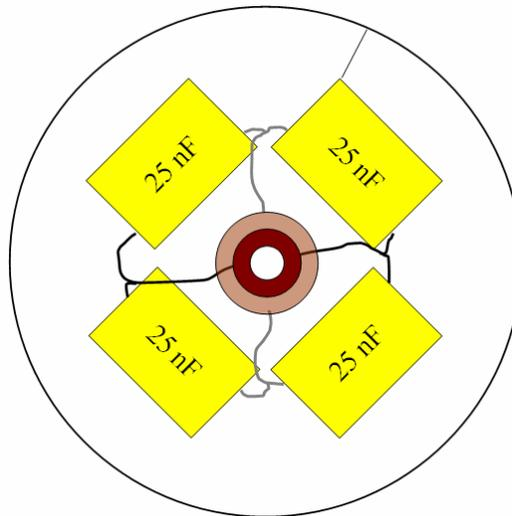
Figure 3.6 – Early capacitor setup for single Marx stage
