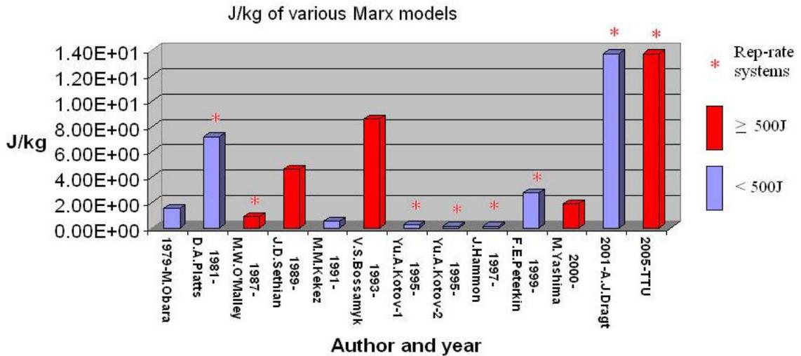
Figure 2.3 – Energy density in J/m<sup>3</sup> of various Marx designs
