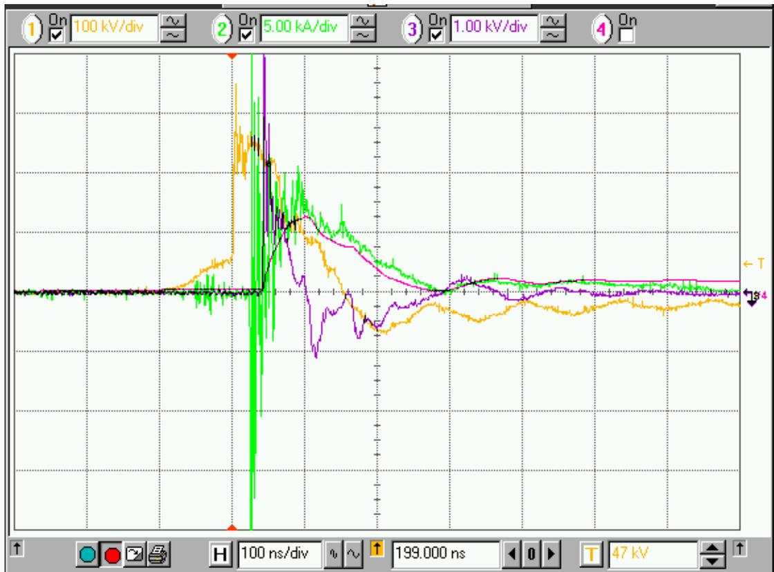
Figure 4.29 - Diagnostic waveforms of voltage (yellow), current from Pearson coil (green), waveform of Rogowski coil (purple), and Integral of Rogowski coil waveform (pink).
