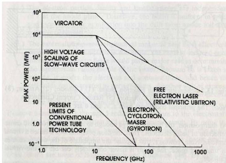
Fig. 13.1 Projected Limits of Ultra-High-Power Microwave Source (<100 ns) Technology (Courtesy of R. Parker).
