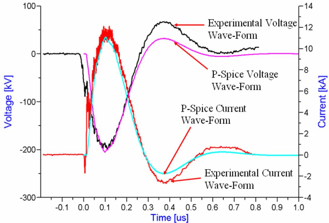
Figure 4.18 - Wave matching of Marx model at 17 kV to measured output waveform with water load of ~20 kV charging, 10 Hz shot, with rapid charger.
