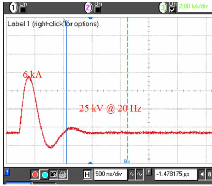
Figure 4.2 - Mica-Capacitor @ 24 kV, 20 Hz waveforms
