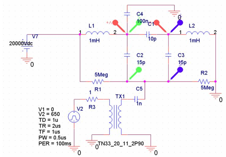
Figure 4.6 – Solid state Marx triggering simulation circuit
