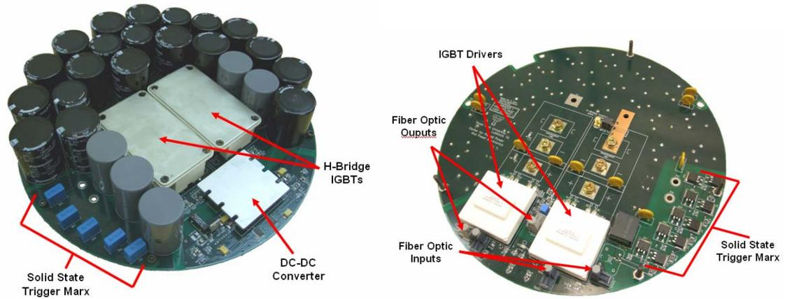
Figure 3.2 – Inverter PCB board
