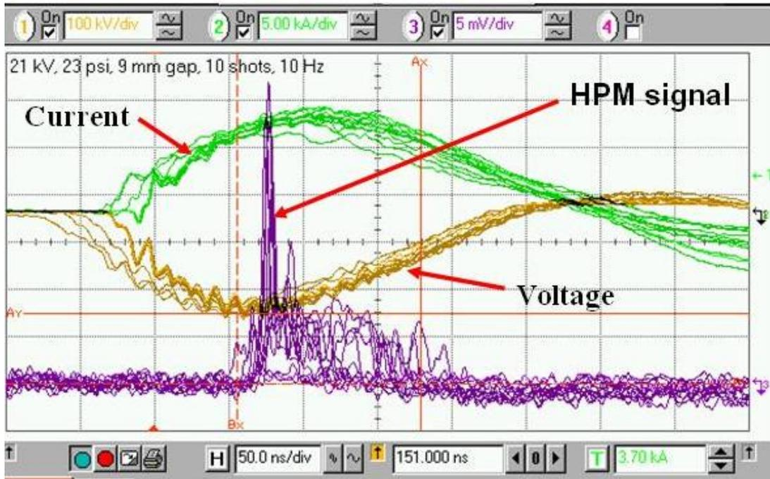
Figure 4.25 - Screen shot of diode power, voltage, and current wave-forms of a burst of 10 shots at ~10 Hz.
