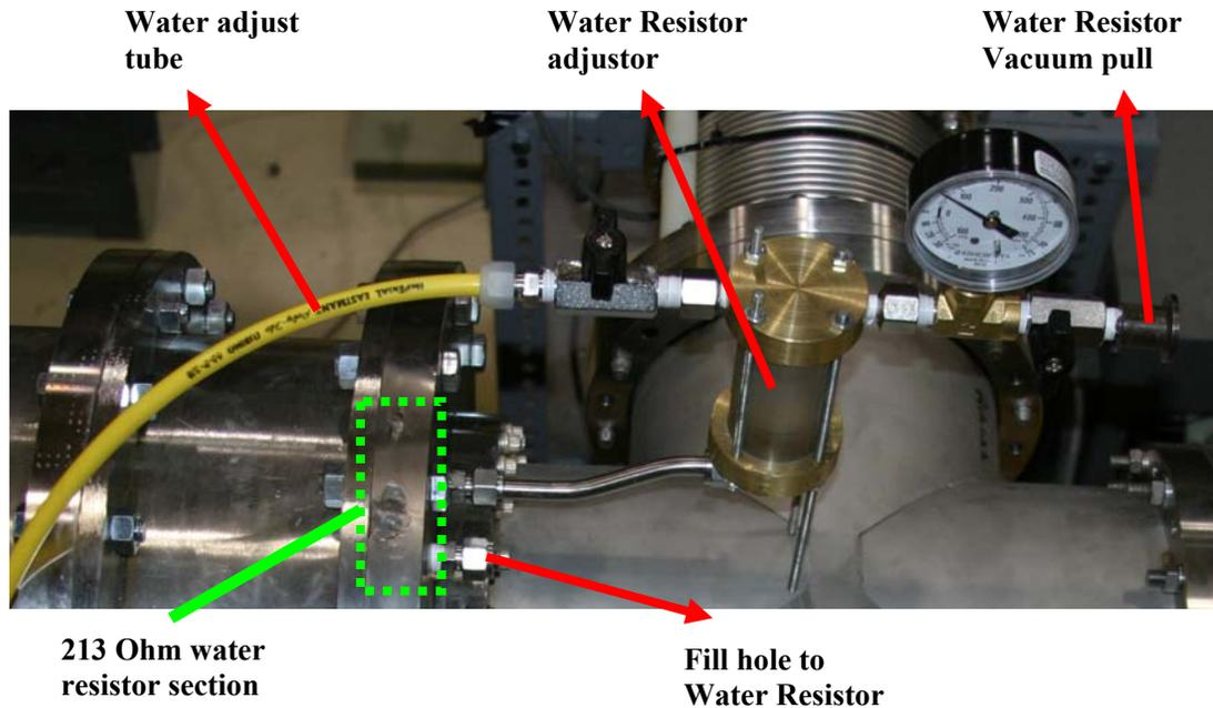
Figure 3.21 - Water resistor setup and various adjusting parts
