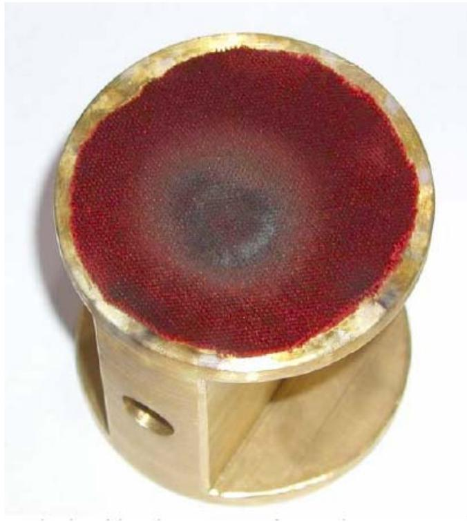
Figure 3.27 – Used cathode with velvet attached
