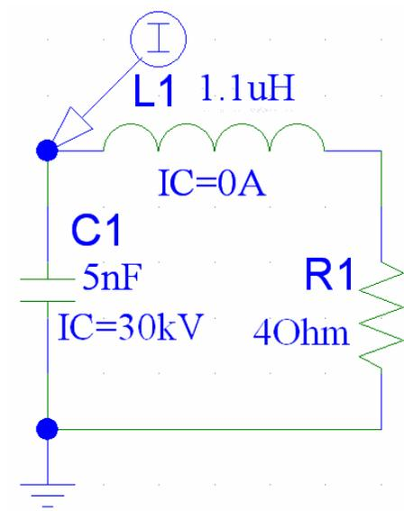
Figure 4.10 - Lumped element representation of 1.5 kV charging, 20 stage CMG into short.
