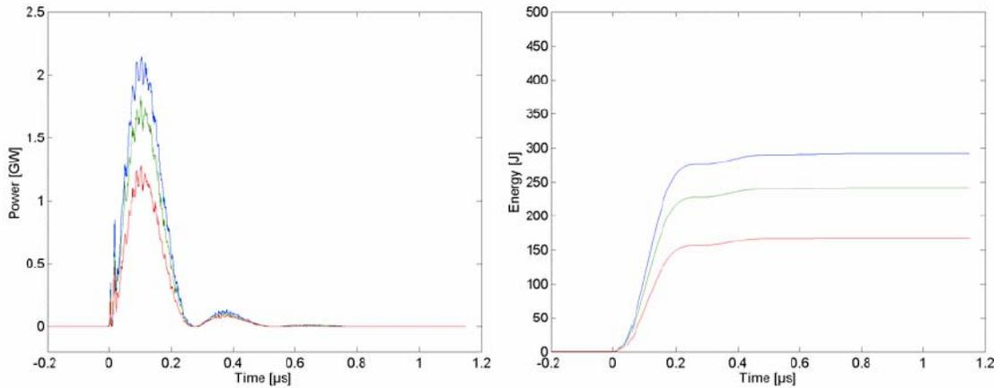
Figure 4.15 - Power and energy of HPM system into an 18.5 Ohm water load with 15, 17.5, and 20 kV charging.
