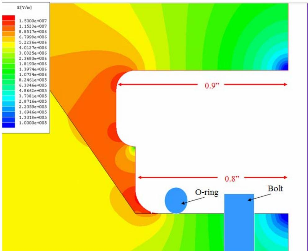
Figure 3.24 - New flange connection and field shaping design for triple point 2.
