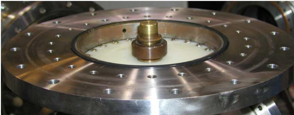
Figure 3.20 - Coaxial water load section
