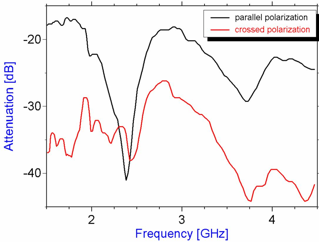
Figure F.2 - Attenuation of parallel and crossed polarization of the Horn adaptor.
