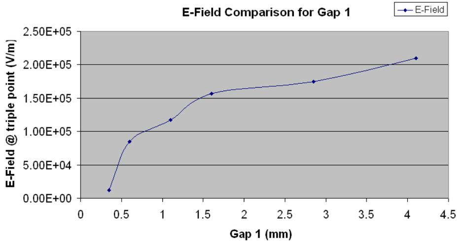
Figure 3.23 – Variance of field strength at triple point 1 vs. gap spacing
