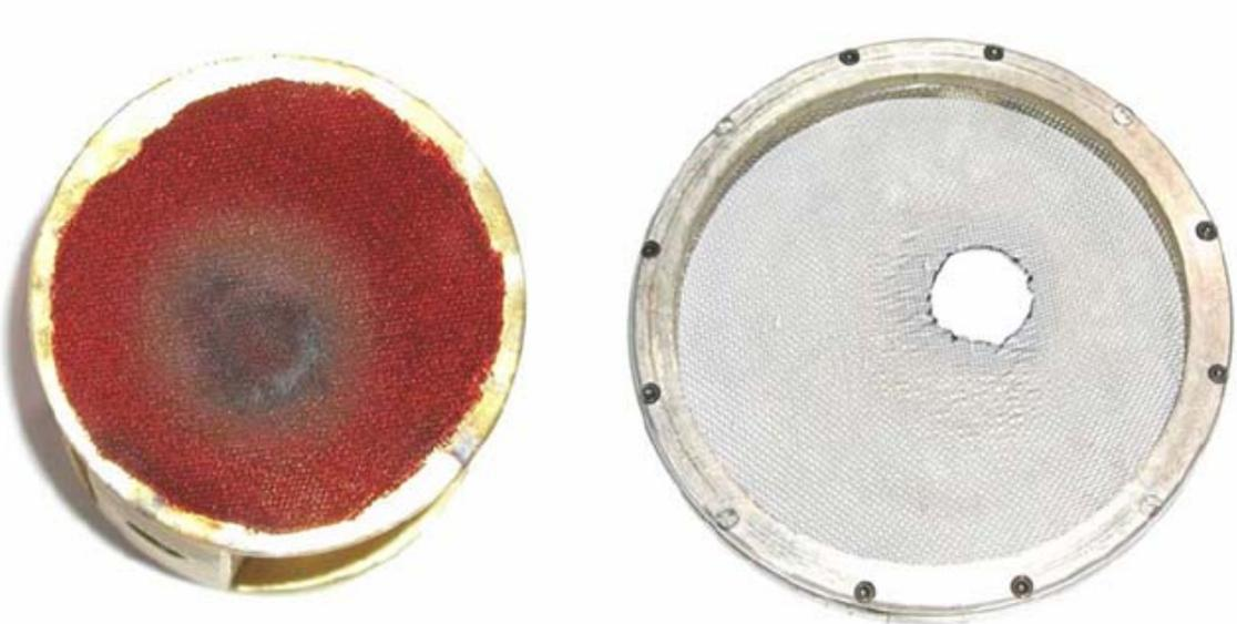
Figure 4.26 - Damage to velvet cathode and screen anode after continuous repetitive operations.
