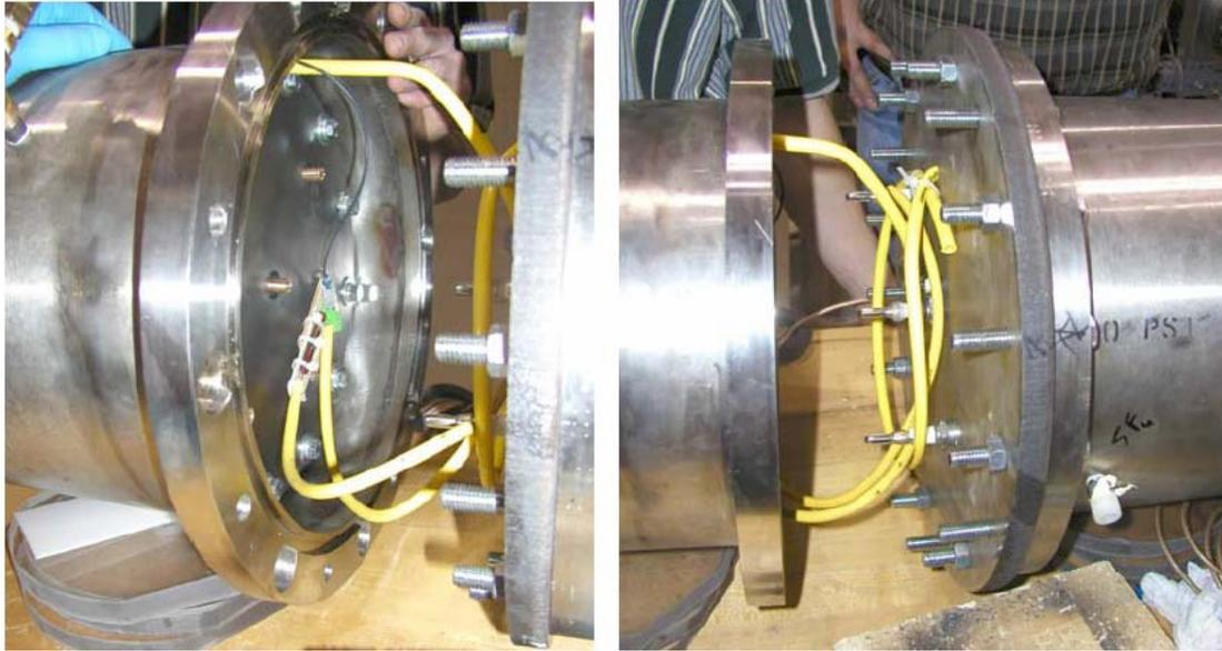
Figure 3.3 – Connection between the rapid charger and the CMG.
