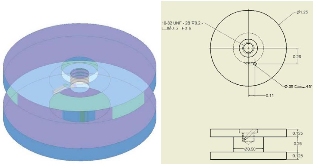
Figure 3.7 - Lexan inductor casing
