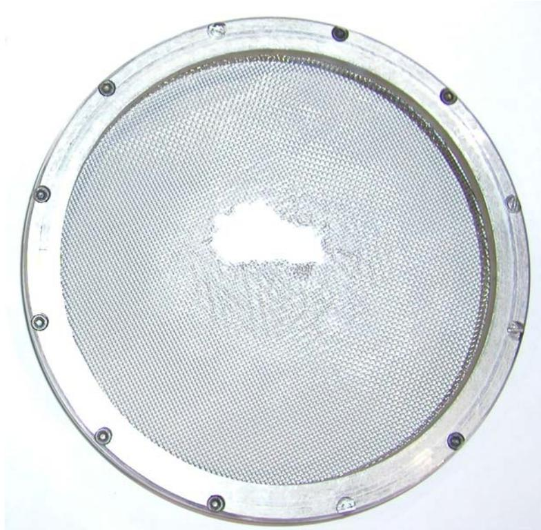
Figure 3.31 – Used screen anode constructed with steel mesh
