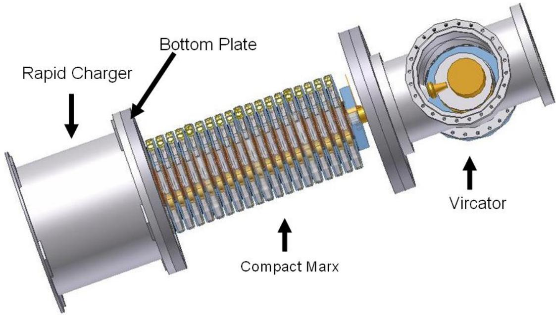
Figure 1.2 - Complete HPM system. Overall length ~ 150 cm. Main diameter ~ 30 cm.
