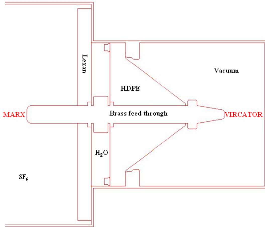
Figure 3.18 – Cross section of the redesigned HV feed-through from the Marx to the Vircator with protection water resistor section.
