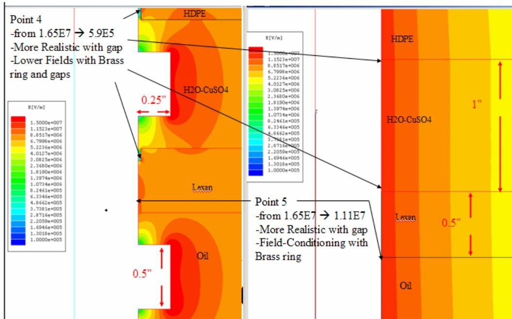
Figure D.4 - Field shaping of base design
