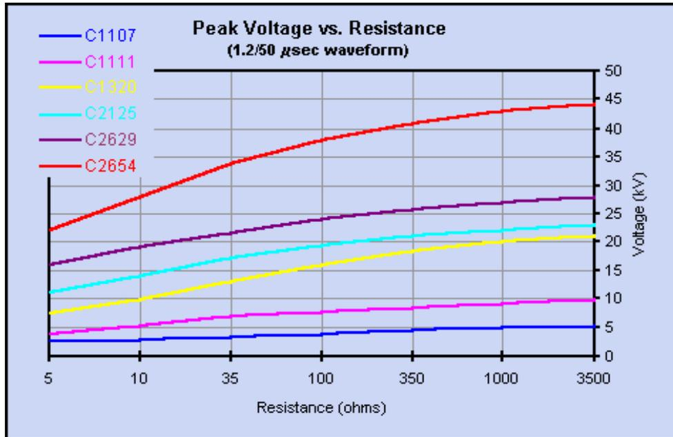
Figure B.2 – Peak Voltage vs. Resistance (<http://www.hvrpc.com/products/c/index.html>)
