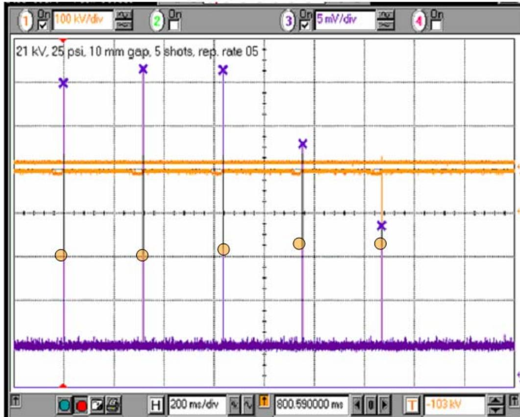
Figure 4.27 - Peak detect of diode power and voltage signals at 3 Hz
