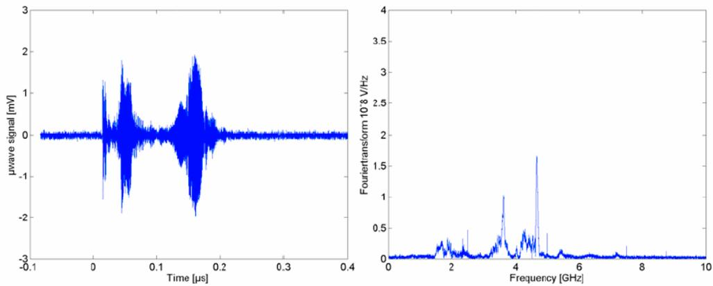
Figure 4.23 - Microwave signal and FFT of HPM system at 21 kV charging with 10 mm A-K gap.
