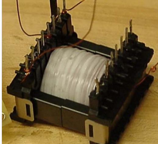
Figure 3.4 - Trigger Transformer
