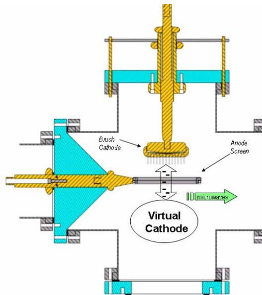
Figure 3.39 - Reflex Triode Vircator configuration
