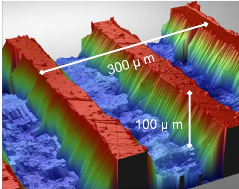
Figure 3.28 - Optical interferometer image of 100 μm depth aluminum cathode
