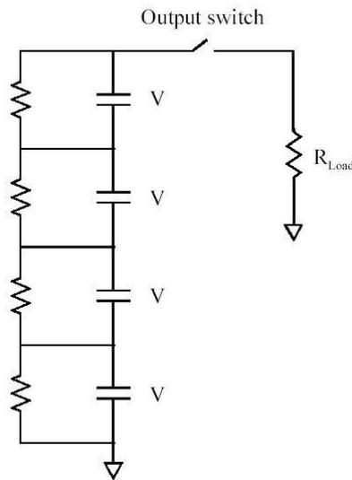
Figure 2.2 – Sample Marx generator discharging circuit [5].
