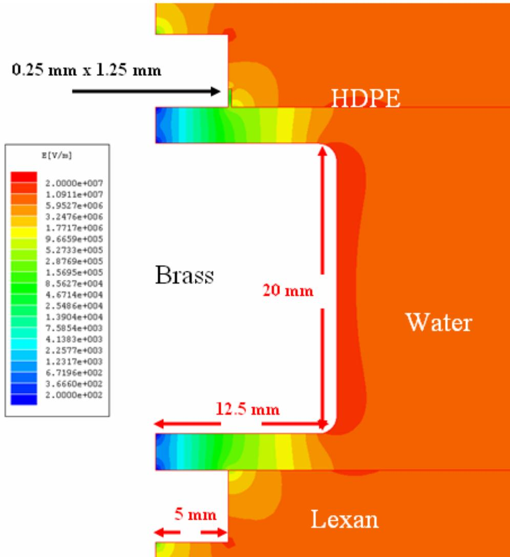
Figure 3.26 – Field simulation final field shaping design of point 3 in protection load section.
