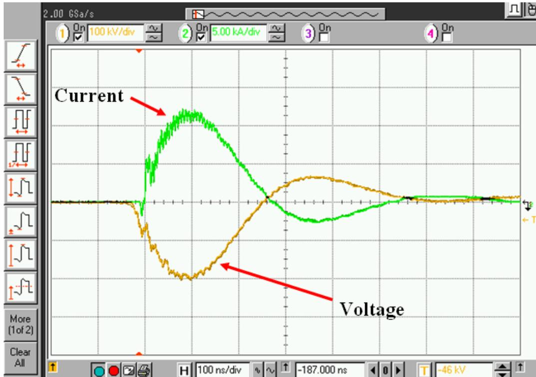
Figure 4.16 - Screen shot of 10 pulses that overlap at 10 Hz operation and 20 kV charging.
