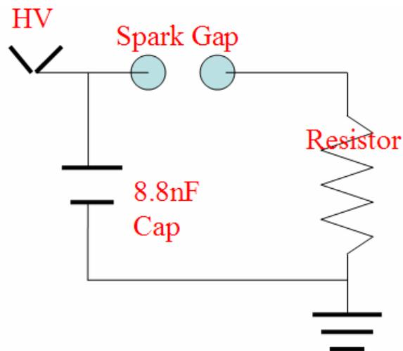
Figure C.1 - Resistor testing setup
