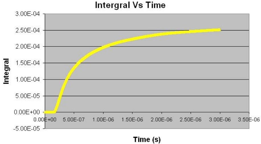
Figure C.4 – Integral of current waveform over time of the Ohmite resistor testing
