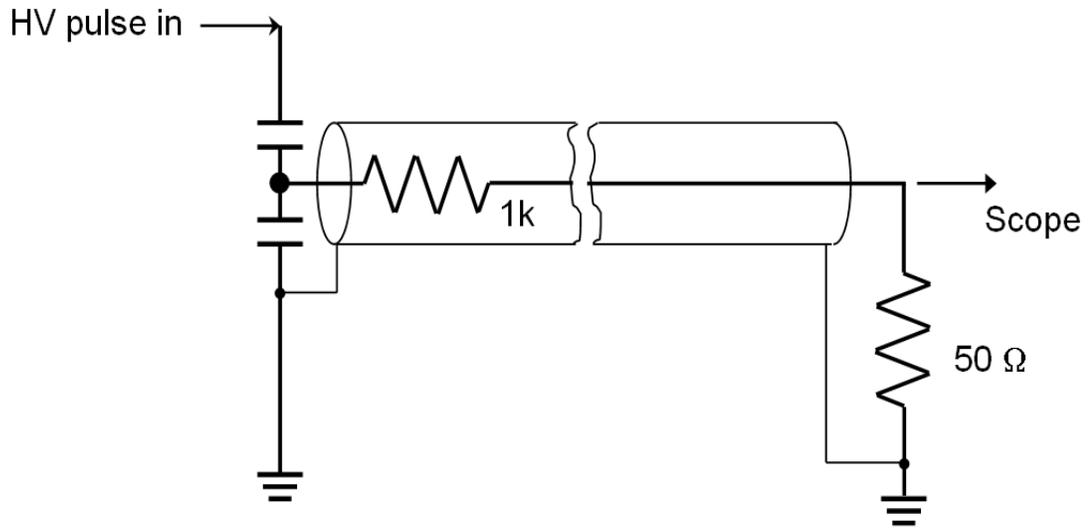
Figure 3.16 – Circuit schematic of capacitive voltage probe.
