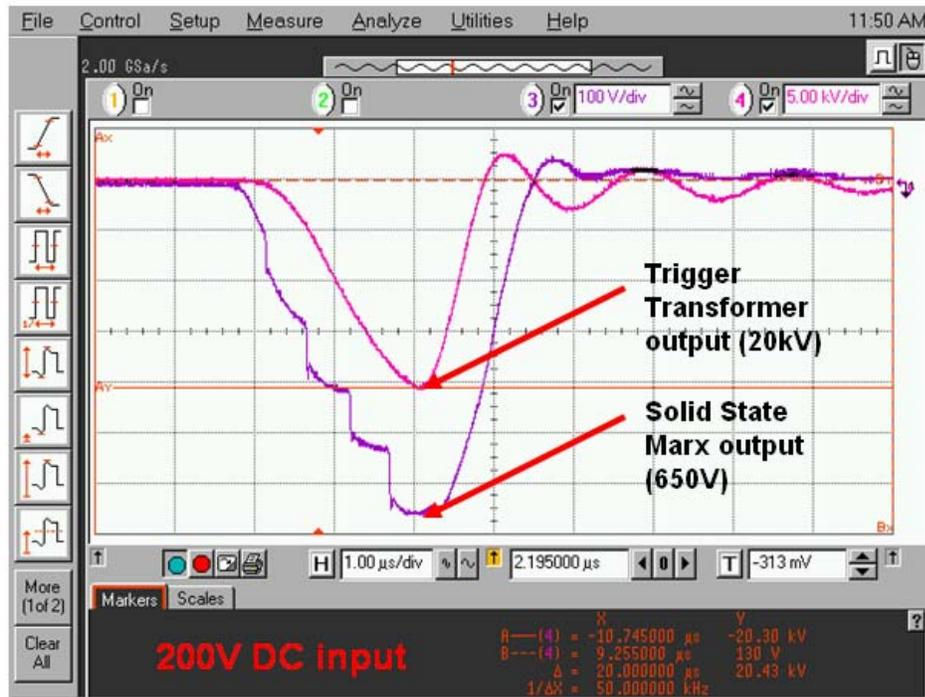
Figure 4.5 – Output of 5 stage thyristor solid state Marx and the trigger wave form after the inductor
