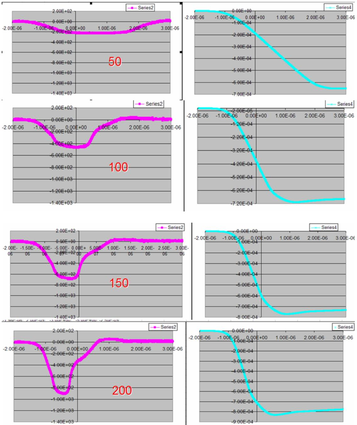
Figure C.6 – Inductor core (ETD 44-3F3, 12.5 mm diameter) testing with 10 turns on the primary, using 50, 100, 150, and 200V charging (Left column: Transformer output voltage. Right column: Volt-seconds)
