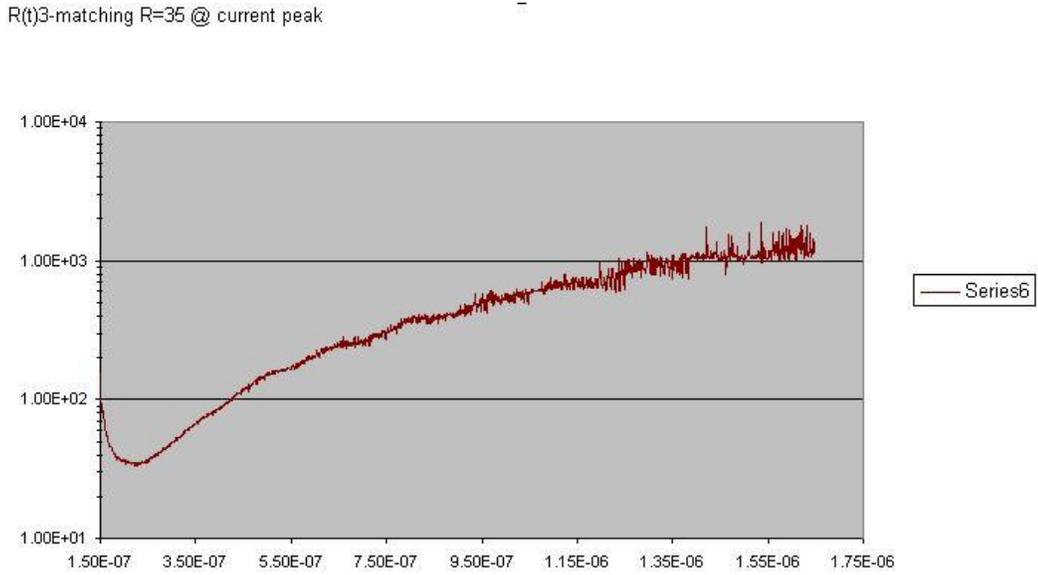
Figure C.5 – Resistance under pulse excitation as a function of time for a  $150\Omega$  nominal resistance.
