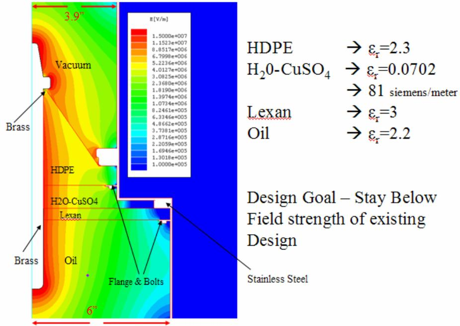
Figure D.3 - Base design of added stages
