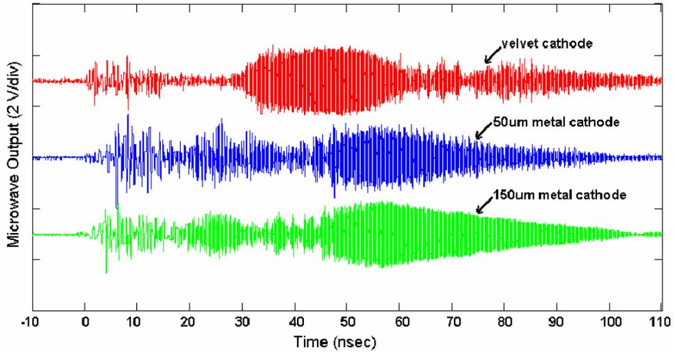
Figure 4.31 - Comparison of microwave signals of the velvet, 100  $\mu\text{m}$ , and 150  $\mu\text{m}$  aluminum cathodes at 6mm A-K gap [11].
