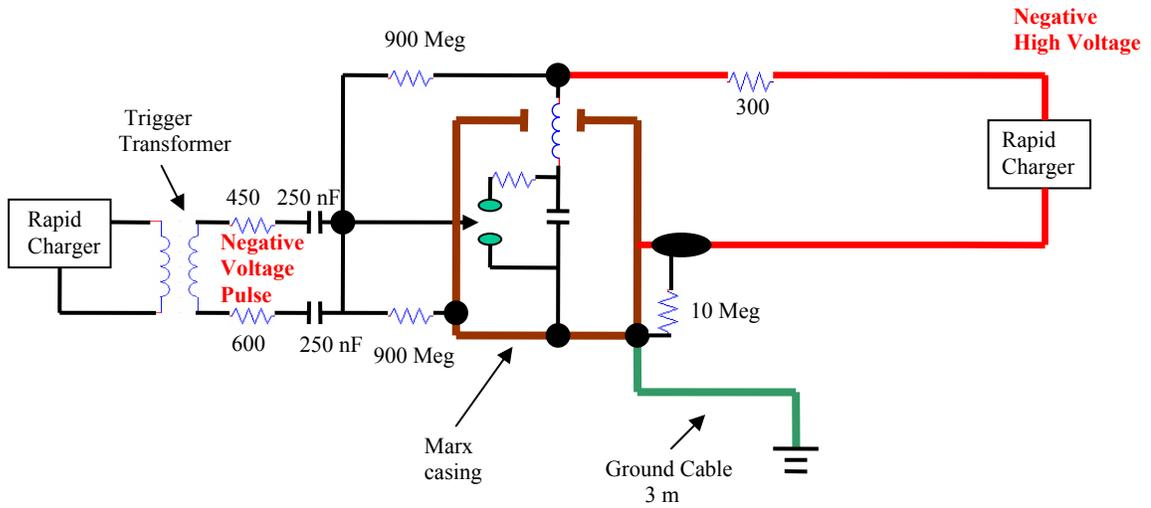
Figure 3.34 - Water load testing with Rapid Charger showing electrical connections and lines
