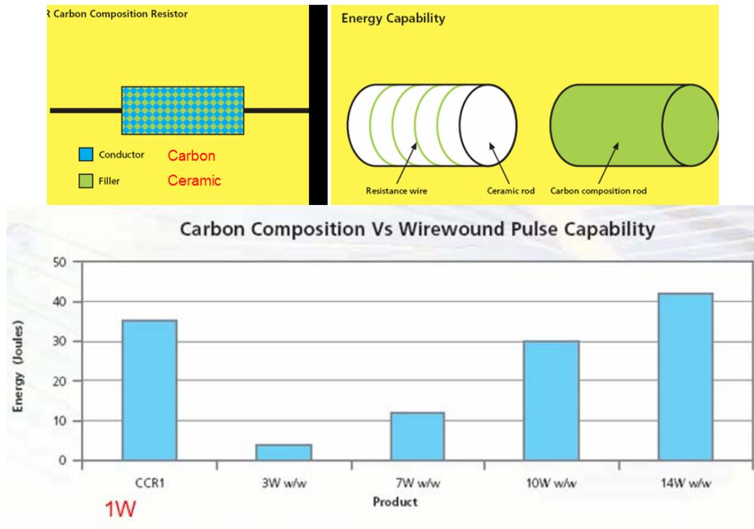
Figure B.1 – Ceramic Composite Resistors structure and energy comparison (<http://www.ttelectronics.com>)
