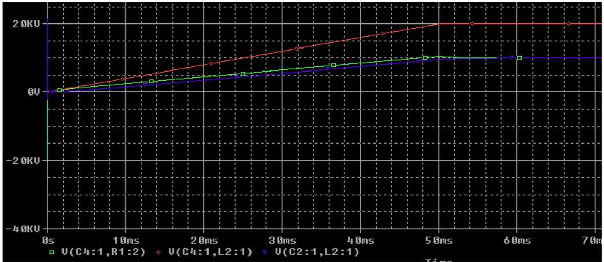
Figure 4.8 - Spark-gap design charging simulation
