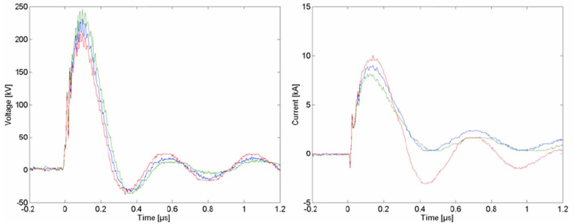
Figure 4.20 - Voltage and current of HPM system at 21 kV charging using a Vircator load with 9mm (green), 10mm (blue), and 11mm (red) AK-gap.
