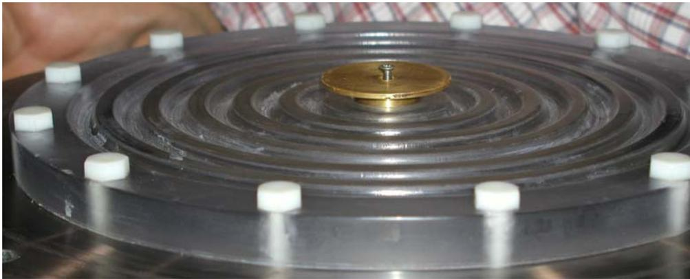
Figure 3.19 - High voltage feed-through connection from CMG spring connectors
