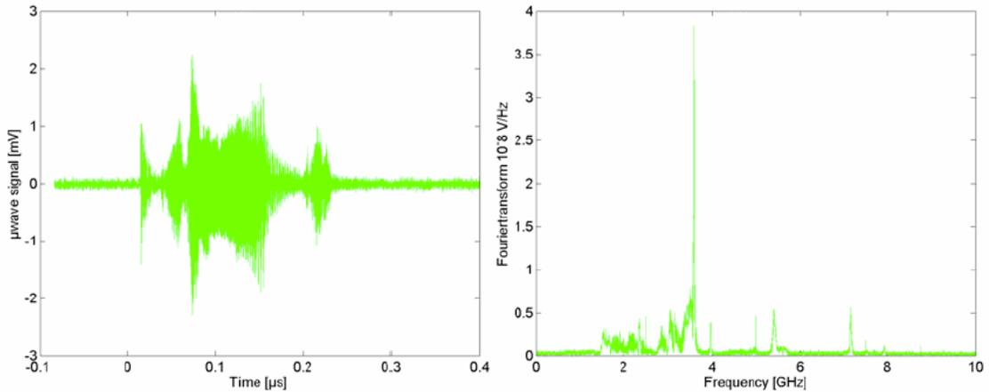
Figure 4.24 - Microwave signal and FFT of HPM system at 21 kV charging with 11 mm A-K gap.
