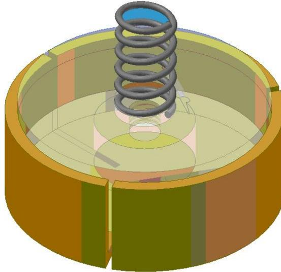
Figure 3.8 - Charging Inductor, showing spring, Lexan, bobbin, and brass encasing
