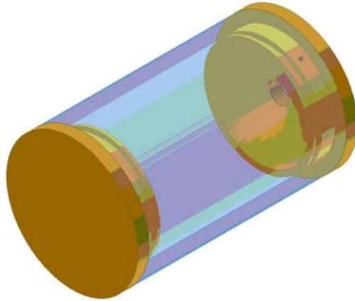
Figure 3.32 - 18.5 Ohm water load
