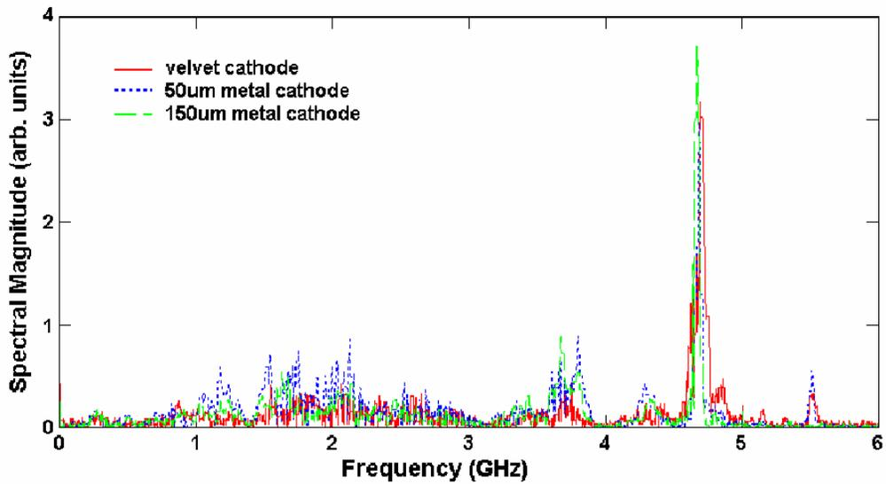
Figure 4.32 - Frequency spectrum of the velvet, 100  $\mu\text{m}$ , and 150  $\mu\text{m}$  aluminum cathodes at 6mm A-K gap [11].
