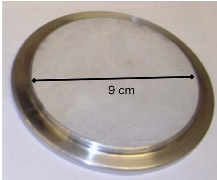
Figure 3.30 - 100 um depth, chemically etched aluminum cathode
