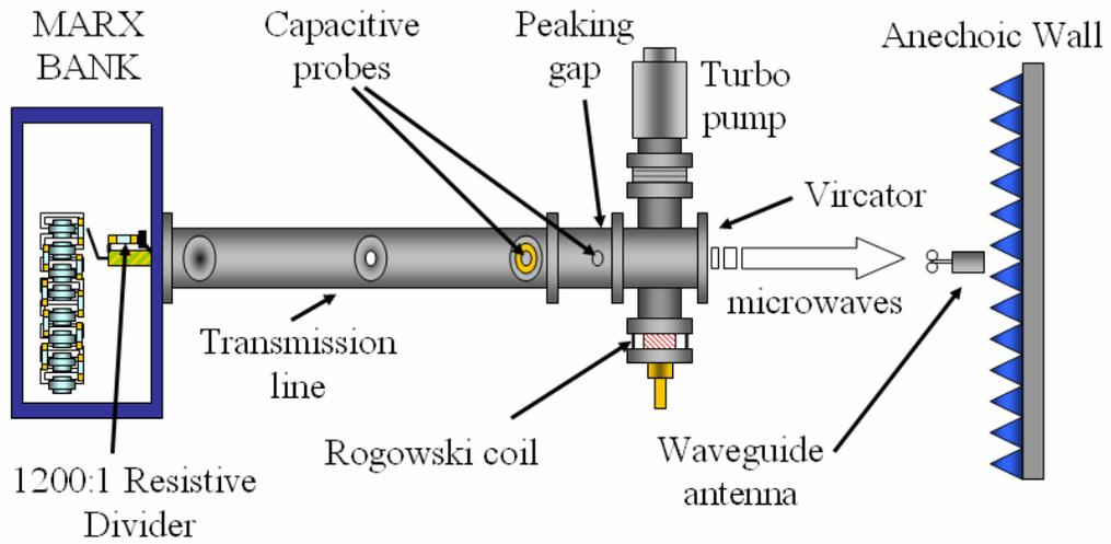
Figure 3.38 - Aluminum cathode single shot testing setup
