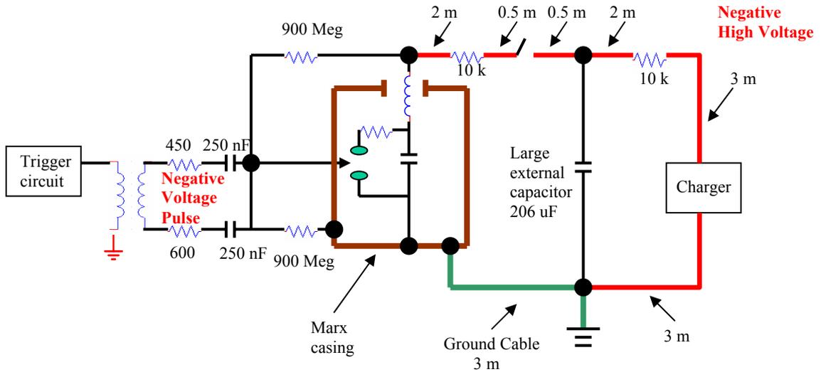
Figure 3.5 - Optional charging setup with large external capacitor
