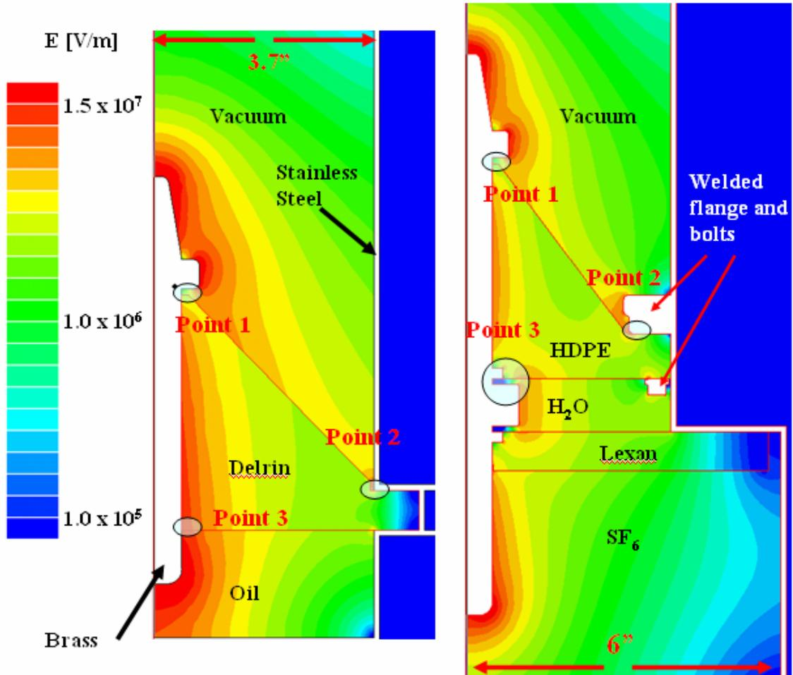
Figure 3.25 – Simulation comparison between the old and new feed-through design with significant triple points labeled
