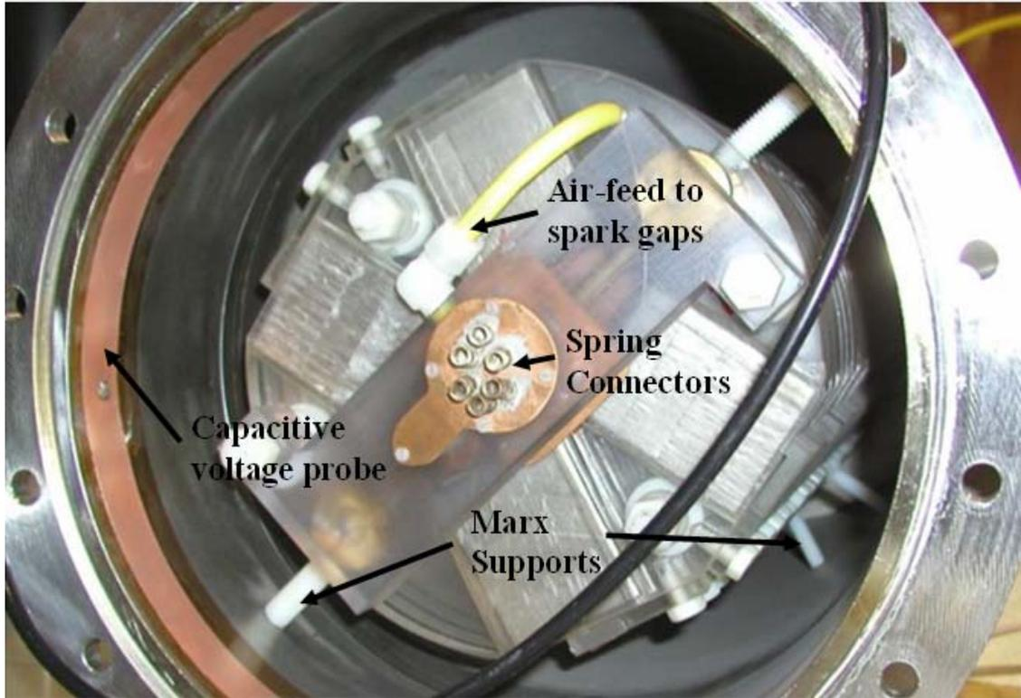
Figure 3.13 - Top stage of Marx, spring connection to HV feed-through, and 200,000:1 capacitive voltage probe.
