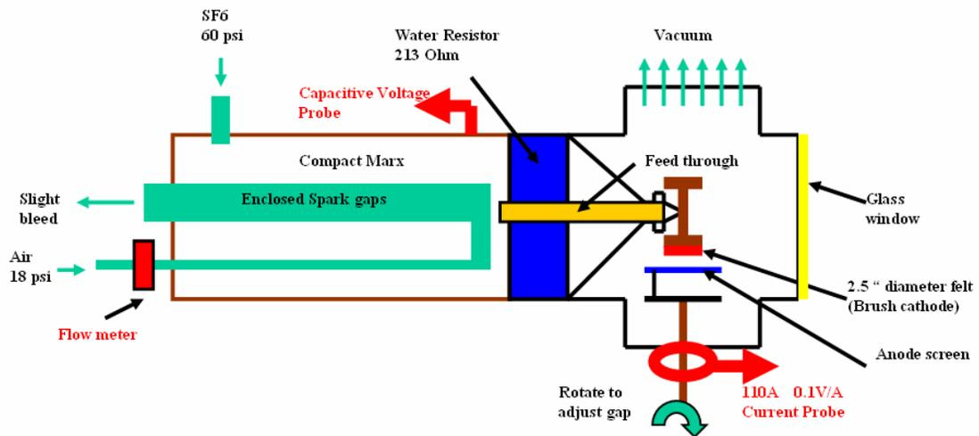
Figure 3.36 - Cross section of Vircator testing
