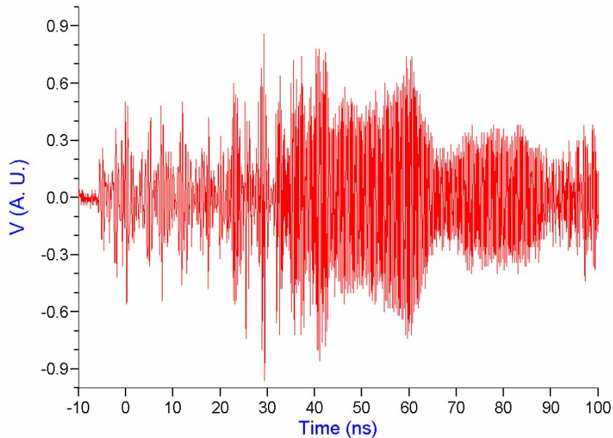
Figure 4.28 – Microwave signal of Velvet cathode using single shot setup at 6 mm A-K gap
