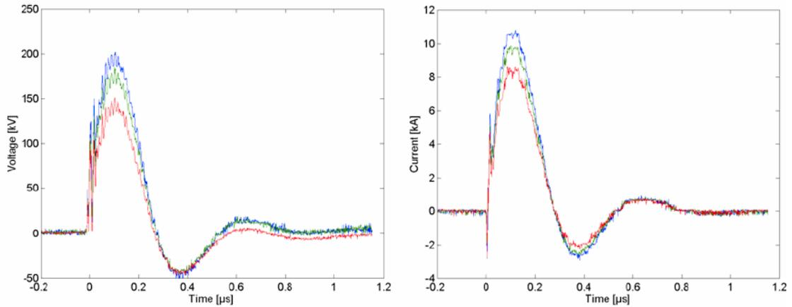
Figure 4.14 - Voltage and current of HPM system into an 18.5 Ohm water load with 15 (red), 17.5 (green), and 20 kV (blue) charging.
