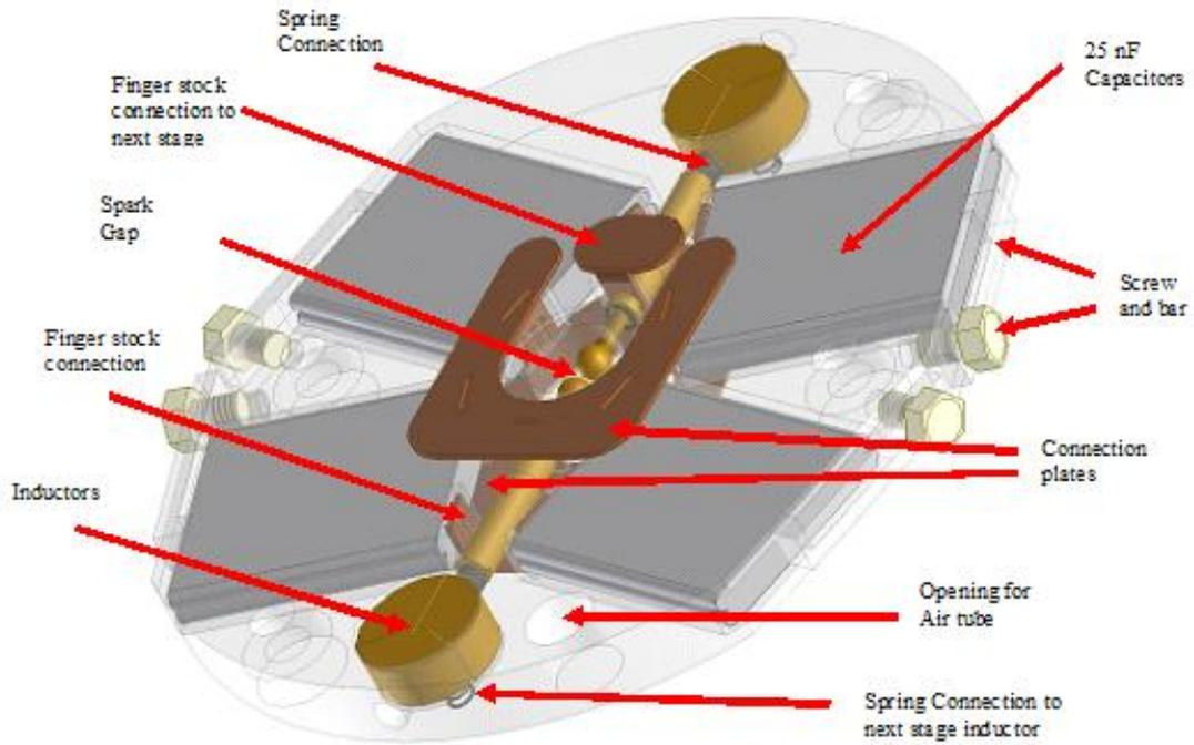
Figure 3.9 - Single stage assembly of the Compact Marx
