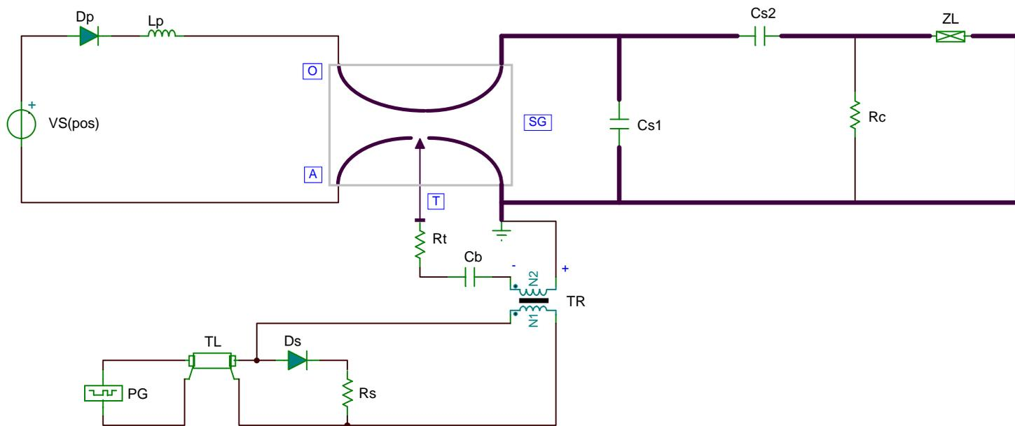
FIGURE 4. LC-inversion circuits.
