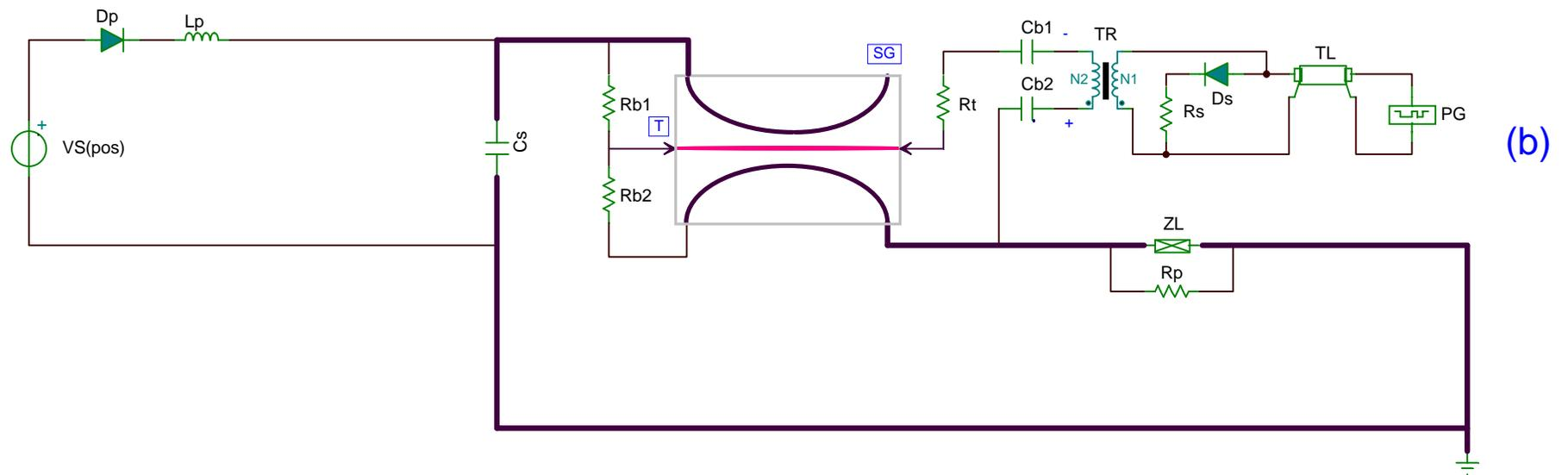
FIGURE 5. Typical series circuits using field-distortion switches.
