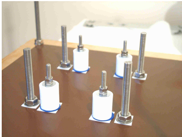
11. On the other side, vacuum facing, the studs come through (without a countersink) with a tapped tefflon standoff tightened down onto compliant washers of silicone and a tefflon piece in contact with the tufnol with the aim of suppressing tracking. (The M8 studs are mechanical supports in blind, threaded, holes. They may end up at a few kV differential to the feedthroughs.)
