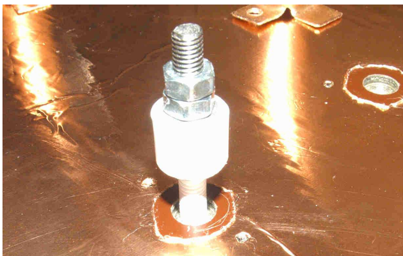
3. M5 A4 stainless stud threaded through with a light wrap of teflon tape and a tapered teflon stand-off.
