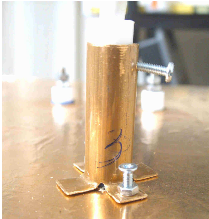
9. Copper pipe petaled out and used as a screening support. Side bolt retains against the strain reliever.
