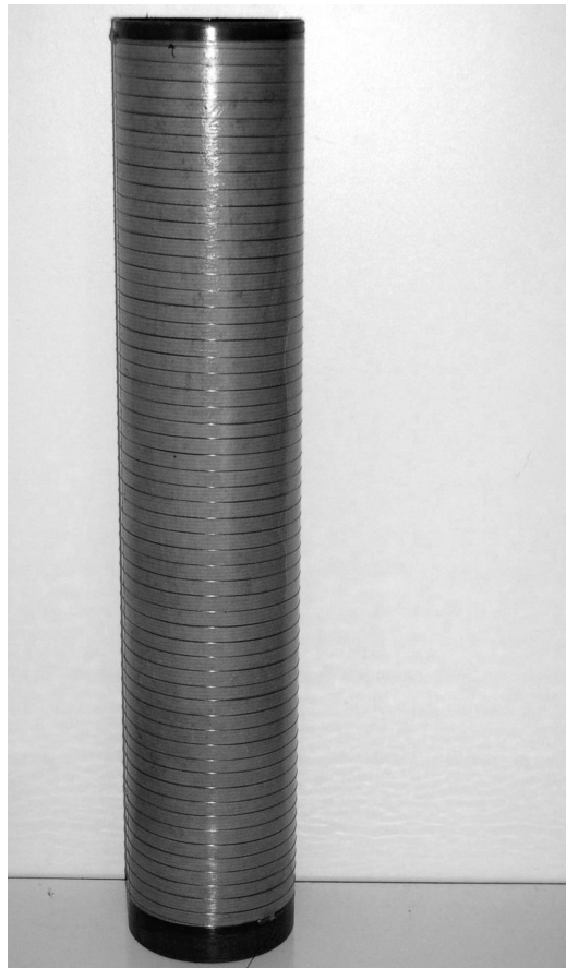
Figure 4.12: Photograph of 56.3 turn constructed model coil
