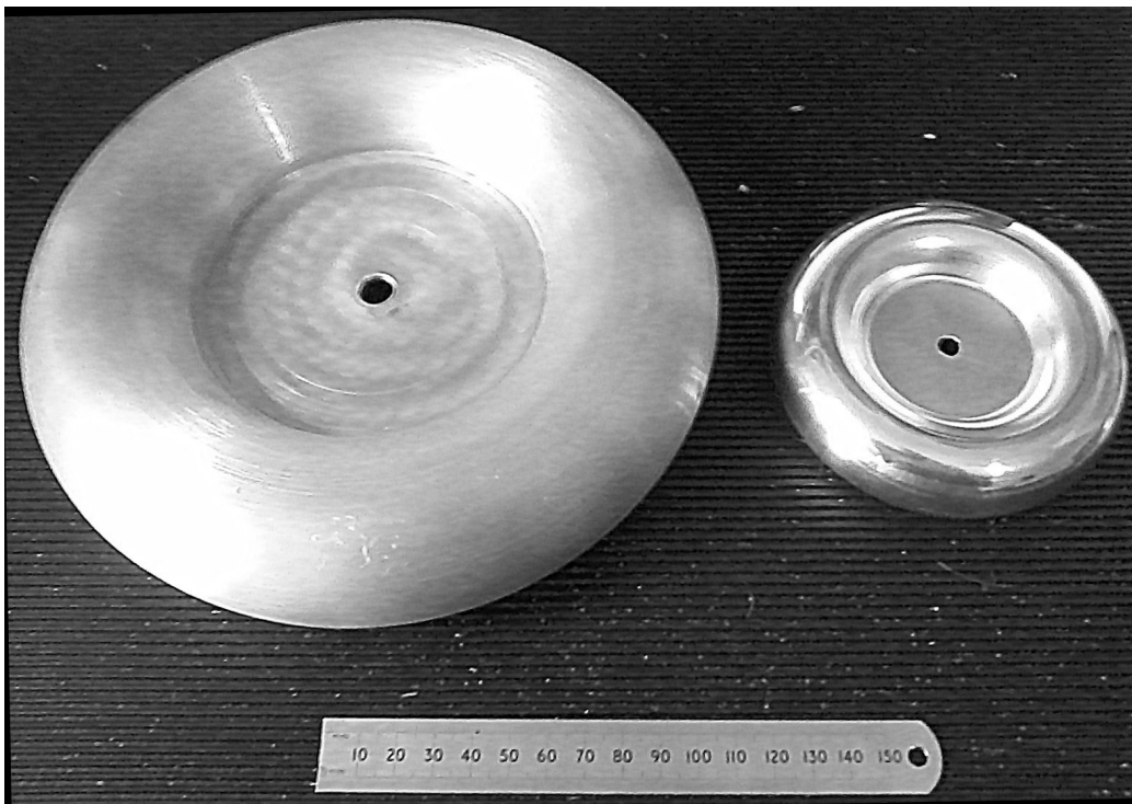
Figure 5.1: Two field grading toroids of different capacitances
