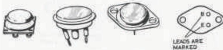
Fig. 11.16 Power transistors.
