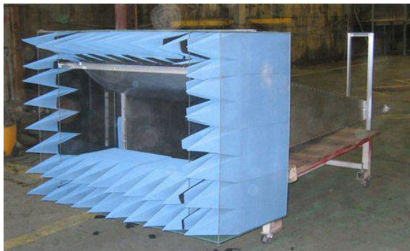
Fig. 5. TEM-horn: 5 GW, 100 MHz to 5 GHz.
