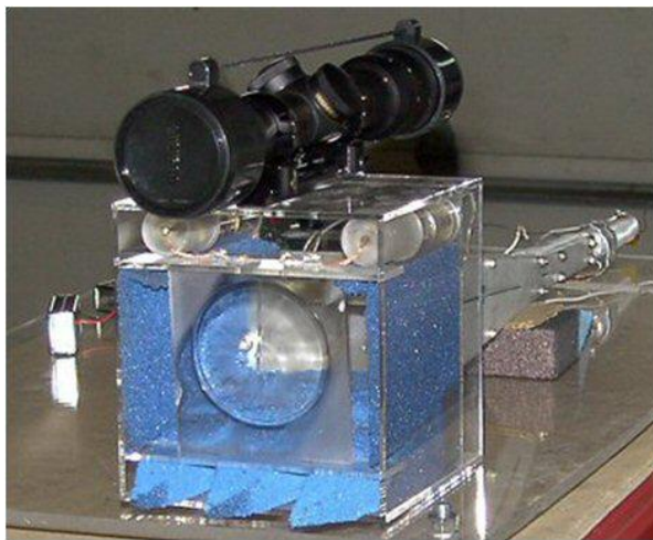
Fig. 6. TEM-horn: 1 GW, 5 to 50 GHz and externally triggered Marx generator powered from small 9 V battery.
