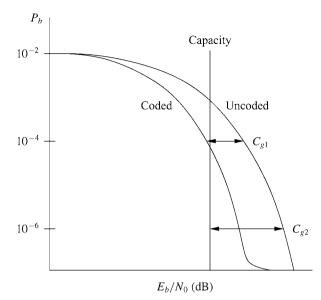
Figure 8.1: Coding gain in AWGN channels.
