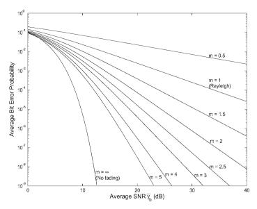
Figure 6.3: Average P<sub>b</sub> for BPSK in Nakagami fading.
