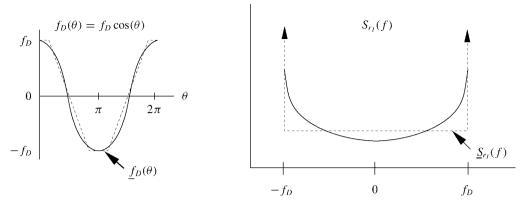
Figure 3.7: Cosine and PSD approximation by straight line segments.
