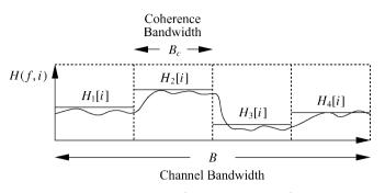
Figure 4.12: Channel division in frequency-selective fading.
