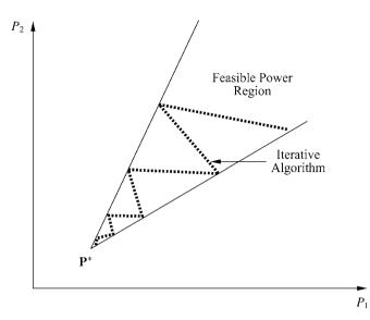
Figure 14.8: Iterative Foschini-Miljanic algorithm.
