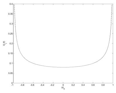
**Figure 3.6:** In-phase and quadrature PSD:  $S_{r_l}(f) = S_{r_Q}(f)$ .
