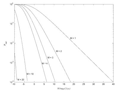
Figure 7.5: Pout for maximal-ratio combining with i.i.d. Rayleigh fading.
