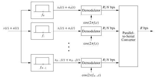
Figure 12.2: Multicarrier receiver.
