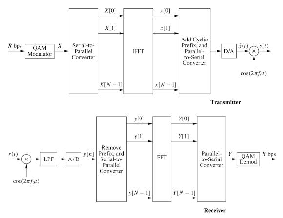
Figure 12.7: OFDM with IFFT/FFT implementation.
