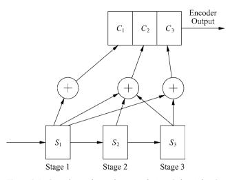
**Figure 8.6:** Convolutional encoder example (n = 3, k = 1, k = 3).
