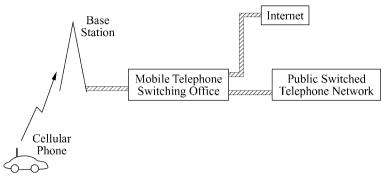
Figure 1.2: Current cellular network architecture.
