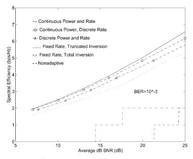
Figure 9.7: Efficiency in log-normal shadowing ( $\sigma_{\psi_{dB}} = 8 \text{ dB}$ ).
