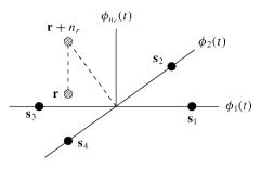
Figure 5.5: Projection of received signal onto received vector **r**.
