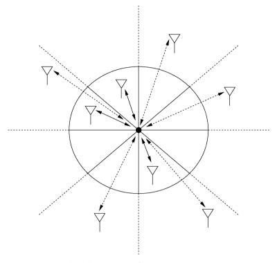
Figure 15.8: Circular cell sectorization for N = 8.
