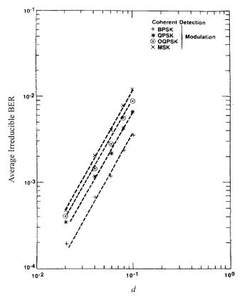
**Figure 6.5:** Irreducible error versus normalized rms delay spread for Gaussian power delay profile. (Reprinted by permission from [25, Fig. 9], © 1987 IEEE.)
