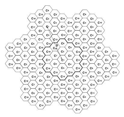
Figure 15.7: Cell clusters for hexagonal cells.
