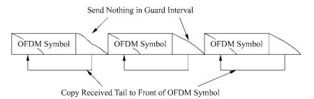
Figure 12.8: Creating a circular channel with an all-zero prefix.
