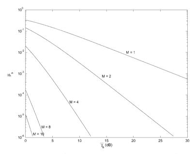
Figure 7.6: Average P<sub>b</sub> for maximal-ratio combining with i.i.d. Rayleigh fading.
