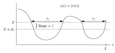
Figure 3.10: Level crossing rate and fade duration for fading process.
