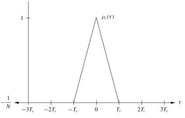
**Figure 13.7:** Autocorrelation of maximal linear code  $(N = T/T_c)$ .
