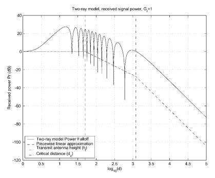
Figure 2.5: Received power versus distance for two-ray model.
