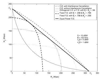
Figure 14.10: Two-user capacity region with 3-dB SNR difference.
