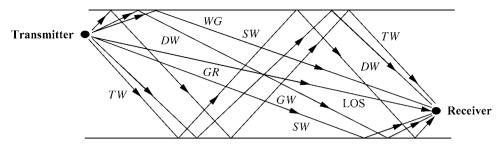
Figure 2.6: Overhead view of the ten-ray model.
