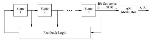
Figure 13.6: Generation of spreading codes.
