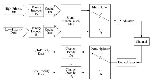
Figure 8.23: Joint optimization of signal constellation.
