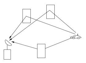
Figure 3.16: Point scatterer channel model.
