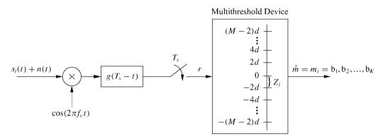
Figure 5.14: Coherent demodulator for MPAM.
