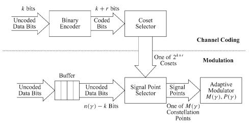
Figure 9.13: Adaptive coded modulation scheme.
