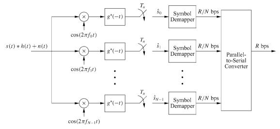
Figure 12.4: Multicarrier receiver for overlapping subcarriers.
