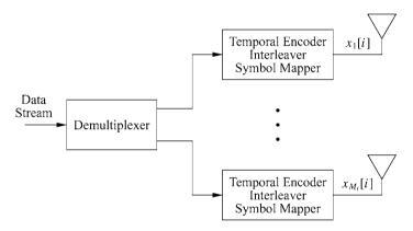
Figure 10.10: Spatial multiplexing with parallel encoding: V-BLAST.
