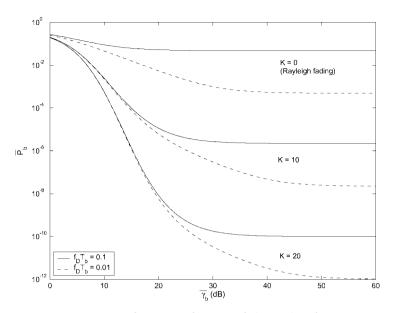
Figure 6.4: Average P<sub>b</sub> for DPSK in fast Rician fading with uniform scattering.
