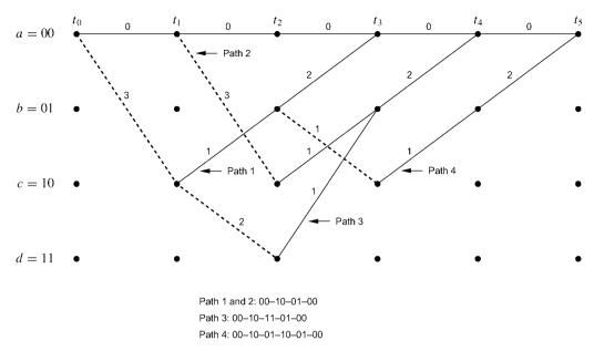
Figure 8.10: Path distances to the all-zero path.
