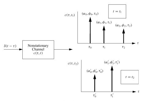
Figure 3.3: Response of nonstationary channel.
