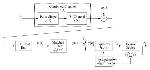
Figure 11.3: End-to-end system (equivalent lowpass representation).
