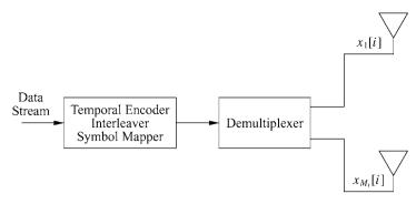
Figure 10.9: Spatial multiplexing with serial encoding.
