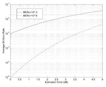
Figure 9.11: Effect of estimation error on BER.
