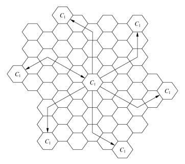
Figure 15.6: Channel assignment in hexagonal cells.
