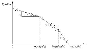
Figure 2.9: Piecewise linear model for path loss.
