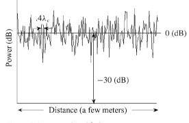
Figure 3.9: Narrowband fading.
