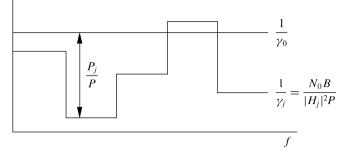
Figure 4.11: Water-filling in frequency-selective block fading.
