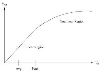
Figure 12.11: Typical power amplifier response.
