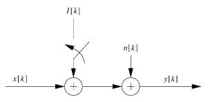
Figure 4.13: Interference channel for Problem 4-8.
