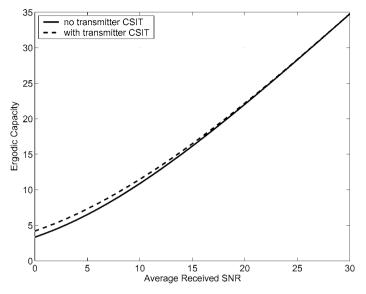
Figure 10.4: Ergodic capacity of  $4 \times 4$  MIMO channel.
