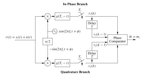
Figure 5.20: Differential PSK demodulator.
