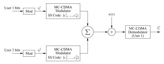
Figure 13.18: Two-user multicarrier CDMA system.
