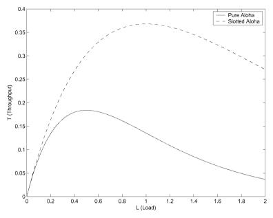
Figure 14.6: Throughput of pure and slotted ALOHA.
