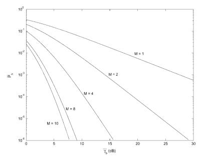
Figure 7.3: Average P<sub>b</sub> of BPSK under selection combining with i.i.d. Rayleigh fading.
