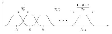
Figure 12.3: Multicarrier with overlapping subcarriers.
