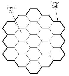
Figure 15.2: Capacity increase by shrinking cell size.
