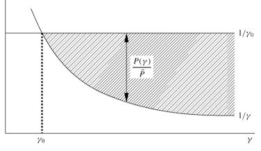
Figure 4.5: Optimal power allocation: water-filling.
