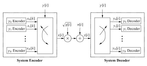
Figure 4.4: Multiplexed coding and decoding.
