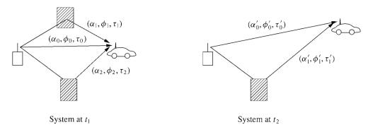
Figure 3.2: System multipath at two different measurement times.
