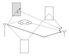
Figure 2.3: Reflected, diffracted, and scattered wave components.
