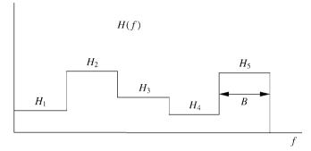
Figure 4.10: Block frequency-selective fading.
