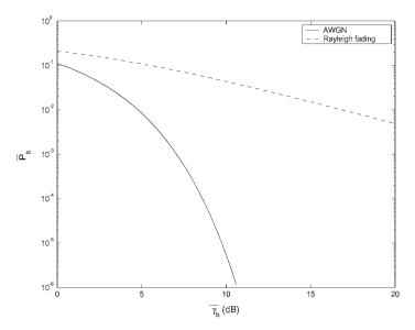
Figure 6.1: Average P<sub>b</sub> for BPSK in Rayleigh fading and AWGN.
