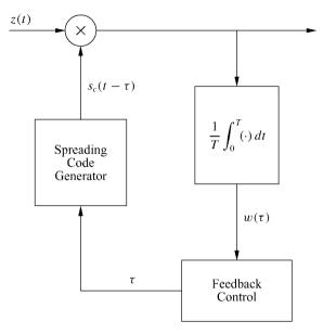
Figure 13.9: Synchronization loop for DSSS.
