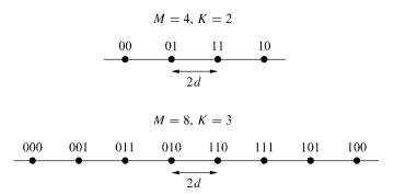
Figure 5.12: Gray encoding for MPAM.
