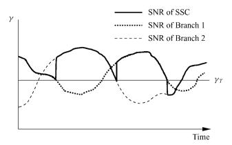
Figure 7.4: SNR of the SSC technique.
