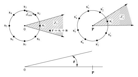
Figure 5.8: Error probability integral and its rotational/shift invariance.
