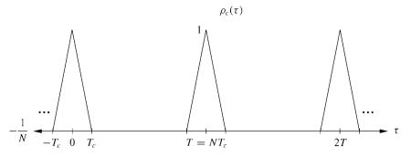
**Figure 13.8:** Autocorrelation has period  $T = NT_c$ .
