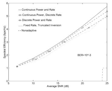
Figure 9.8: Efficiency in Rayleigh fading.
