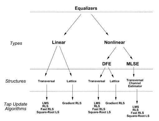
Figure 11.2: Equalizer types, structures, and algorithms.
