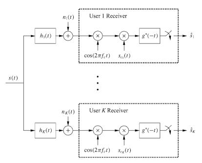
Figure 13.14: Downlink channel and receiver.
