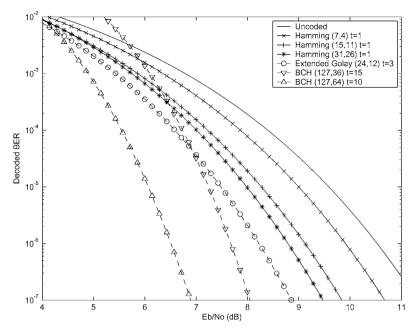
Figure 8.4: Pb for different BCH codes.
