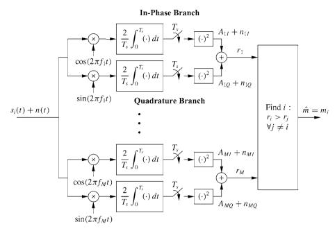
Figure 5.25: Noncoherent FSK demodulator.
