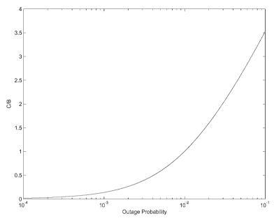
Figure 4.2: Normalized capacity (C/B) versus outage probability.
