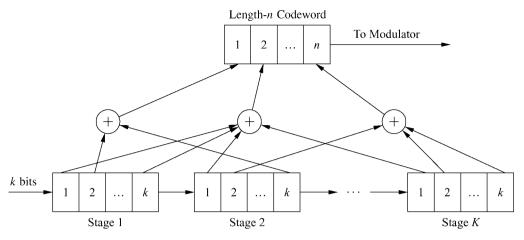
Figure 8.5: Convolutional encoder.
