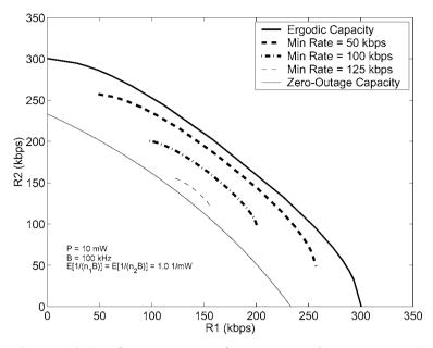
**Figure 14.12:** Ergodic, zero-outage, and minimum rate BC capacity regions (Rician fading with a K-factor of 1, average SNR = 10 dB).
