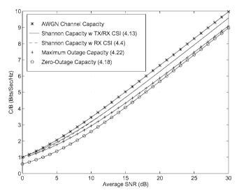
**Figure 4.8:** Capacity in Nakagami fading (m = 2).
