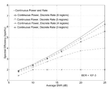
**Figure 9.5:** Discrete-rate efficiency in log-normal shadowing ( $\sigma_{\psi_{dB}} = 8 \text{ dB}$ ).
