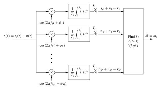
Figure 5.23: Frequency demodulator (coherent).
