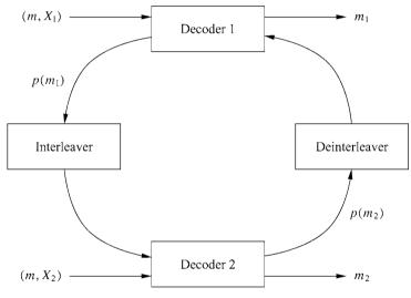
Figure 8.15: Turbo decoder.
