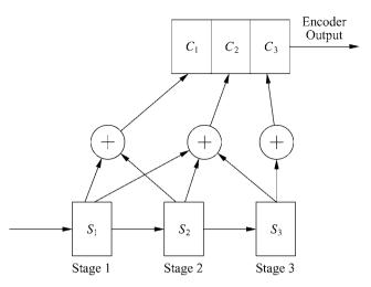
Figure 8.24: Convolutional encoder for Problems 8-14 and 8-15.
