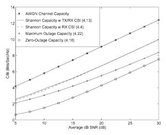
Figure 4.6: Capacity in log-normal fading.
