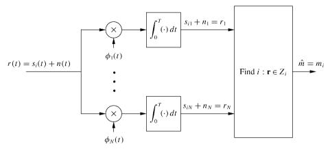
Figure 5.4: Receiver structure for signal detection in AWGN.
