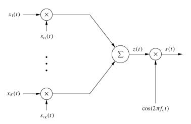
Figure 13.13: Downlink transmitter.
