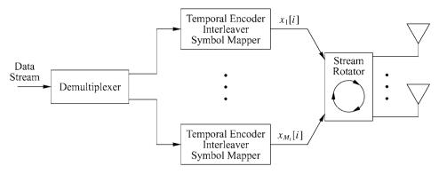
Figure 10.12: Diagonal encoding with stream rotation.
