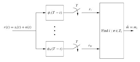
Figure 5.7: Matched filter receiver structure.
