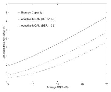
Figure 9.3: Average spectral efficiency in Rayleigh fading.
