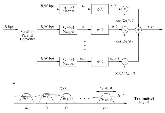
Figure 12.1: Multicarrier transmitter.
