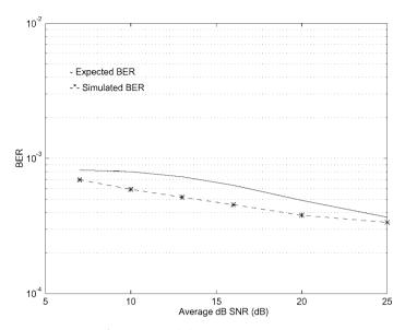
Figure 9.9: BER for log-normal shadowing (six regions).
