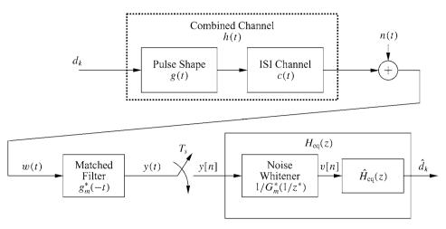
Figure 11.4: MMSE equalizer with noise-whitening filter.
