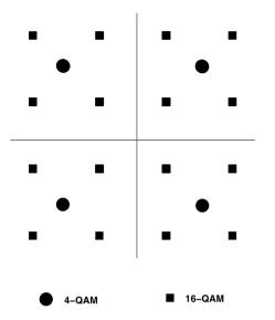
Figure 5.18: 4-QAM and 16-QAM constellations.
