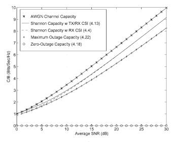
Figure 4.7: Capacity in Rayleigh fading.
