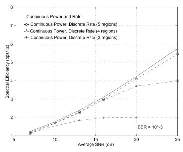
Figure 9.6: Discrete-rate efficiency in Rayleigh fading.
