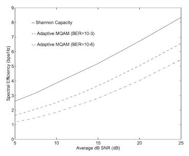
**Figure 9.2:** Average spectral efficiency in log-normal shadowing ( $\sigma_{\psi_{dB}} = 8 \text{ dB}$ ).
