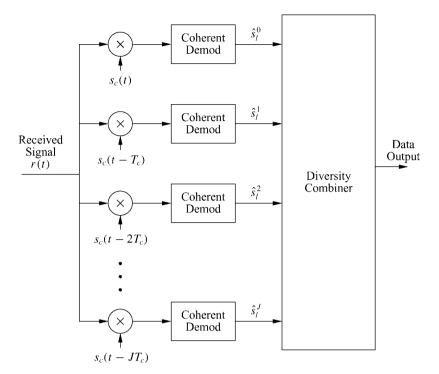
Figure 13.10: RAKE receiver.
