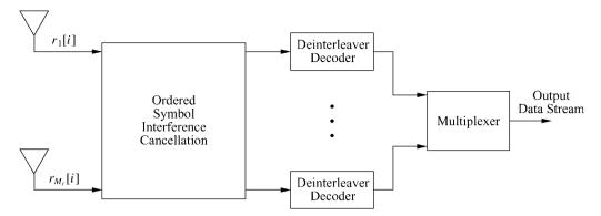
Figure 10.11: V-BLAST receiver with linear complexity.
