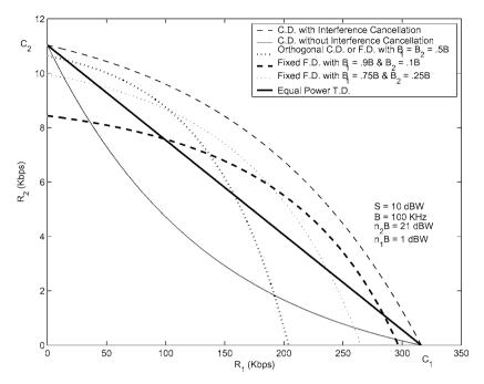
Figure 14.11: Two-user capacity region with 20-dB SNR difference.
