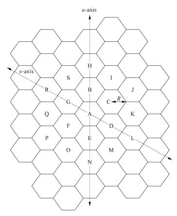
Figure 15.4: Axes for reuse distance in hexagonal cells.
