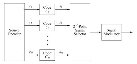
Figure 8.21: Multilevel encoder.
