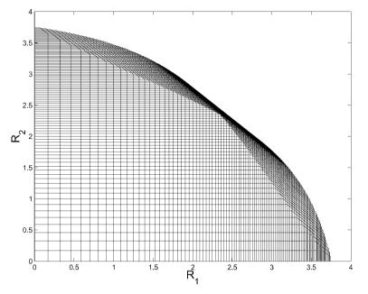
Figure 14.13: MIMO BC capacity region with  $H_1 = [1 \ 0.5]$ ,  $H_2 = [0.5 \ 1]$ , and P = 10.
