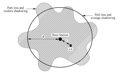
Figure 2.10: Contours of constant received power.
