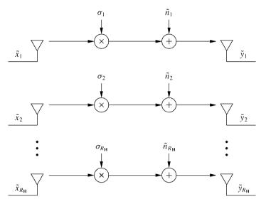
Figure 10.3: Parallel decomposition of the MIMO channel.
