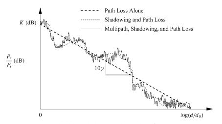
Figure 3.8: Combined path loss, shadowing, and narrowband fading.
