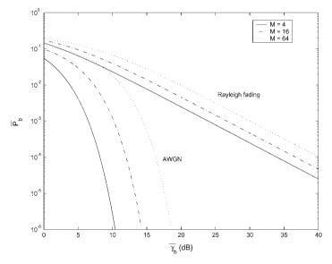
Figure 6.2: Average P<sub>b</sub> for MQAM in Rayleigh fading and AWGN.
