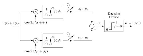
Figure 5.24: Demodulator for binary FSK.
