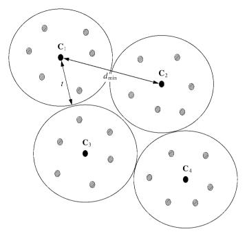
Figure 8.3: Maximum likelihood decoding in code space.
