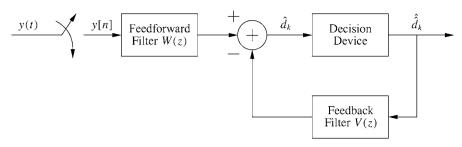
Figure 11.5: Decision-feedback equalizer structure.
