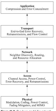
Figure 16.2: Five-layer model for network protocol design.
