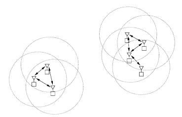
Figure 16.3: Disconnected network.
