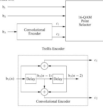
Figure 8.25: 16-QAM trellis encoder for Problem 8-16.
