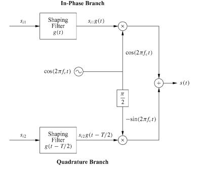
Figure 5.21: Modulator with quadrature offset.
