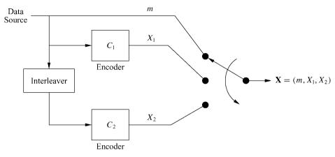
Figure 8.14: Parallel concatenated (turbo) encoder.
