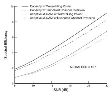
Figure 9.4: Spectral efficiency with different power adaptation policies (Rayleigh fading).
