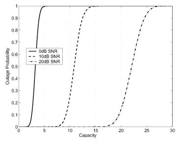
Figure 10.6: Outage probability distribution of a 4 × 4 MIMO channel.
