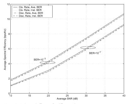
Figure 9.16: Spectral efficiency for different adaptation constraints.
