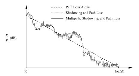
Figure 2.1: Path loss, shadowing, and multipath versus distance.
