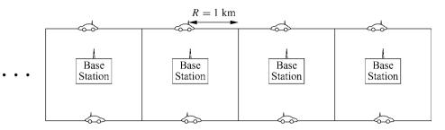
Figure 15.12: One-dimensional cellular system with square cells (Problem 15-11).
