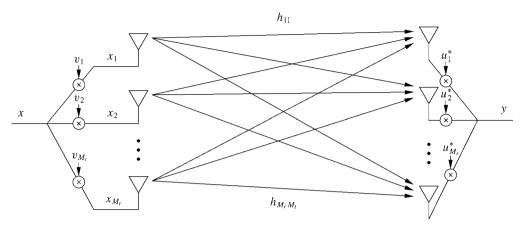
Figure 10.7: MIMO channel with beamforming.
