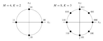
Figure 5.15: Gray encoding for MPSK.
