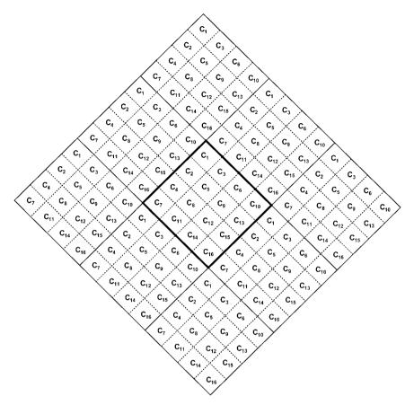
Figure 15.5: Cell clusters for diamond cells.
