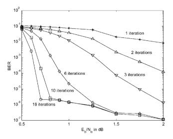
Figure 8.16: Turbo code performance (rate 1/2, K = 5 component codes with interleaver depth 2<sup>16</sup>).
