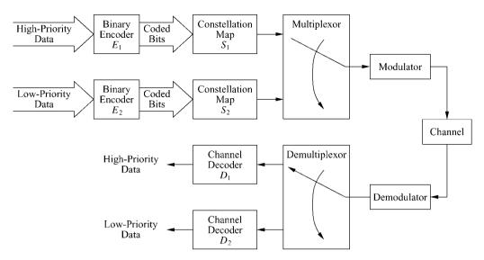
Figure 8.22: Transceiver for time-multiplexed coded modulation.
