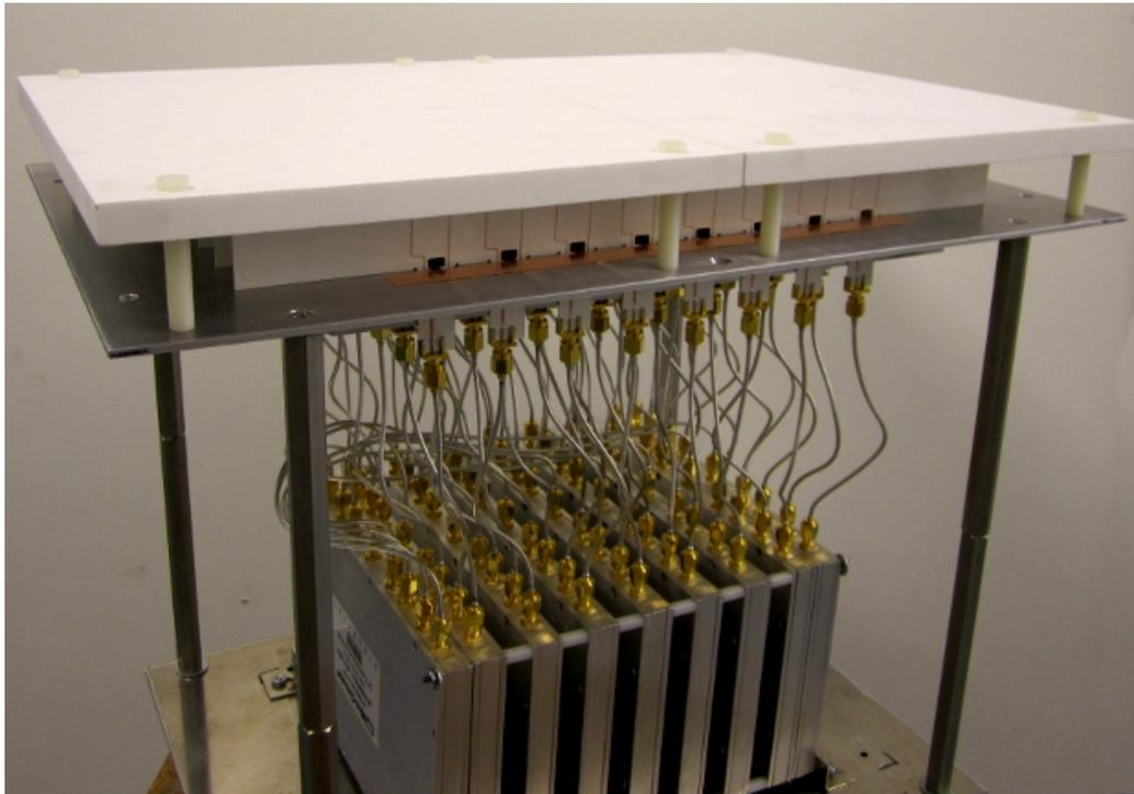
Figure 6.18: Entire TCDA-IB prototype array showing 64:1 power divider network.
