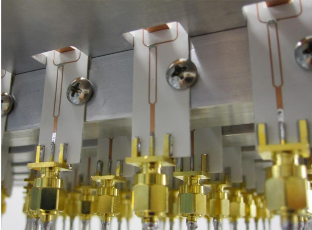
Figure 6.17: Detail of TCDA-IB prototype underside showing element mounting and coaxial connectors.
