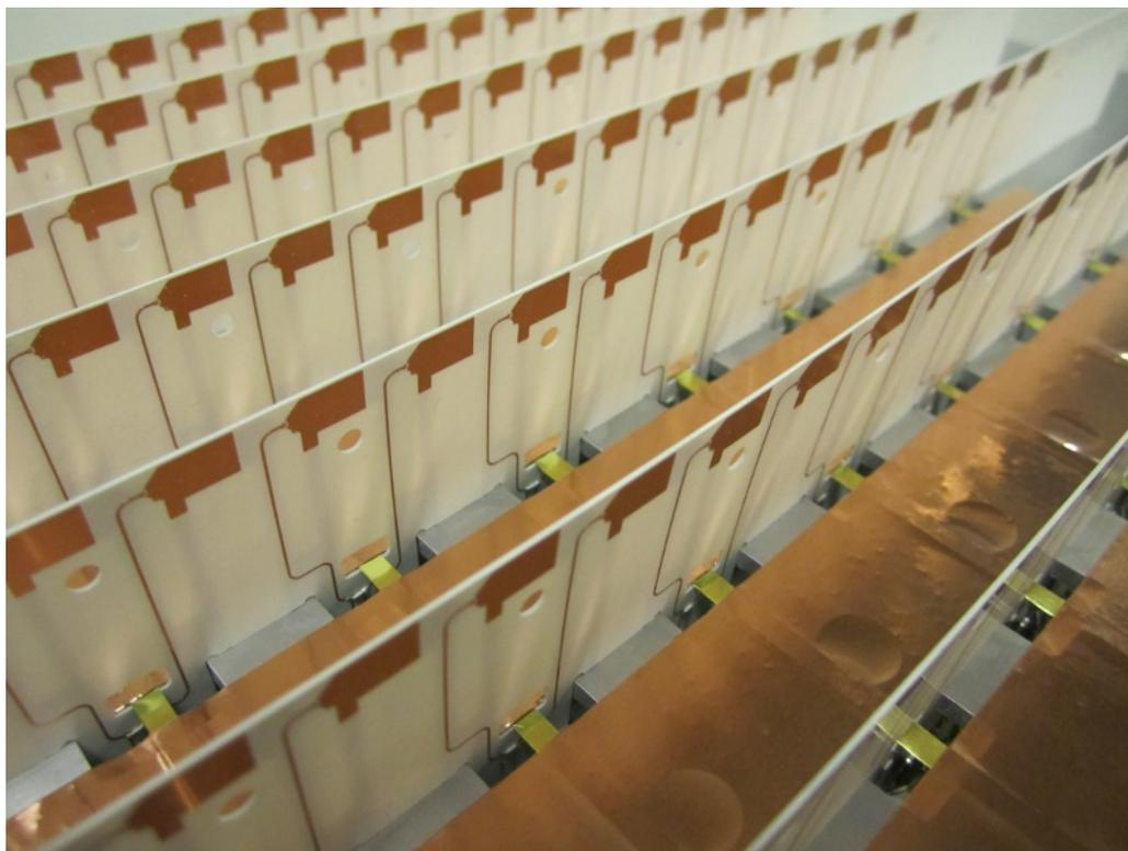
Figure 6.15: Closeup of TCDA-IB prototype aperture showing element details.
