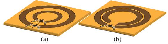
Fig. 4. Unique magnetic properties of the ULM attainable by using multiple rings of resonance frequencies  $\omega_{0n}$ , here two rings with resonance frequencies  $\omega_{01}$  and  $\omega_{02}$ . (a) Multiband operation using independent rings with separate resonance frequencies. (b) Enhanced bandwidth using coupled-resonant rings with overlapping resonance frequencies.
