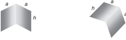
Figure 6.42 Dihedral, left: co-polarization \sigma_{hh} and \sigma_{vv} only; right: cross-polarization only \sigma_{hv} and \sigma_{vh} .
