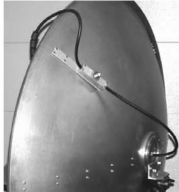
Figure 3. Splitter with feed cables mounted on back side of IRA-6.
