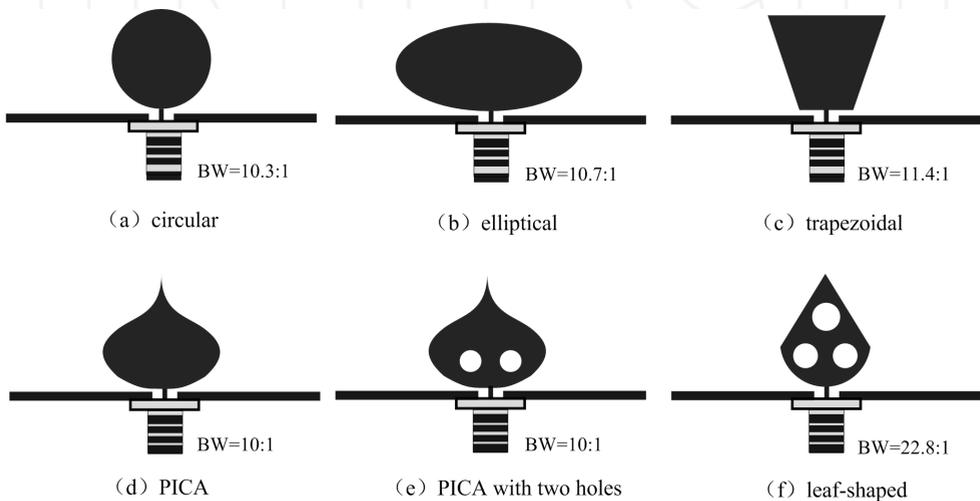
**Figure 9.** Various geometries of planar monopole antennas<sup>[11-14]</sup>.
