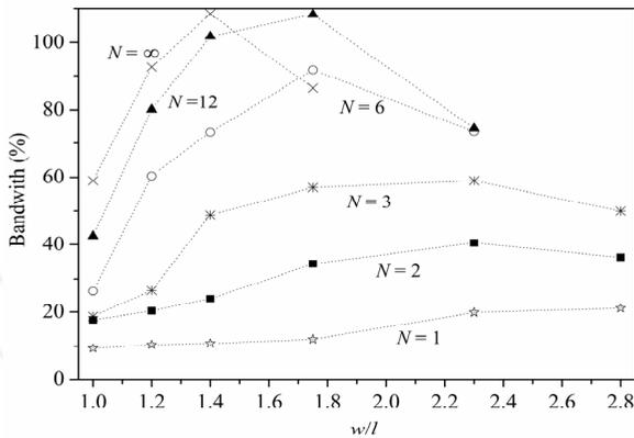
**Figure 21.** Various bandwidths for orders  $N$ .
