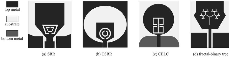
**Figure 27.** Notched-band designs with various periodic structure slots [70-73].
