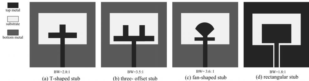
Figure 16. Various shapes of tuning stubs [40-43].
