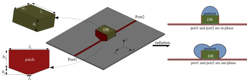
**Figure 25.** UWB DRAs with a radiation reconfiguration.
