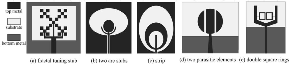
**Figure 28.** Notched-band designs with various stubs [74–78].
