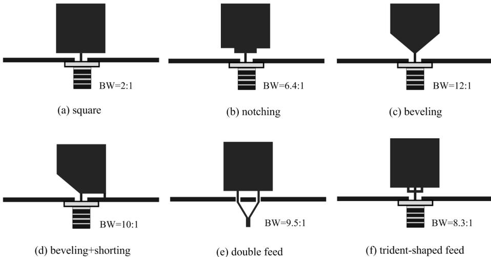
**Figure 10.** Various wideband techniques for planar square monopole antennas<sup>[15-19]</sup>.
