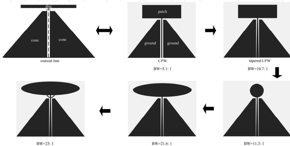
**Figure 13.** Various printed monopole antennas with trapeziform ground [32-36].
