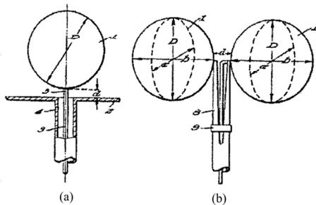
**Figure 8.** Stohr's ellipsoidal monopole and dipole (1968).
