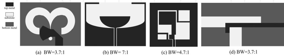
**Figure 18.** Special geometries of wide-slot antennas [49-52].
