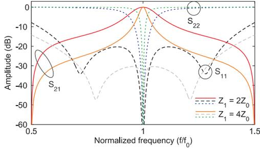
Fig. 2. Theoretical synthesis examples of the reflectionless bandpass filter in Fig. 1(a) in terms of  $S$  parameters: bandwidth control by means of  $Z_1$  ( $Z_2 = Z_{r1} = Z_{r2} = Z_0$  where  $Z_0$  is the reference impedance).
