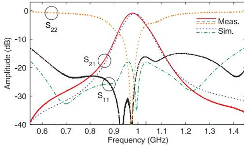
Fig. 5. Simulated and measured power transmission ( $|S_{21}|$ ) and input-reflection ( $|S_{11}|$ ) parameters and measured power output-reflection ( $|S_{22}|$ ) parameter of the manufactured reflectionless tunable microstrip bandpass filter prototype for one example state (estimated quality factor  $Q = 100$  at 1 GHz for all variable capacitors).
