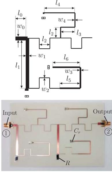
Fig. 4. Layout—half part—and photograph of the manufactured reflectionless tunable microstrip bandpass filter prototype (dimensions in mm:  $w_0 = 3.42$ ,  $w_1 = 2.97$ ,  $w_2 = 0.3$ ,  $w_3 = 1.12$ ,  $w_4 = 0.56$ ,  $l_0 = 10$ ,  $l_1 = 40.4$ ,  $l_2 = 10$ ,  $l_3 = 13.4$ ,  $l_4 = 29.4$ ,  $l_5 = 19.2$ , and  $l_6 = 26.2$ ; components:  $C_r = 1\text{--}5$  pF and  $R = 45.9$   $\Omega$ ).
