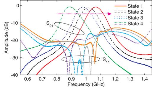
Fig. 6. Measured center-frequency tuning capabilities in terms of power transmission ( $|S_{21}|$ ) and input-reflection ( $|S_{11}|$ ) parameters of the manufactured reflectionless tunable microstrip bandpass filter prototype.
