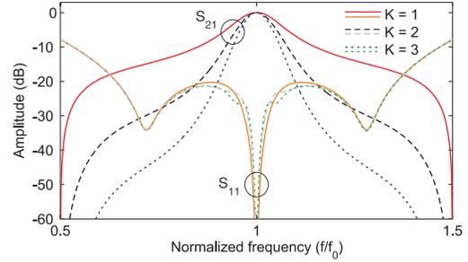
Fig. 3. Theoretical synthesis examples of the reflectionless bandpass filter in Fig. 1(a) and (b) in terms of  $S$  parameters: single- and multi-stage designs ( $Z_1 = 2Z_0, Z_2 = Z_{r1} = Z_{r2} = Z_0$  where  $Z_0$  is the reference impedance).
