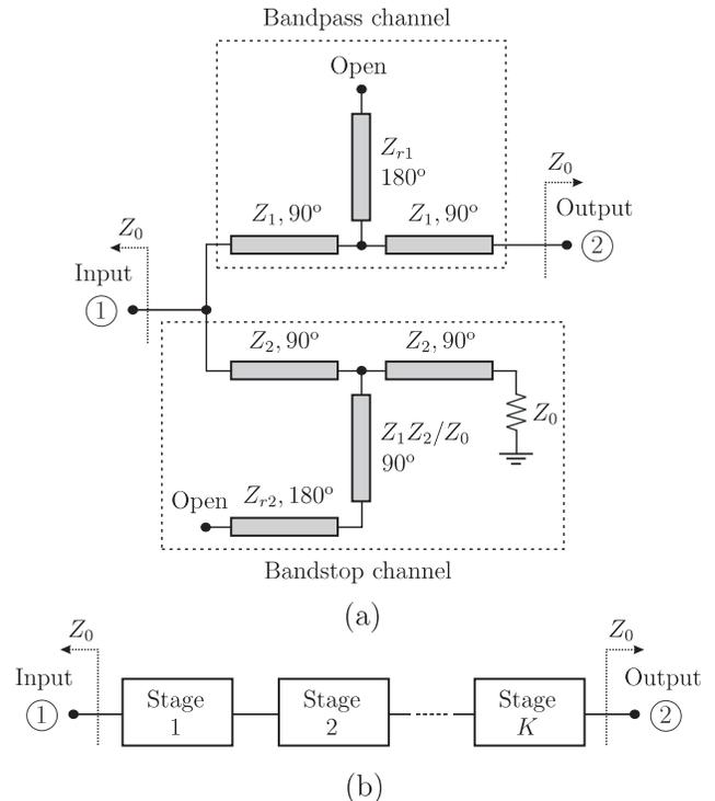
Fig. 1. (a) Circuit detail of the proposed reflectionless bandpass filter based on a complementary-duplexer architecture: first-order case ( $Z_1$ ,  $Z_2$ ,  $Z_{r1}$ , and  $Z_{r2}$  denote characteristic impedances of transmission-line segments— $Z_0$  is the reference impedance—and all their electrical-length values are expressed at the center frequency of the filter). (b) In-series-cascade  $K$ -stage scheme for filter designs with increased stopband attenuation.
