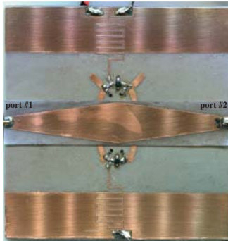
Figure 11. Prototype device with asymmetric stub structure ( a = b = 1 , c = d = 6 mm), corresponding to the structure giving the response of fig.6.
