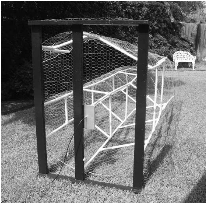
Figure 13 — The complete TASH antenna on its side showing the feed point.
