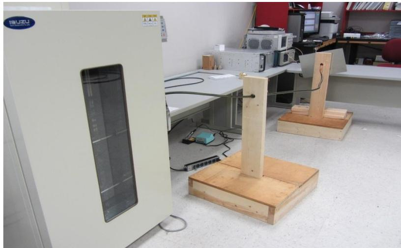
Figure 7.2. Photograph of non-intrusive accelerated aging test.
