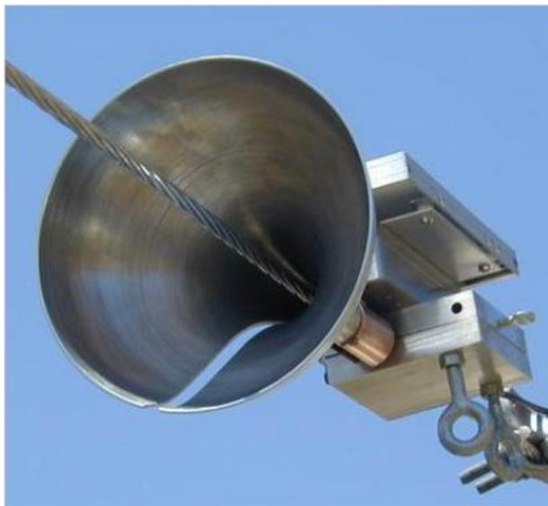
Figure 4.5. Elmore designed slotted horn antenna directly connected with a bare aluminum power line cable reported in [65].
