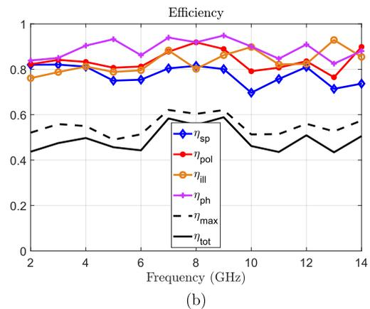
Fig. 26. Feed efficiency of the reflector based on the measured radiation patterns of (a) Dyson element and (b) DYQSA feed.
