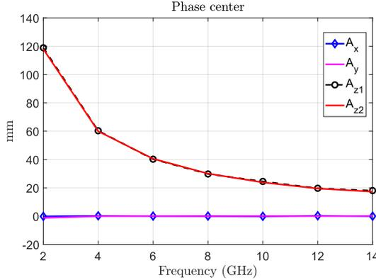
Fig. 9. Phase center estimation of the Dyson element.
