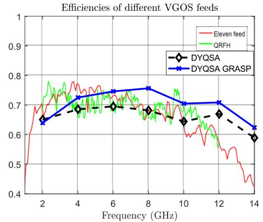
Fig. 22. Comparison of the efficiency of different feeds.
