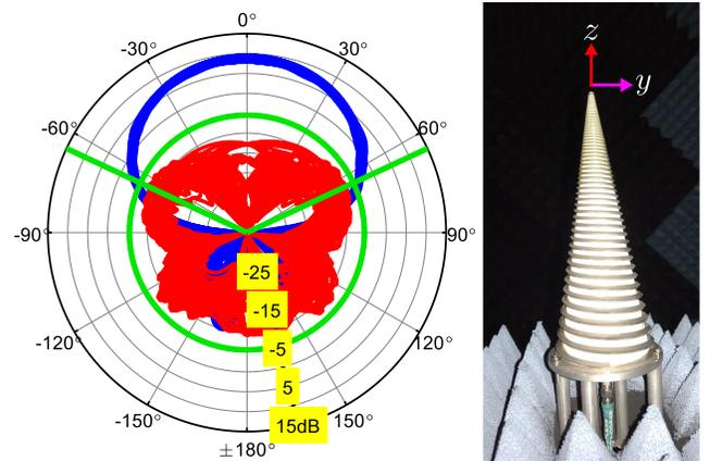
Fig. 7. Radiation patterns of the Dyson element.
