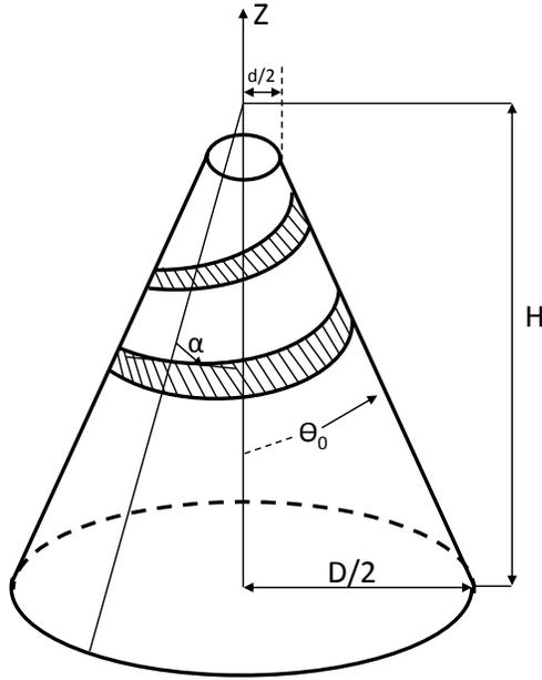
Fig. 5. Geometry of the Dyson conical log-spiral antenna.
