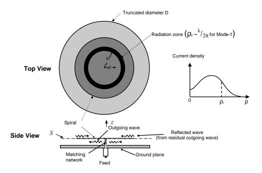
Figure 1. The radiation and radiation zone of a TW antenna.
