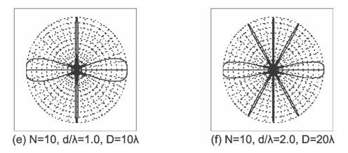
Figure 5-3 Further examples of radiation patterns for d/λ
