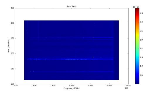
This waterfall chart shows the telescope scanning to and from the sun. From approximately second 180 to second 250 the overall noise level is higher, showing that the Sun was detected and affected noise levels.
