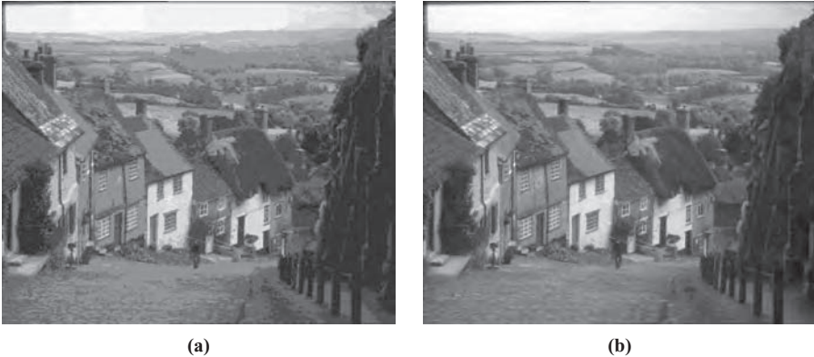
Figure 27-4 The Goldhill image compressed at 64:1 using (a) one-level DWT and (b) four-level DWT.
