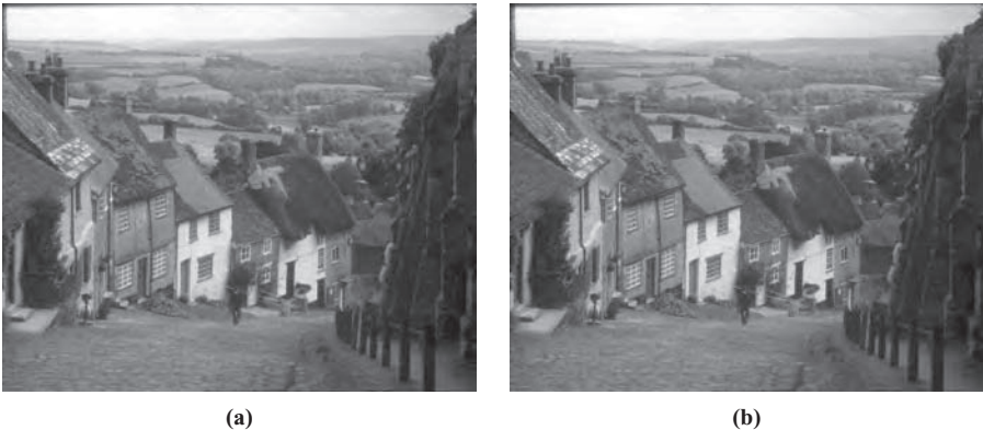
Figure 27-3 The Goldhill image compressed at 16:1 using (a) one-level DWT and (b) two-level DWT.
