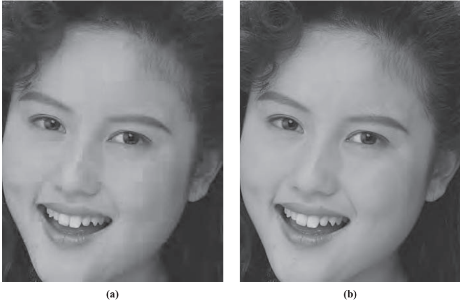
Figure 27-1 The Woman image compressed at 100:1 with tile size (a) 64 \times 64 and (b) 256 \times 256 .
