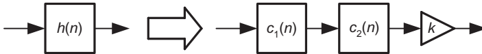
Figure 2-3 Direct form of h(n) and the equivalent cascade form using c_1(n) , c_2(n) , and k .
