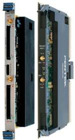
Model 6821 commercial (left) and conduction-cooled version
