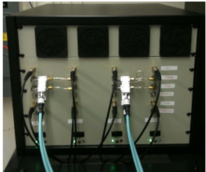
FIG. 4. Custom crate to house up to eight ROACH assemblies. The SMA connectors to each IF board are visible on the front panel.
