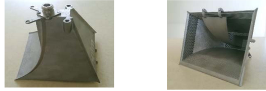
Fig. 20 DRA antenna without geopolymer and resistive loads
