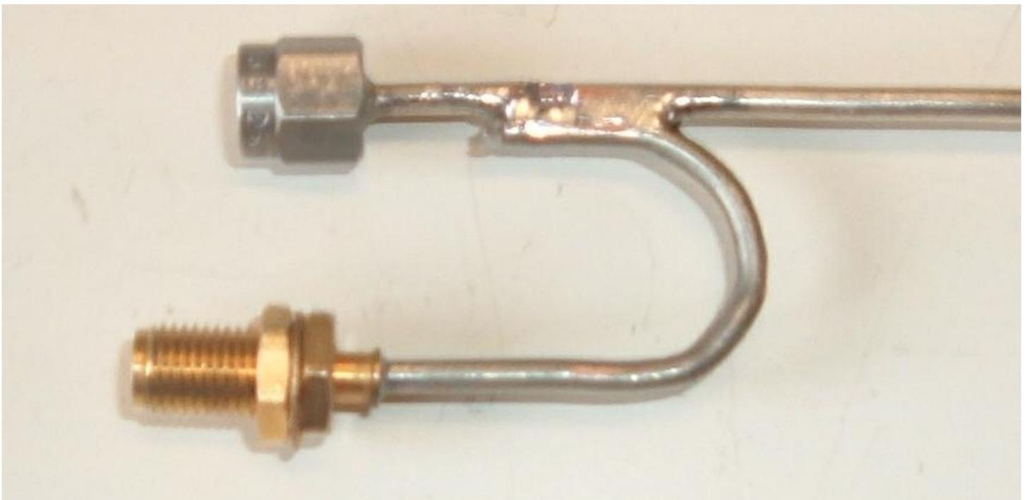
To form the IF Port connection, fit a very thin wire 5-6 mm long (coiled turns are not really necessary) from the inner conductor of the main OSC cable to the inner of the IF cable. See below this very thin RFC connection.
