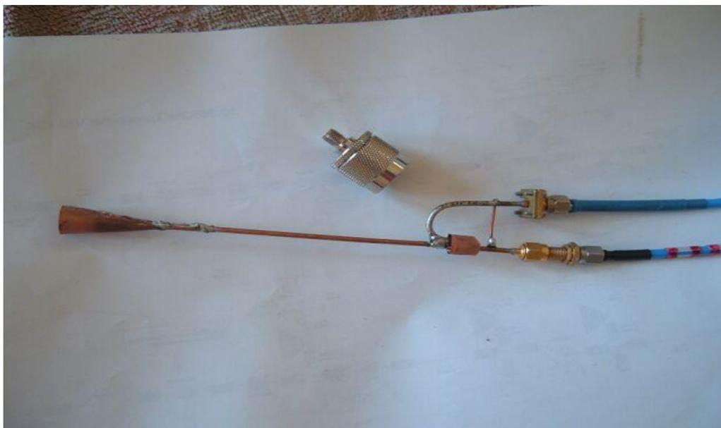
The “coaxial” mechanism that I have used is not my own design. The concept however has been around for decades. The technique I have used is to simply “pump” a pair of RF/Microwave diodes connected in series in a “coaxial” environment rather than the usual Waveguide scenario. The usual term for these series diodes is “Antiphase”. I then couple my IF Port to these “pumped” diodes via a simple RFC/Diplexer function.
