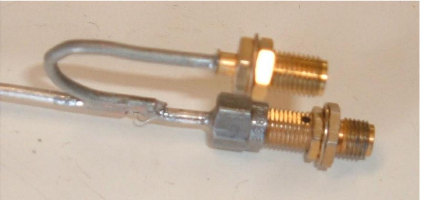
This RFC/IF connection forms a Diplexer. It will be vulnerable to damage so a small protective cover as per the first Photo in this article will need to be soldered in place to protect this Diplexer connection. A piece of 2mm wire soldered between the sides of the IF loop in the first Photo provides additional rigidity. There should be minimal degradation when converting any 2 Port Mixer to a 3 Port Mixer.
