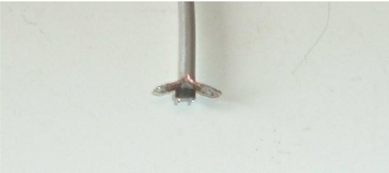
Being careful not to crush the easily damaged diode package, bend the .085 flaps towards the diode body to permit soldering to the 2 connection points of the diode.
