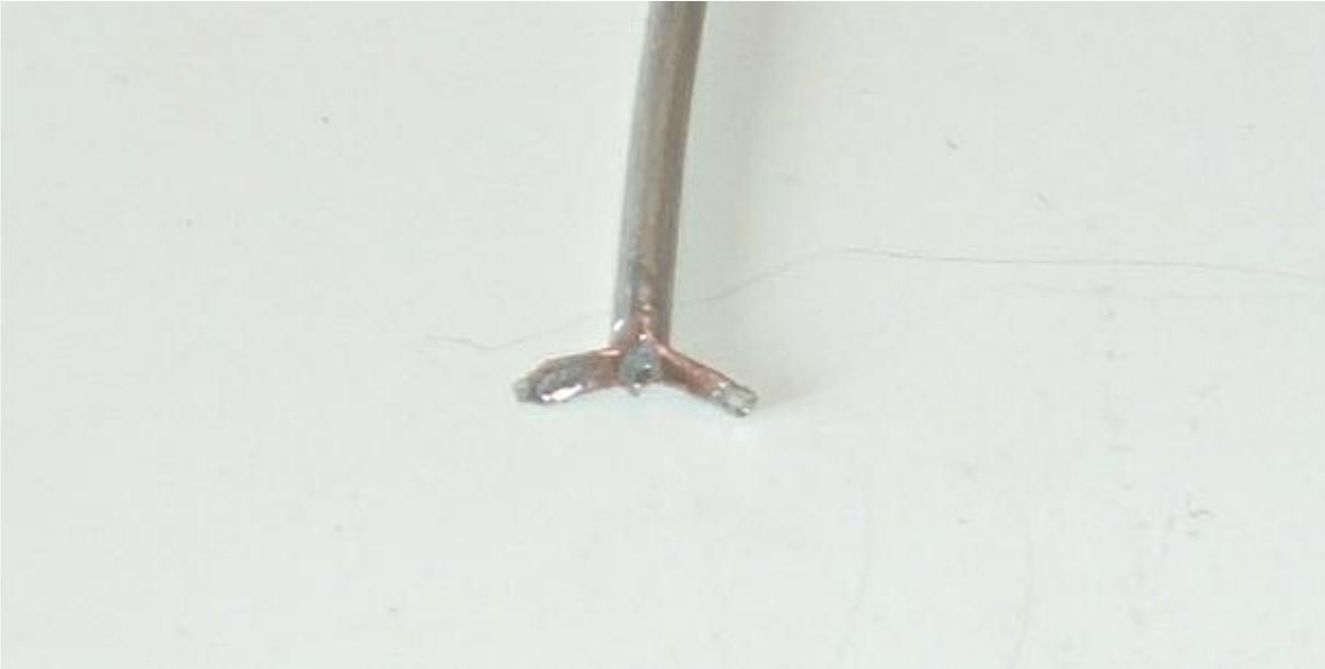
Solder the single tab of the diode package to the inner conductor as per below.
