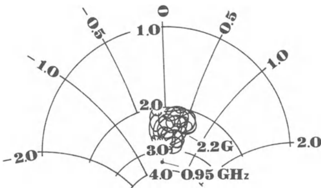
Fig. 11.2 Measured input impedance of M-S type MSCA ( Z_0 = 50 \Omega ).
