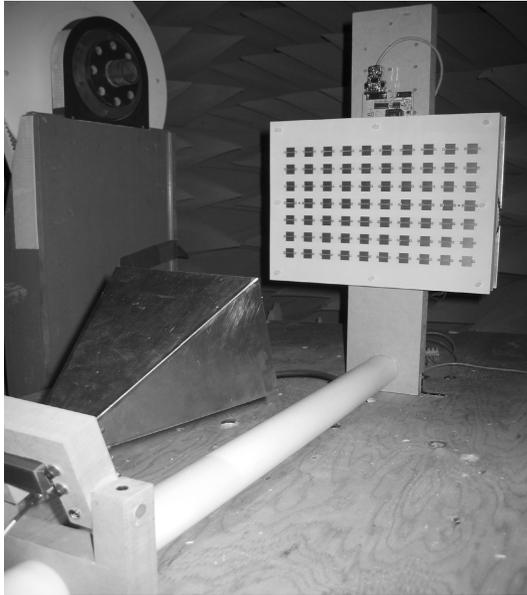
**Figure 7.65.** Photo of the 70-element C-band beam scanning reflectarray with tunable varactor diodes. (Courtesy of Dr. Sean Hum and Prof. Michal Okoniewski of Univ. of Calgary, Canada.)
