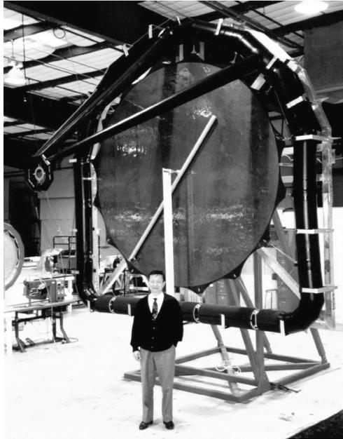
**Figure 7.3.** 3-m diameter Ka-band inflatable reflectarray.
