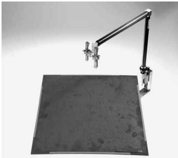
Figure 4.26 Photograph of 45.0 cm \times 45.0 cm dual-band CP reflectarray. (© 2006 IEE. From: [11]. Reprinted with permission. )
