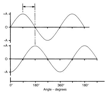
Figure 1.3 Phase difference between two waveforms
