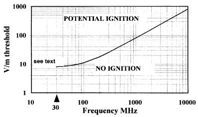
**Figure 4.15** Safe thresholds gas group 2c – CW (single transmission)
