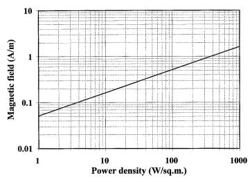
Figure A1.2 Power density values (Wm<sup>-2</sup>) versus magnetic field plane wave values (Am<sup>-1</sup>)
