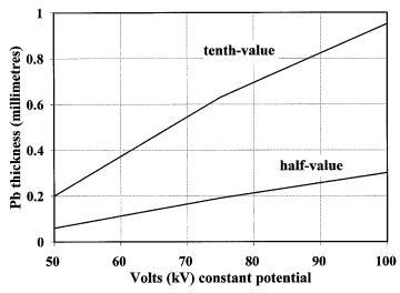
**Figure 11.5** Half and one tenth value layer thickness for lead shielding (Courtesy of BSI London)
