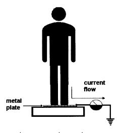
Figure 3.4 Limb current measurement concept
