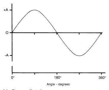
Figure 1.1 Sine wave illustration
