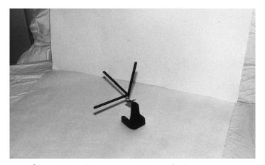
Figure 7.3 Sensor isotropic antennas – electric field
