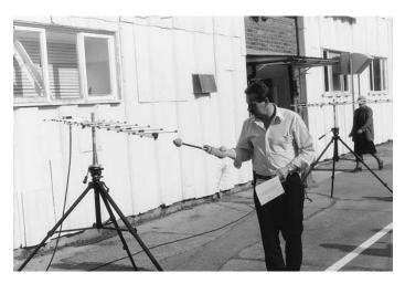
**Figure 12.1** Yagi antenna fed by 100 W source for training exercises (Courtesy TUV Fareham)
