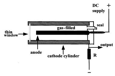
Figure 8.12 GM X-ray counter tube (Courtesy Philips Electronic tubes)
