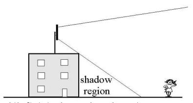
Figure 6.16 Shadowing of coverage from roof-mounted antennas
