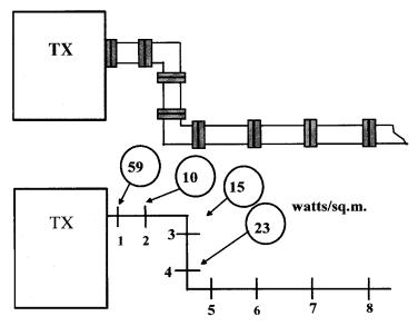
Figure 9.10 Leakage testing - waveguide runs
