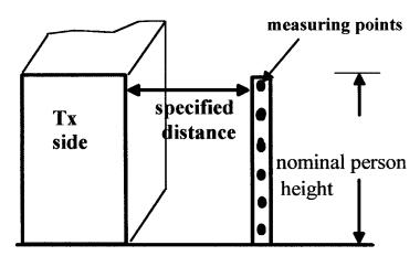
Figure 10.4 Exposure due to leakage – another method of specification
