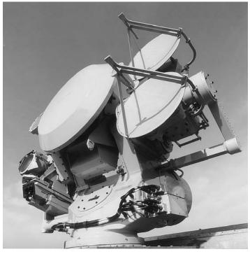
Seawolf tracker radar and gunfire control system (Courtesy Alenia Figure 2.21 - Marconi)
