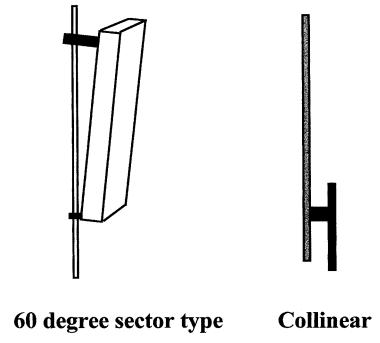
Figure 6.8 Examples of omni-directional and sectoral antennas
