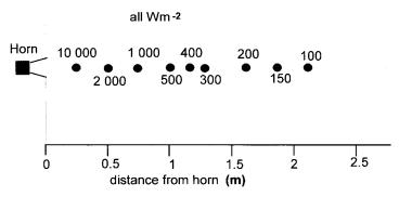
Figure 10.16 Axis power density calculation for Figure 10.15
