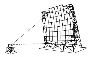
Figure 10.15 Fixed tropospheric scatter installation
