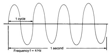
Figure 1.2 Sine wave frequency and time relationship
