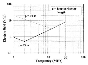
Field strength safety limits for the 1 to 30 MHz band calculated **Figure 10.17** from BS6656:1991 for flammable vapours, gas group 2c
