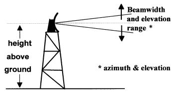
Figure 9.2 Positional data for rotating and fixed microwave antennas
