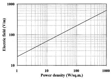
Figure A1.1 Power density values (Wm<sup>-2</sup>) versus electric field plane wave values (Vm<sup>-1</sup>)
