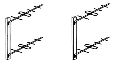
Figure 6.9 Stacked Yagi antennas
