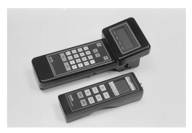
**Figure 7.10** Narda type 8718/8712 digital RF radiation meter (Courtesy Narda Safety Test Systems)
