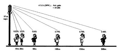
Figure 6.15 Measured levels from mast-mounted antennas as a percentage of a permitted level of 2Wm<sup>-2</sup> (Courtesy of C&W Communications)
