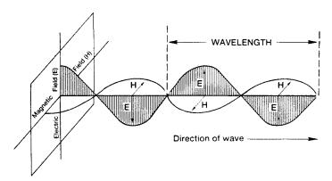
Figure 1.4 Representation of a plane wave
