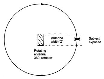
Figure 5.14 Rotating beam power density time-averaging for a subject in the near field case
