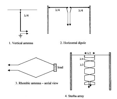
Figure 2.5 Simple HF antennas
