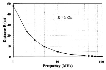
**Figure 5.15** Plot of  $\lambda/2\pi$  versus distance for 1 to 100 MHz
