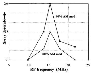
Figure 8.7 High power HF broadcast transmitter X-ray leakage investigation
