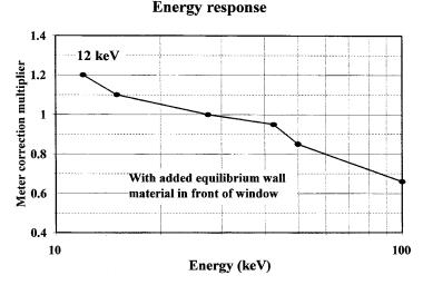
Figure 8.17 Victoreen 440RF/D energy response (Courtesy Victoreen Inc.)
