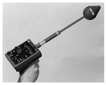
Figure 7.12 GMC Raham 495 meter unit and probe (Courtesy General Microwave Corp.)
