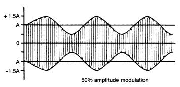
Figure 1.5 RF signal, amplitude modulated by a low frequency signal
