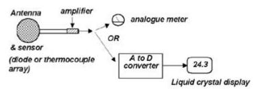
Figure 7.2 Schematic illustration of analogue and digital instrument concepts
