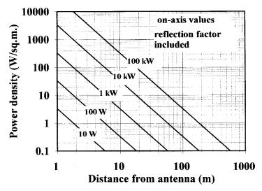
Figure 5.19 Transmission on-axis power densities for various power values
