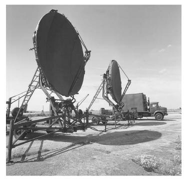
Figure 2.12 Tactical tropospheric scatter (Courtesy Marconi Electronic Systems)
