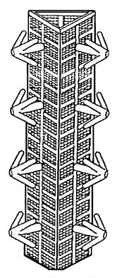
Figure 2.10 VHF antennas – typical broadcasting type
