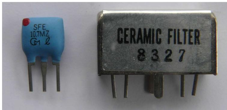
Figure 73. 10.7MHz ceramic IF filters.
