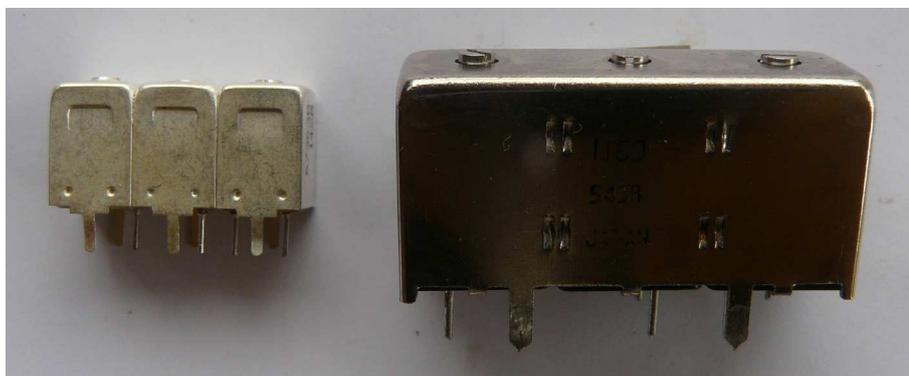
Figure 48. Commercial Helical Filters. Temwell Left, Toko Right.
