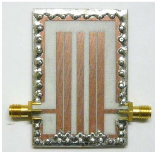
Figure 70. Comblin filter hardware.
