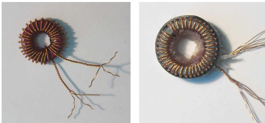
Figure 5. A trifilar wound RF Transformer (left) and a penta-filar transformer (right).
