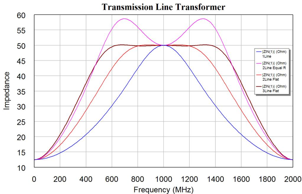
Figure 2. Plot of impedance variation versus frequency.
