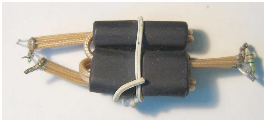
Figure 18. Circuit of hybrid in figure 17
