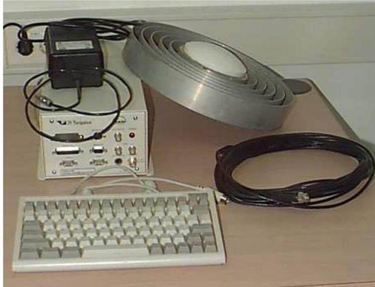
Figure 3.14: MAN / 3S Navigation GNSS-200 GPS/GLONASS receiver.
