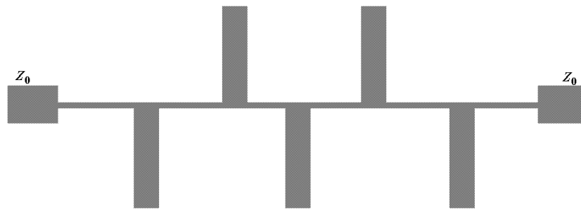
FIGURE 23.3. Stub low-pass filter example (not drawn to scale)
