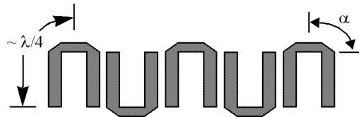
FIGURE 23.57. Hairpin bandpass filter (input-output couplings not shown)
