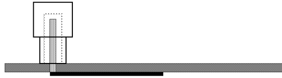
FIGURE 7.18. Unorthodox mounting method for bulkhead BNC (side view)
