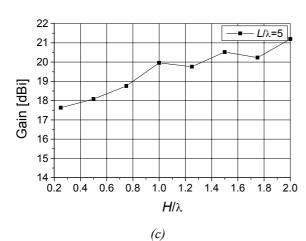
Figure 2. Maximal antenna gain versus normalized truncated-cone height for normalized helix lengths (a)  $L/\lambda = 1$ , (b)  $L/\lambda = 2$ , and (c)  $L/\lambda = 5$
