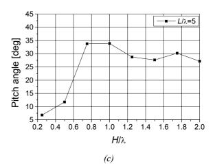
Figure 3. Optimal pitch angle versus normalized truncated-cone height for normalized helix lengths (a)  $L/\lambda = 1$ , (b)  $L/\lambda = 2$ , and (c)  $L/\lambda = 5$
