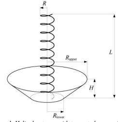
*Figure 1. Helical antenna with truncated-cone reflector*
