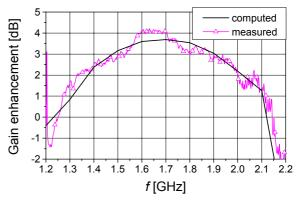
Figure 6. Computed and measured enhancement of helix gain [1]
