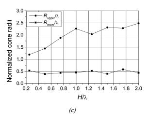
Figure 5. Optimal normalized upper and lower cone radii versus normalized truncated-cone height for normalized helix lengths (a)  $L/\lambda = 1$ , (b)  $L/\lambda = 2$ , and (c)  $L/\lambda = 5$
