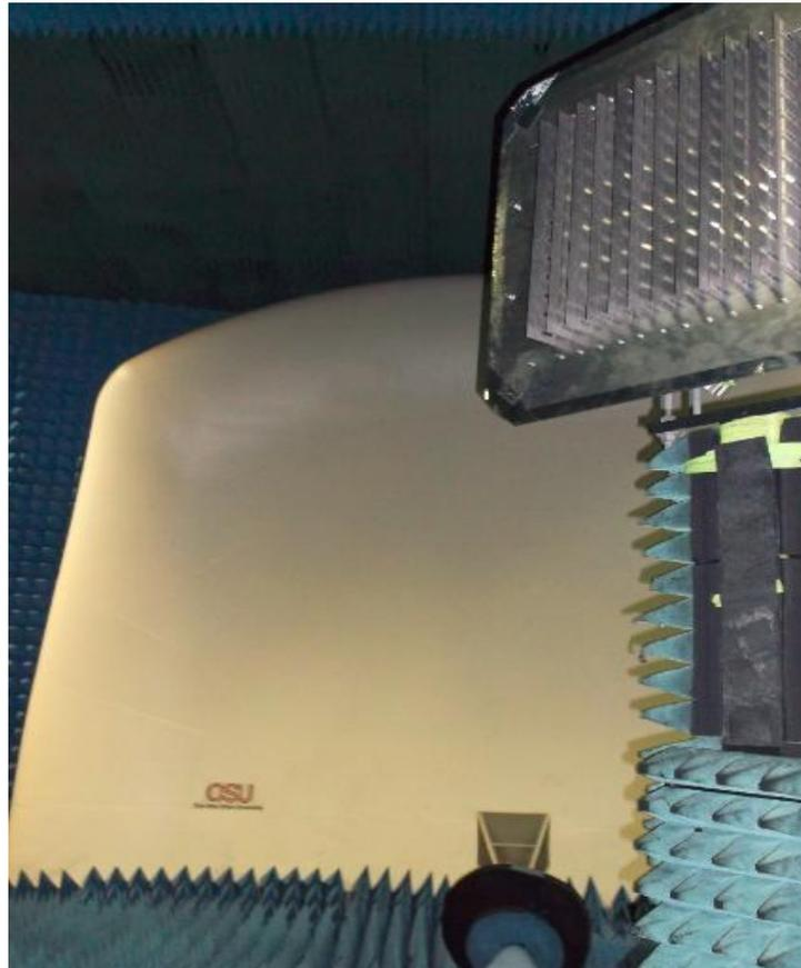
Figure 4.3: Far-field measurement setup in The Ohio State University anechoic chamber.
