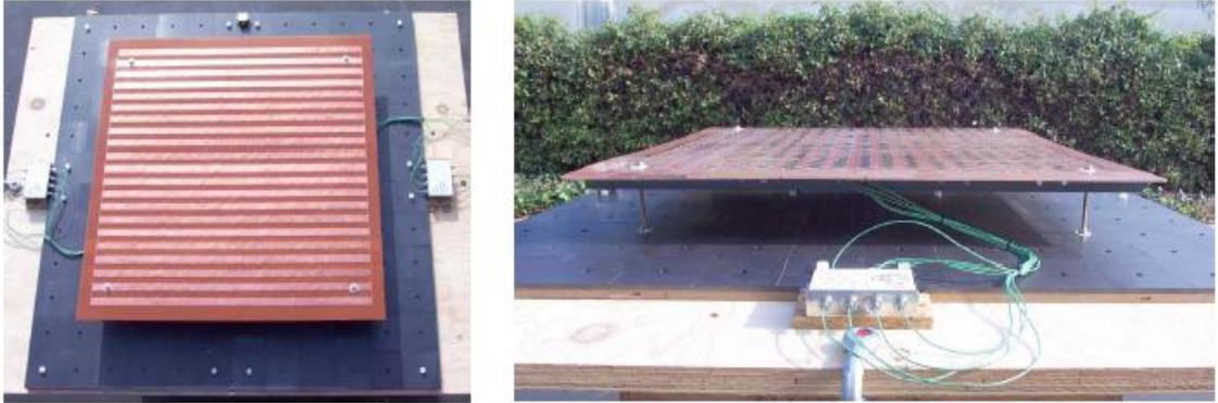
Figure 1.6: Ferrite loaded slot array from [33], ©2008 IEEE.
