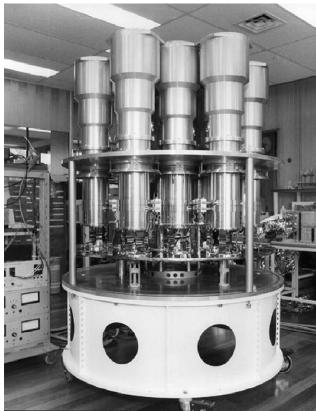
Figure 18.15 The 13-element multibeam feed system for the Parkes (Australia) radio telescope.
