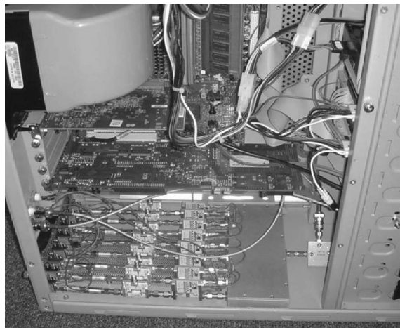
Figure 25.45 Inside view of the case housing the eight-channel RF–IF chain, ADC, and the data capturing and processing computer.
