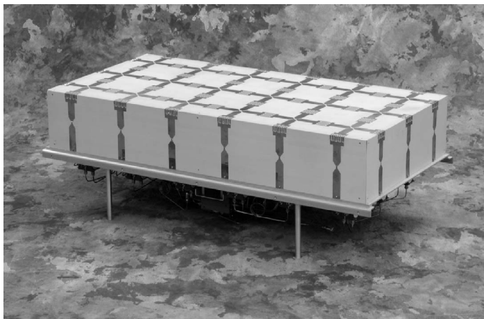
Figure 12.20 CSA breadboard designed for 110-MHz to 1-GHz operation.
