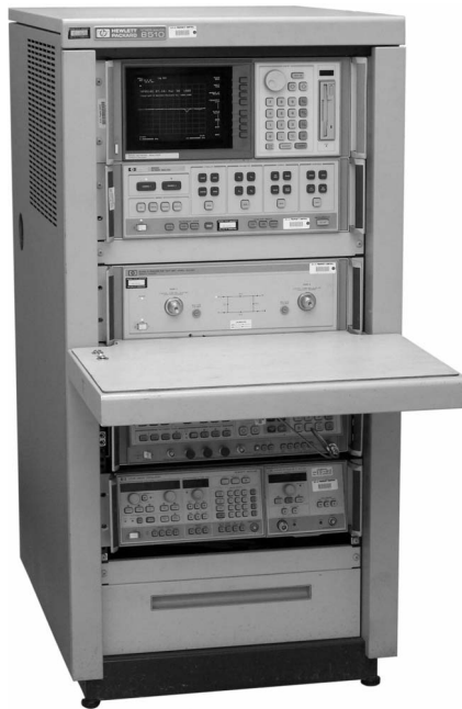
Figure 20.35 The HP8510 vector network analyzer has become a fairly common antenna-range instrumentation.
