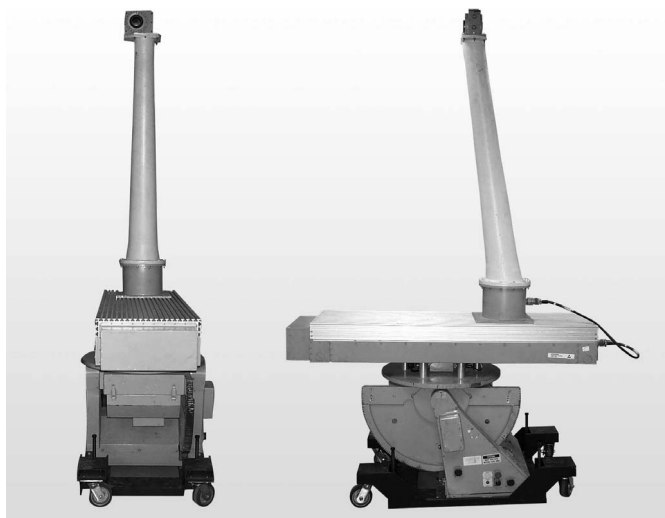
Figure 20.37 The front and side views of a model tower positioning system. A roll axis is located at the top of the tower, which is mounted on a fore-aft linear offset axis. This in turn is mounted on the azimuthal table of an AZ/EL positioner.
