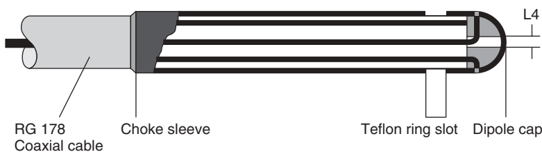
Figure 27.8 A dipole antenna with a coaxial choke. The two hemi-ellipsoidal caps make up the two arms of the dipole. (From Ref. 55.)
