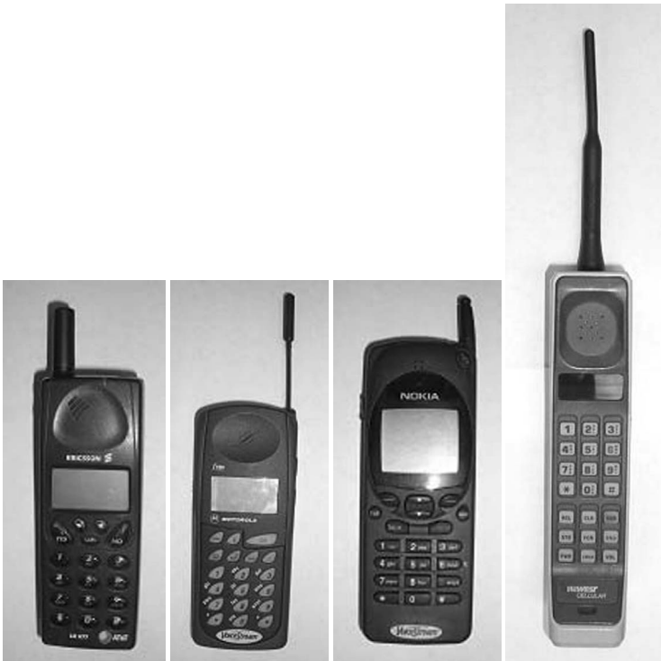
Figure 2.23 Examples of stationary and retractable/telescopic monopole antennas used in commercial cellular telephones.
