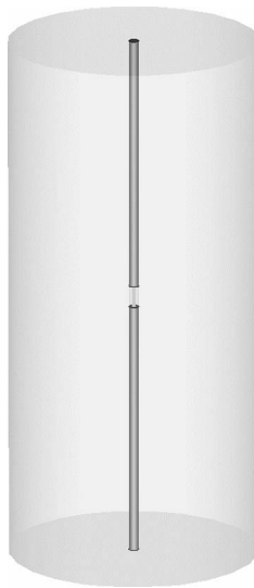
Figure 10.19 Depiction of the straight-wire dipole enclosed with a dielectric cylinder. The dipole has an overall length of 12.6 cm. The diameter of the dielectric cylinder ranges from 0.5 to 5 cm.
