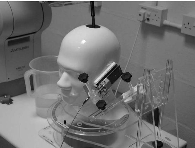
Figure 22.39 SAR measurement of U-slotted PIFA antenna.
