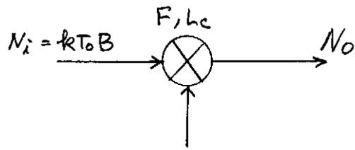
$$N_o = \underbrace{\frac{kT_0B}{L_c}}_{\text{INPUT NOISE}} + \underbrace{\frac{kT_0B(F-1)}{L_c}}_{\text{MIXER NOISE}} = \frac{kT_0BF}{L_c} \checkmark$$
