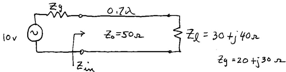
By Smith chart,  $Z_{in} = 56.6 - j61.1 \Omega$ . Then (assuming peak voltages), since the line is lossless,
