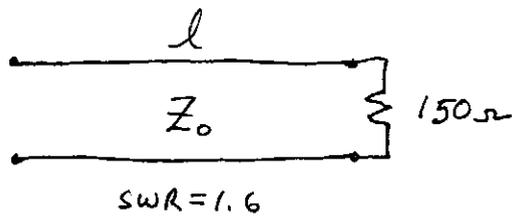
From (2.23),  $SWR = \frac{1+|\Gamma|}{1-|\Gamma|}$  so  $|\Gamma| = \frac{SWR-1}{SWR+1} = \frac{0.6}{2.6} = 0.231$
