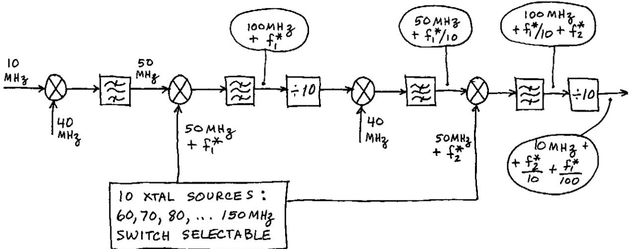
Two 10-position switches are used to select  $f_1^*$  and  $f_2^*$  individually as 10, 20, 30, ... 100 MHz. A 10 MHz and a 40 MHz source are also needed.
