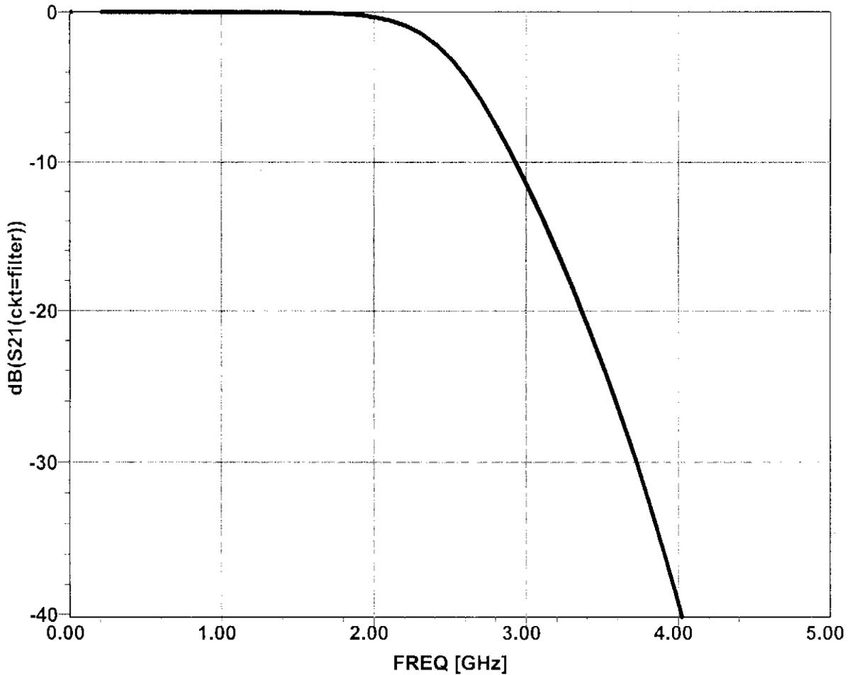
5.10  $f_0 = 2.5 \text{ GHz}$ , BAND-STOP,  $\Delta = 0.5$ ,  $N = 4$ , MAXIMALLY-FLAT,  $Z_0 = 50 \Omega$ , SHUNT STUBS.
