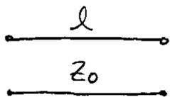
For  $I_2=0$ ,  $V_1 = V^+(e^{j\beta l} + e^{-j\beta l}) = 2V^+ \cos \beta l$
