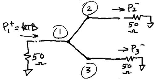
$$\begin{aligned} P_1^+ &= T & P_1^- &= T/2 + T/2 \\ P_2^+ &= T & P_2^- &= T/2 + T/4 + T/4 \\ P_3^+ &= T & P_3^- &= T/2 + T/4 + T/4 \\ \hline \sum P_i^+ &= 3T & \sum P_i^- &= 3T \checkmark \\ & & (\text{EQUILIBRIUM}) & \end{aligned}$$
