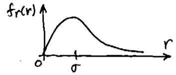
$$\frac{d f_r(r)}{d r} = \frac{e^{-r^2/2\sigma^2}}{\sigma^2} + \left(\frac{r}{\sigma^2}\right) \left(\frac{-r}{\sigma^2}\right) e^{-r^2/2\sigma^2} = 0$$
