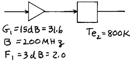
From (3.64),  $F_2 = 1 + \frac{T_{e2}}{T_0} = 1 + \frac{800}{290} = 3.76$
