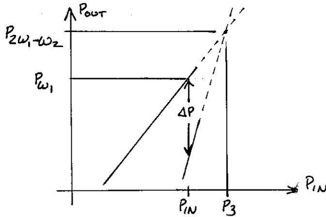
$$P_{W_1} = P_{in} + b_1 \quad (\text{EQ. OF LINE, SLOPE} = 1)$$
