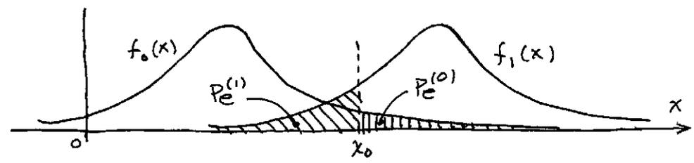
$$\frac{\partial P_e}{\partial x_0} = -P_0 f_0(x_0) + P_1 f_1(x_0) = 0, \text{ since } \frac{\partial}{\partial x} \int_a^x f(y) dy = f(x).$$
