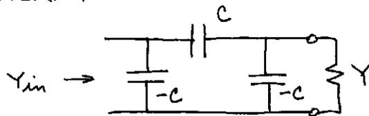
$$Y_{in} = -j\omega c + \left[ \frac{1}{j\omega c} + \frac{1}{Y - j\omega c} \right]^{-1} = -j\omega c + \frac{j\omega c Y + \omega^2 c^2}{Y - j\omega c + j\omega c} = -j\omega c + j\omega c + \frac{\omega^2 c^2}{Y}$$
