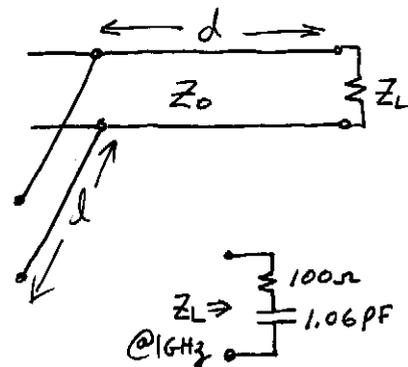
(VERIFIED WITH ANALYSIS WITH SERENADE WITH  $C = \frac{1}{2\pi f X_L} = 1.06 \text{ pF}$  at  $16 \text{ GHz}$ )
