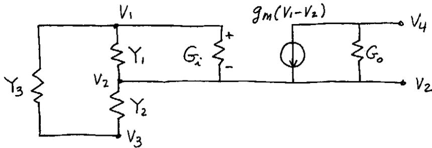
Writing KCL for nodes  $V_1, V_2, V_3, V_4$ :
