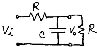
$$H(f) = \frac{V_o}{V_i} = \frac{Y_{j\omega C}}{R + Y_{j\omega C}} = \frac{1}{1 + j\omega RC} = \frac{1}{1 + jf/f_c} \quad \text{where } f_c = \frac{1}{2\pi RC}$$
