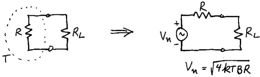
$$P_L = \left[ \frac{V_n R_L}{R + R_L} \right]^2 \frac{1}{R_L} = \frac{4kTB R R_L}{(R + R_L)^2}$$
