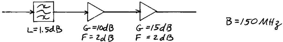
a)  $F = F_1 + \frac{F_2 - 1}{G_1} + \frac{F_3 - 1}{G_1 G_2} = 1.41 + \frac{(1.58 - 1)}{1/1.41} + \frac{(1.58 - 1)}{10/1.41} = 2.31 = \underline{\underline{3.6\text{dB}}}$  ✓
