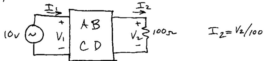
$$V_1 = AV_2 + BI_2 = (A + B/100)V_2$$
