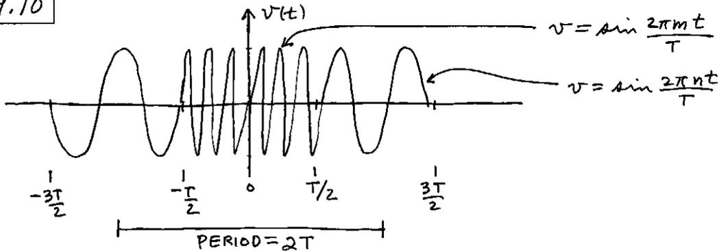
This is an odd function of  $t$  as defined above, so we can use a Fourier sine series:
