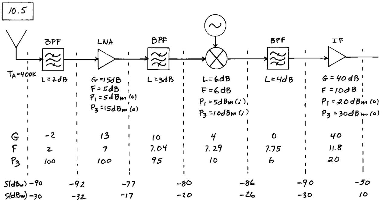
(a) overall noise figure is  $F_{REC} = 11.8 \text{ dB} \checkmark = 15.1$
