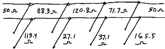
All lines and stubs are  $\lambda/8$  long at 2.5 GHz. The simulated filter response is shown below:
