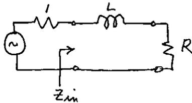
$N=1, \omega_c=1, 1\text{dB EQUAL RIPPLE}$
