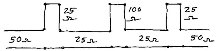
All lines and stubs are  $\lambda/8$  long at  $2.5 \text{ GHz}$ . The simulated filter response is shown below.
