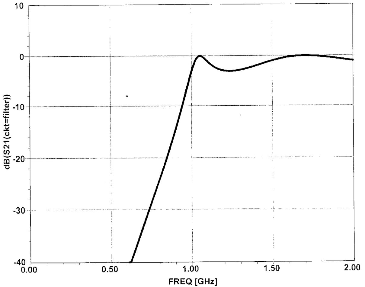
5.5  $f_0 = 2\text{GHz}$ , BANDPASS, MAXIMALLY FLAT GROUP DELAY
