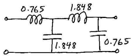
If Richard's transform is used with stub lengths of  $\lambda/4$  at  $f_0$ , a bandstop response can be achieved, since the s.c. stubs (series L) will look like opens, while the o.c. stubs (shunt C) will look like shorts. Also the values of  $Z, Y$  must be scaled by  $\gamma = \cot[\frac{\pi}{2}(1 - \frac{\Delta}{2})] = 0.414$  so that the stub impedances/admittances will be unity at the band edges. Thus we have,
