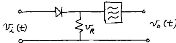
$$\text{For DSB-LC, } v_i(t) = A[1 + m(t)] \cos \omega_{IF} t$$
