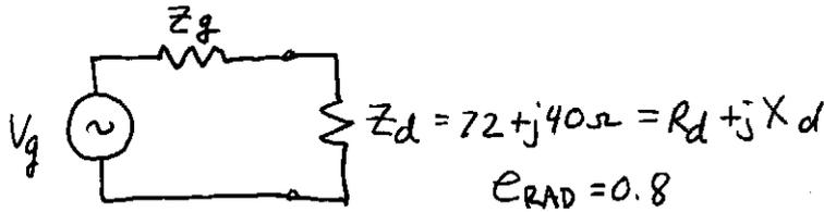
Maximum power transfer will occur when the generator is conjugately matched to the load. Thus,  $Z_g = Z_d^* = 72 - j40 \Omega$ . The power delivered to the antenna is,
