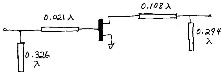
Analysis using Serenade gives  $RL_1 = 10 \text{ dB}$ ,  $RL_2 = 18 \text{ dB}$ ,
