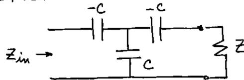
$$Z_{in} = \frac{j}{\omega c} + \left[ j\omega c + \frac{1}{Z + j/\omega c} \right]^{-1} = \frac{j}{\omega c} + \frac{Z + j/\omega c}{1 + j\omega c Z - 1} = \frac{j}{\omega c} + \frac{-j + j/\omega c Z}{\omega c}$$
