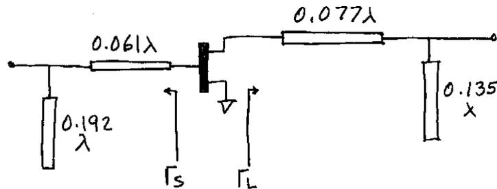
Since the gain with this  $\Gamma_s, \Gamma_p$  is 10 dB, the input power for a 1W output is,
