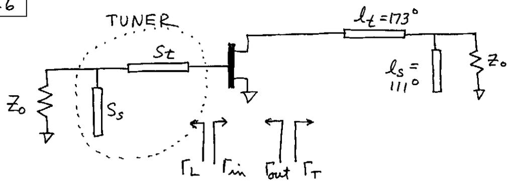
As in Example 8.4, choose  $\Gamma_L = 0.6 \angle -130^\circ$ . Then  $\Gamma_{out}$ ,  $Z_{out}$ ,  $Z_T$ ,  $l_t$ , and  $l_s$  are unchanged. Then we have the matching problem of using a stub tuner to match  $50\Omega$  to  $\Gamma_L$ . The stub susceptance is  $jB_s = +j1.56$ , for a stub length of  $S_s = 0.158\lambda$ . The line length is  $S_t = 0.004\lambda$ .
