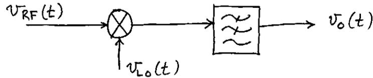
$$v_{RF}(t) = V_U \cos(\omega_{LO} + \omega_{IF})t + V_L \cos(\omega_{LO} - \omega_{IF})t$$
