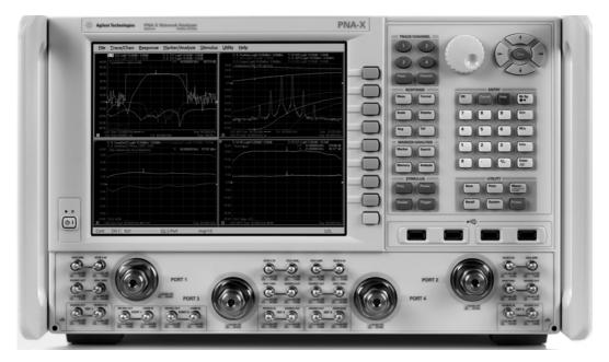
FIGURE 4.7 Photograph of the Agilent N5247A Programmable Network Analyzer. This instrument is used to measure the scattering parameters of RF and microwave networks from 10 MHz to 67 GHz. The instrument is programmable, performs error correction, and has a wide variety of display formats and data conversions. Courtesy of Agilent Technologies.
