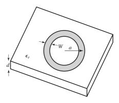
**6.17** A circular microstrip disk resonator is shown below. Solve the wave equation for  $\text{TM}_{nm0}$  modes for this structure, using the magnetic wall approximation that  $H_{\varphi} = 0$  at  $\rho = a$ . If fringing fields are neglected, show that the resonant frequency of the dominant mode is given by
