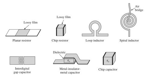
Resistors are fabricated with thin films of lossy material such as nichrome, tantalum nitride, or doped semiconductor material. In monolithic circuits such films can be deposited or grown, whereas chip resistors made from a lossy film deposited on a ceramic chip can be bonded or soldered in a hybrid circuit. Low resistances are hard to obtain.
