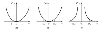
**FIGURE 8.28** Frequency scaling for low-pass filters and transformation to a high-pass response. (a) Low-pass filter prototype response for  $\omega_c = 1$  rad/sec. (b) Frequency scaling for low-pass response. (c) Transformation to high-pass response.
