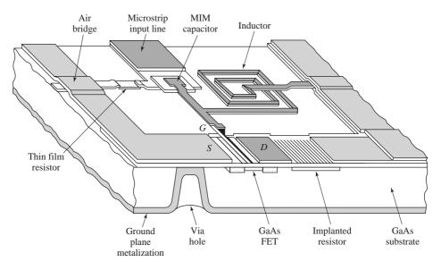
FIGURE 11.26 Layout of a monolithic microwave integrated circuit.
