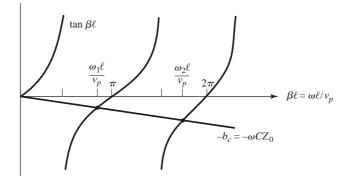
**FIGURE 6.17** Solutions to (6.78) for the resonant frequencies of the gap-coupled microstrip resonator.
