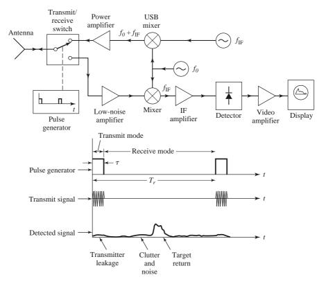
FIGURE 14.21 A pulse radar system and timing diagram.
