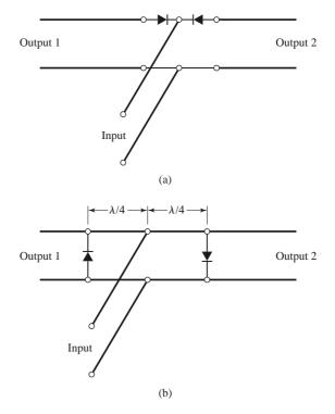
FIGURE 11.9 Circuits for single-pole, double-throw PIN diode switches. (a) Series. (b) Shunt.
