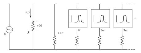
FIGURE 13.21 Conceptual circuit for the derivation of power relations in a resistive frequency multiplier.
