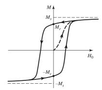
FIGURE 9.16 A hysteresis curve for a ferrite toroid.
