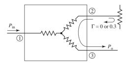
**7.9** Consider the general resistive divider shown below. For an arbitrary power division ratio  $\alpha = P_2/P_3$ , derive expressions for the resistors  $R_1$ ,  $R_2$ , and  $R_3$ , and the output characteristic impedances  $Z_{o2}$  and  $Z_{o3}$  so that all ports are matched, assuming the source impedance is  $Z_0$ .
