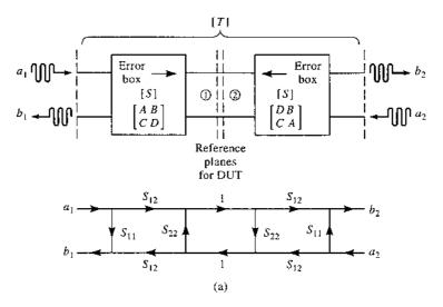
FIGURE 4.21a Block diagram and signal flow graph for the *Thru* connection.
