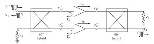
FIGURE 12.11 A balanced amplifier using 90° hybrid couplers.
