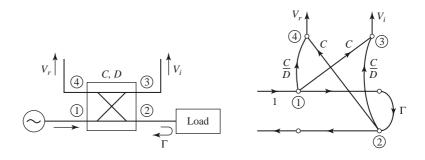
Realistic directional couplers, however, have finite directivity, which means that both incident and reflected powers will contribute to both  $V_i$  and  $V_r$ , leading to an error. If we assume a unit incident wave from the source, inspection of the signal flow graph leads to the following expressions for  $V_i$  and  $V_r$ :
