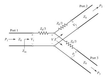
FIGURE 7.7 An equal-split three-port resistive power divider.
