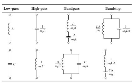
TABLE 8.6Summary of Prototype Filter Transformations $\left(\Delta = \frac{\omega_2 - \omega_1}{\omega_0}\right)$
