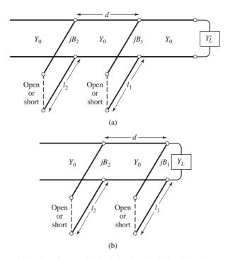
**FIGURE 5.7** Double-stub tuning. (a) Original circuit with the load an arbitrary distance from the first stub. (b) Equivalent circuit with the load transformed to the first stub.
