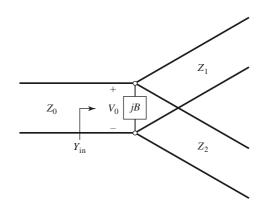
FIGURE 7.6 Transmission line model of a lossless T-junction divider.
