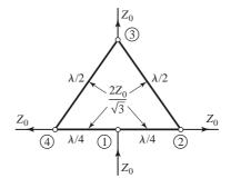
**7.32** For the symmetric hybrid shown below, calculate the output voltages if port 1 is fed with an incident wave of  $1\angle 0$  V. Assume that the outputs are matched.
