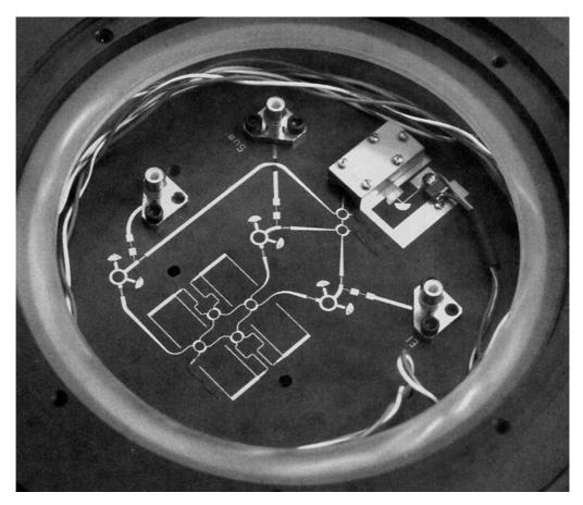
**FIGURE 13.30** Photograph of a 35 GHz microstrip monopulse radar receiver circuit. Three balanced mixers using ring hybrids can be seen, along with three stepped-impedance low-pass filters, and six quadrature hybrids. Eight feedlines are aperture coupled to microstrip antennas on the reverse side. The circuit also contains a Gunn diode source for the local oscillator.
