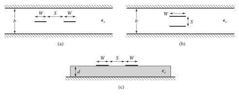
**FIGURE 7.26** Various coupled transmission line geometries. (a) Coupled stripline (planar, or edge-coupled). (b) Coupled stripline (stacked, or broadside-coupled). (c) Coupled microstrip lines.
