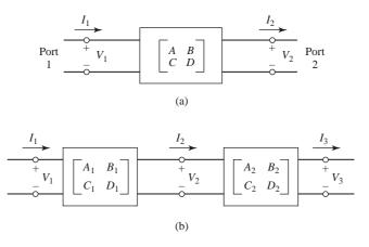
FIGURE 4.11 (a) A two-port network; (b) a cascade connection of two-port networks.
