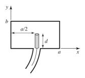
**4.35** Consider the infinitely long waveguide fed with two probes driven  $180^{\circ}$  out of phase, as shown below. What are the resulting excitation coefficients for the TE<sub>10</sub> and TE<sub>20</sub> modes? What other modes can be excited by this feeding arrangement?
