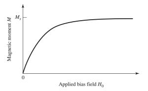
**FIGURE 9.2** Magnetic moment of a ferrimagnetic material versus bias field,  $H_0$ .
