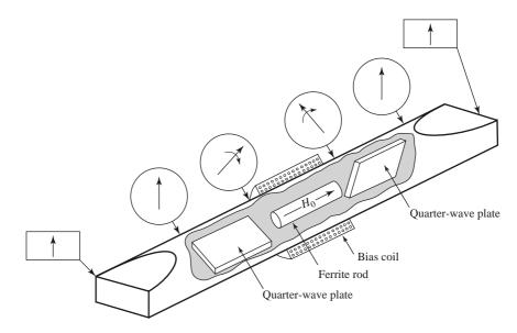
FIGURE 9.18 Nonreciprocal Faraday rotation phase shifter.
