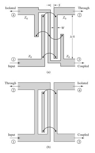
FIGURE 7.38 The Lange coupler. (a) Layout in microstrip form. (b) The unfolded Lange coupler.
