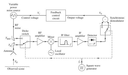
FIGURE 14.27 Balanced Dicke radiometer block diagram.
