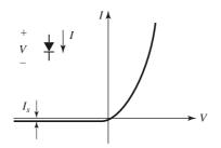
**FIGURE 11.2** *V*–*I* characteristics of a Schottky diode.
