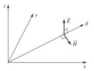
**FIGURE 1.8** Orientation of the  $\overline{E}$ ,  $\overline{H}$ , and  $\overline{k} = k_0 \hat{n}$  vectors for a general plane wave.
