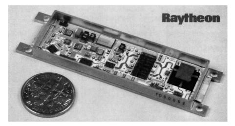
**FIGURE 11.25** Photograph of one of the 25,344 hybrid integrated T/R modules used in Raytheon's Ground Based Radar system. This X-band module contains phase shifters, amplifiers, switches, couplers, a ferrite circulator, and associated control and bias circuitry.
