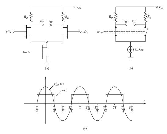
FIGURE 13.32 (a) A singly balanced differential FET mixer. (b) Simplified equivalent circuit. (c) LO voltage waveform and idealized switching waveform of the top left FET.
