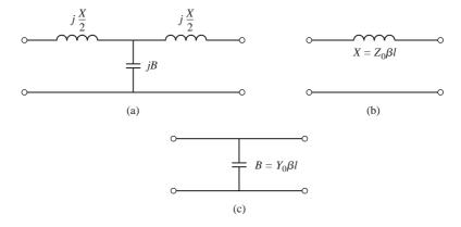
**FIGURE 8.39** Approximate equivalent circuits for short sections of transmission lines. (a) Tequivalent circuit for a transmission line section having  $\beta \ell \ll \pi/2$ . (b) Equivalent circuit for small  $\beta \ell$  and large  $Z_0$ . (c) Equivalent circuit for small  $\beta \ell$  and small  $Z_0$ .
