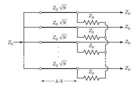
FIGURE 7.14 An *N*-way, equal-split Wilkinson power divider.
