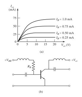
**FIGURE 11.19** (a) DC characteristics of an *npn* BJT; (b) biasing and decoupling circuit for an *npn* BJT.
