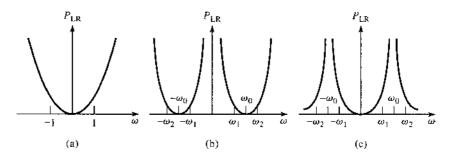
**FIGURE 8.31** Bandpass and bandstop frequency transformations. (a) Low-pass filter prototype response for  $\omega_c = 1$ . (b) Transformation to bandpass response. (c) Transformation to bandstop response.
