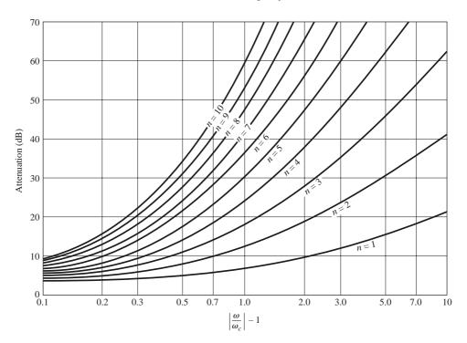
FIGURE 8.26 Attenuation versus normalized frequency for maximally flat filter prototypes. Adapted from G. L. Matthaei, L. Young, and E. M. T. Jones, *Microwave Filters, Impedance-Matching Networks, and Coupling Structures*, Artech House, Dedham, Mass., 1980, with permission.
