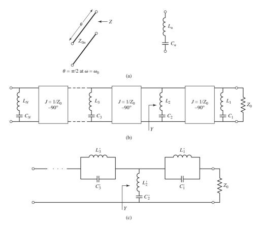
**FIGURE 8.48** Equivalent circuit for the bandstop filter of Figure 8.47a. (a) Equivalent circuit of an open-circuited stub for  $\theta$  near  $\pi/2$ . (b) Equivalent filter circuit using resonators and admittance inverters. (c) Equivalent lumped-element bandstop filter.
