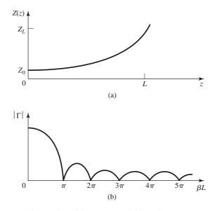
**FIGURE 5.19** A matching section with an exponential impedance taper. (a) Variation of impedance. (b) Resulting reflection coefficient magnitude response.
