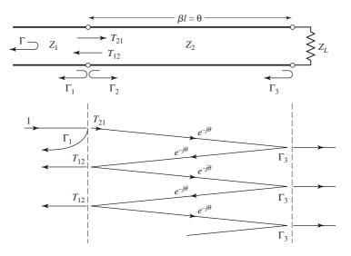
FIGURE 5.13 Partial reflections and transmissions on a single-section matching transformer.
