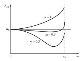
Variation of  $Z_{i\pi}$  in the passband of a low-pass *m*-derived section for various values **FIGURE 8.16** of *m*.
