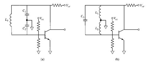
**FIGURE 13.3** Transistor oscillator circuits using a common emitter BJT. (a) Colpitts oscillator. (b) Hartley oscillator.
