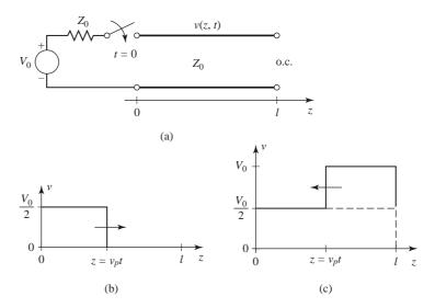
**FIGURE 2.23** Transient response of a transmission line terminated with an open circuit. (a) Transmission line circuit with a step function voltage source. (b) Response for  $0 < t < \ell/v_p$ . (c) Response for  $\ell/v_p < t < 2\ell/v_p$ ; the incident pulse is reflected with  $\Gamma = 1$ .
