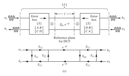
FIGURE 4.21c Block diagram and signal flow graph for the *Line* connection.
