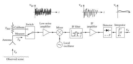
FIGURE 14.26 Total power radiometer block diagram.
