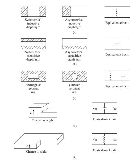
FIGURE 4.22 Rectangular waveguide discontinuities.
