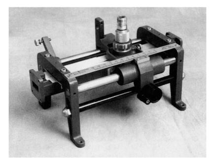
FIGURE 2.13 An X-band waveguide slotted line.
