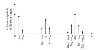
FIGURE 11.4 Output spectrum of a detected AM signal.
