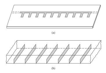
FIGURE 8.1 Examples of periodic structures. (a) Periodic stubs on a microstrip line. (b) Periodic diaphragms in a waveguide.
