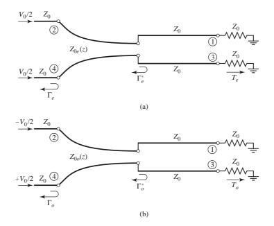
**FIGURE 7.48** Excitation of the tapered coupled line hybrid. (a) Even-mode excitation. (b) Odd-mode excitation.
