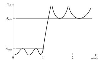
FIGURE 8.22 Elliptic function low-pass filter response.
