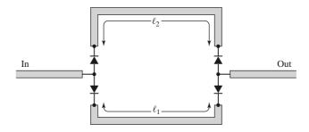
FIGURE 11.11 A switched-line phase shifter.
