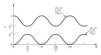
Coupled and through port voltages (squared) versus frequency for the coupled line coupler of Figure 7.31.
