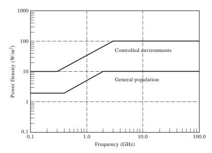
FIGURE 14.32 IEEE Standard C95.1-2005 recommended power density limits for human exposure to RF and microwave electromagnetic fields. For a controlled (occupational) environment the exposure is averaged over a 6 minute period, while for the general population the exposure is averaged over a 30 minute period.
