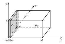
6.27 Derive an expression for the change in resonant frequency for the screw-tuned rectangular cavity of Example 6.8 if the screw is located at x = a/2, z = 0, where  $H_x$  is maximum and  $E_y$  is minimum.
