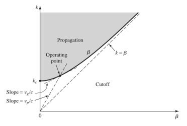
**FIGURE 8.4** k- $\beta$  diagram for a waveguide mode.
