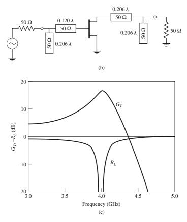
FIGURE 12.7 Continued. (b) RF circuit. (c) Frequency response.
