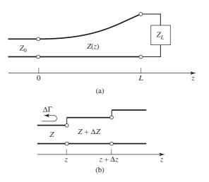
**FIGURE 5.18** A tapered transmission line matching section and the model for an incremental length of tapered line. (a) The tapered transmission line matching section. (b) Model for an incremental step change in impedance of the tapered line.
