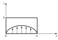
**FIGURE 4.2** Electric field lines for the  $TE_{10}$  mode of a rectangular waveguide.
