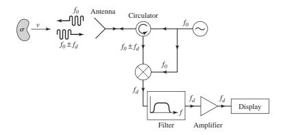
FIGURE 14.22 Doppler radar system.
