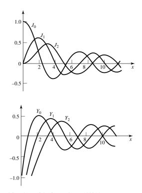
FIGURE C.1 Bessel functions of the first and second kind.
