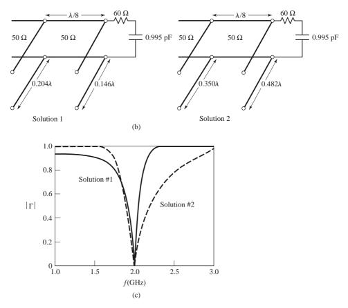
**FIGURE 5.9** Continued. (b) The two double-stub tuning solutions. (c) Reflection coefficient magnitudes versus frequency for the tuning circuits of (b).
