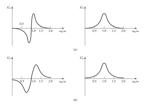
FIGURE 9.4Complex susceptibilities for a typical ferrite. (a) Real and imaginary parts of  $\chi_{xx}$ .<br/>(b) Real and imaginary parts of  $\chi_{xy}$ .
