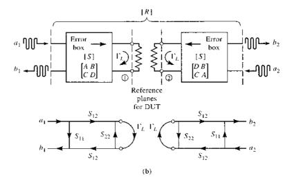
FIGURE 4.21b Block diagram and signal flow graph for the *Reflect* connection.
