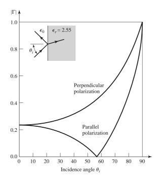
**FIGURE 1.14** Reflection coefficient magnitude for parallel and perpendicular polarizations of a plane wave obliquely incident on a dielectric half-space.
