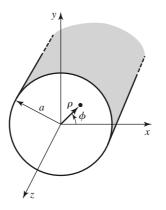
**FIGURE 3.11** Geometry of a circular waveguide.
