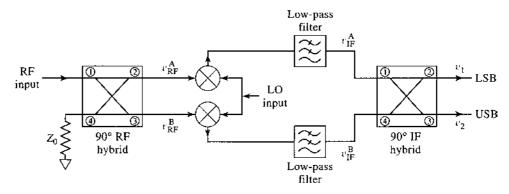
FIGURE 13.31 Circuit for an image reject mixer.
