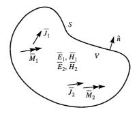
FIGURE 1.15 Geometry for the Lorentz reciprocity theorem.
