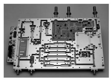
**FIGURE 8.55** Photograph of a wideband down converter. Multiple PIN diode switches, filter banks, amplifiers, and mixers are used to cover the range of 10 MHz to 27 GHz. Several types of filters can be seen in this module, including stub filters, coupled line filters, and stepped impedance filters. The microstrip stub filter at left is a low-pass 21-pole filter with a cutoff frequency of 5.4 GHz and more than 75 dB of rejection from 5.8 to 9.0 GHz.
