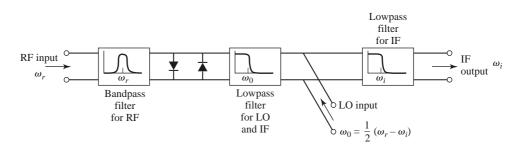
FIGURE 13.35 Subharmonically pumped mixer using an antiparallel diode pair.
