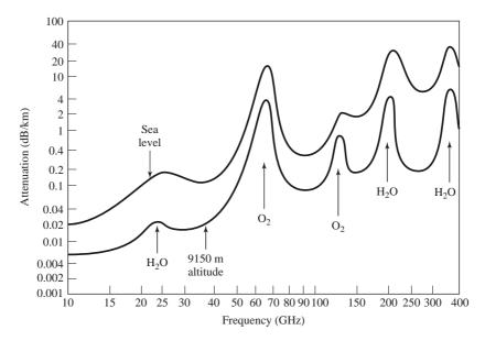
**FIGURE 14.29** Average atmospheric attenuation versus frequency (horizontal polarization).
