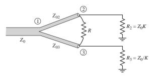
**FIGURE 7.13** A Wilkinson power divider in microstrip form having unequal power division.
