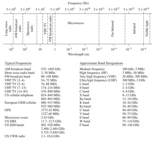
FIGURE 1.1 The electromagnetic spectrum.
