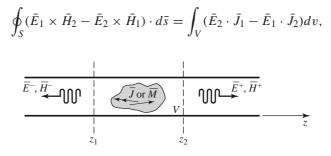
FIGURE 4.27 An arbitrary electric or magnetic current source in an infinitely long waveguide.
