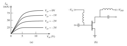
**FIGURE 11.22** (a) DC characteristics of an *n*-channel GaAs MESFET; (b) biasing and decoupling circuitry.
