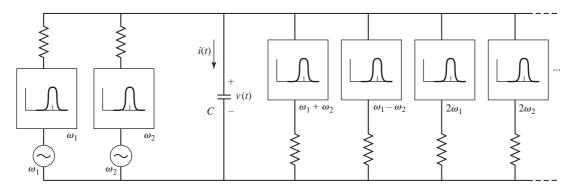
FIGURE 13.19 Conceptual circuit for the derivation of the Manley–Rowe relations.
