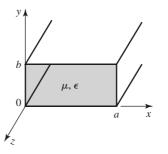
FIGURE 3.7 Geometry of a rectangular waveguide.
