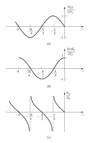
**FIGURE 2.6** (a) Voltage, (b) current, and (c) impedance  $(R_{in} = 0 \text{ or } \infty)$  variation along a shortcircuited transmission line.
