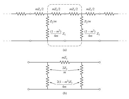
**FIGURE 8.15** Development of an *m*-derived  $\pi$ -section. (a) Infinite cascade of *m*-derived T-sections. (b) A de-embedded  $\pi$ -equivalent.
