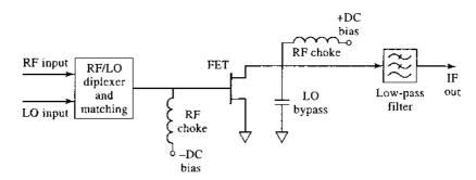
FIGURE 13.27 Circuit for a single-ended FET mixer.
