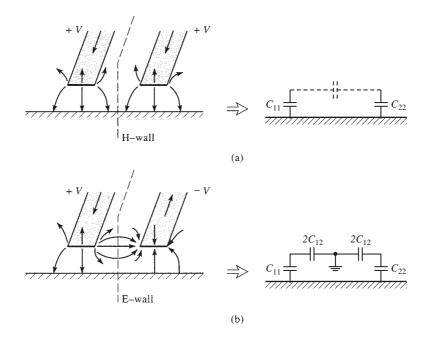
**FIGURE 7.28** Even- and odd-mode excitations for a coupled line, and the resulting equivalent capacitance networks. (a) Even-mode excitation. (b) Odd-mode excitation.
