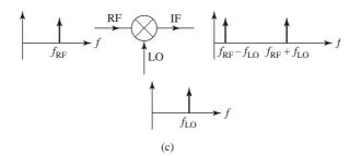
**FIGURE 11.1** Basic frequency conversion operations of rectification, detection, and mixing. (a) Diode rectifier. (b) Diode detector. (c) Mixer.
