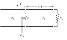
FIGURE 2.16 The quarter-wave matching transformer.
