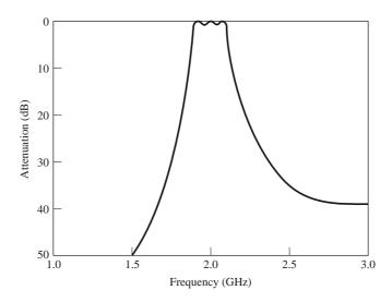
**FIGURE 8.51** Amplitude response for the capacitive-gap coupled series resonator bandpass filter of Example 8.9.
