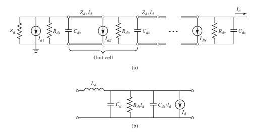
**FIGURE 12.15** (a) Transmission line circuit for the drain line of the distributed amplifier; (b) equivalent circuit of a single unit cell of the drain line.
