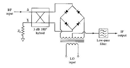
FIGURE 13.34 Double-balanced mixer circuit.
