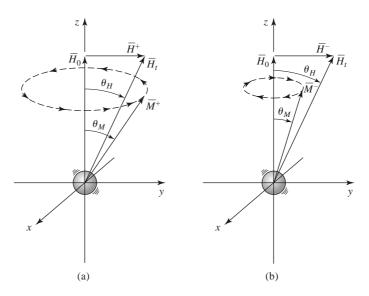
**FIGURE 9.3** Forced precession of a magnetic dipole with circularly polarized fields. (a) RHCP,  $\theta_M > \theta_H$ . (b) LHCP,  $\theta_M < \theta_H$ .
