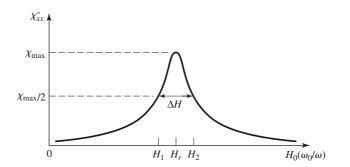
**FIGURE 9.5** Definition of the linewidth,  $\Delta H$ , of the gyromagnetic resonance.
