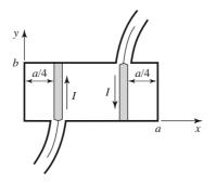
**4.36** Consider a small current loop on the sidewall of a rectangular waveguide, as shown below. Find the  $TE_{10}$  fields excited by this loop if the loop is of radius  $r_0$ .
