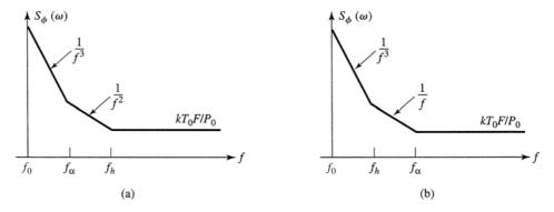
**FIGURE 13.17** Power spectral density of phase noise at the output of an oscillator. (a) Response for  $f_h > f_\alpha$  (low Q). (b) Response for  $f_h > f_\alpha$  (high Q).
