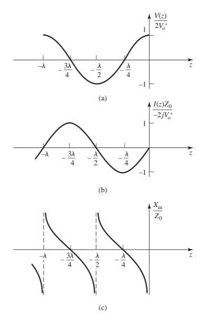
**FIGURE 2.8** (a) Voltage, (b) current, and (c) impedance  $(R_{in} = 0 \text{ or } \infty)$  variation along an opencircuited transmission line.
