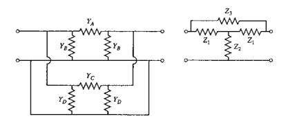
**4.11** Find the scattering parameters for the series and shunt loads shown below. Show that  $S_{12} = 1 - S_{11}$  for the series case, and that  $S_{12} = 1 + S_{11}$  for the shunt case. Assume a characteristic impedance  $Z_0$ .
