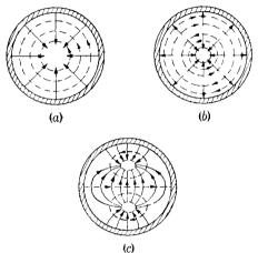
Fig. 7·13.—TM-mode in circular waveguide: (a)  $TM_{01}$ -mode [ $\lambda_{01}^{(c)} = 1.31d$ ]; (b)  $TM_{02}$ -mode [ $\lambda_{02}^{(c)} = 1.07d$ ]; (c)  $TM_{11}$ -mode [ $\lambda_{11}^{(c)} = 0.82d$ ]. ———electric field; ———magnetic field.
