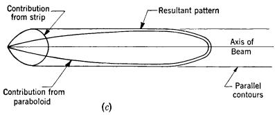
out strip; (b) central horizontal section showing strip; (c) mechanism of beam shaping.
