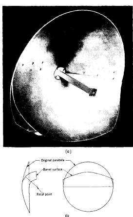
Fig. 13-17.—Barrel-reflector antenna for high-altitude beam shaping: (a) photograph; (b) drawing.
