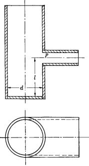
Fig. 9.33.— $TE_{10}$  to  $TM_{01}$ -mode converter
