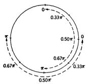
Fig. 9·10.—The effect of introducing a constant-phase difference  $-\pi/2$  on the elements of a quarter-wavelength-spaced uniform array. The inner semicircle shows the original range of z and the corresponding values of  $\theta$ . The outer semicircle is the range of z due to the phase difference; the corresponding values of  $\theta$  are indicated.
