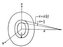
Fig. 6.9.—Division of the aperture into Fresnel zones.
