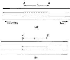
Fig. 7.5.—Cascade impedance transformers: (a) sleeve section; (b) undercut section.
