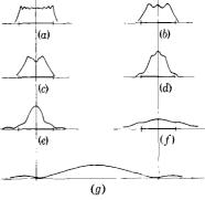
Fig. 6.2.—Transition from Fresnel to Fraunhofer diffraction for a slit; (a) . . . (f) depict the field distribution across planes in the Fresnel region at increasing distances from the slit, showing progressive diffusion of the field into the shadow region; (g) is the Fraunhofer pattern. (Reproduced from J. C. Slater and N. H. Frank, Introduction to Theoretical Physics, McGraw-Hill, New York, by courtesy of the authors.)
