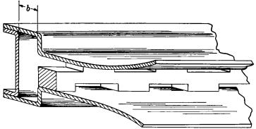
Fig. 9.55.—Transversely polarized array of waveguide radiators.
