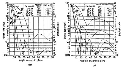
Fig. 12-8.—Principal plane patterns as a function of diameter for a series of paraboloids of  $f/D=0.25;~\lambda=4.00~{\rm in.}:~(a)~E-{\rm plane};~(b)~H-{\rm plane}.$
