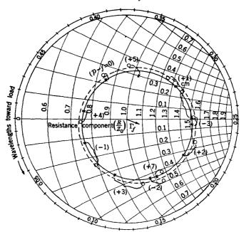
Fig. 12-12.—Variation of the reflection coefficient with position of the feed along the axis;
