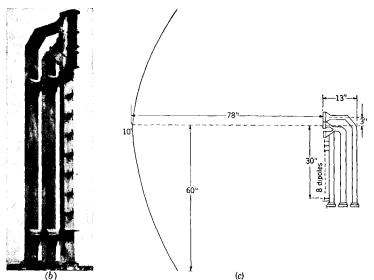
Fig. 13-15.—Cut paraboloid reflector with 11-element array feed: (a) antenna; (b) feed; (c) central vertical section.
