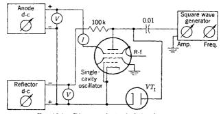
Fig. 16-1.—Diagram of a typical signal generator.
