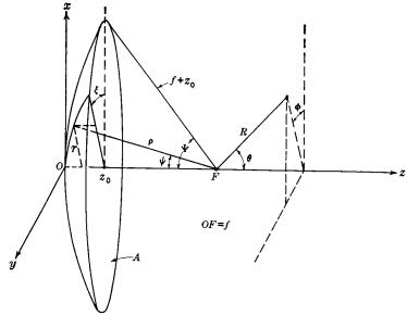
Fig. 12·1.—Geometrical parameters for the paraboloidal reflector.
