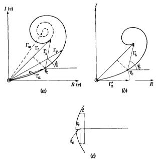
Fig. 12·14.—Elimination of the mismatch caused by the reflector: (a) reflection coefficient spiral; (b) effect of infinitely thin zone plate; (c) final position of zone plate.
