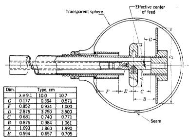
Fig. 8.10.—Dipole-disk feed assembly.
