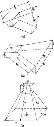
Fig. 15-19.—Electromagnetic horns: (a) E-plane sectoral horn; (b) H-plane sectoral horn; (c) pyramidal horn.
