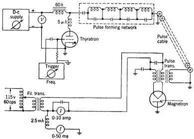
Fig. 16-7.—Schematic diagram of a magnetron signal generator.
