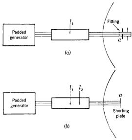
Fig. 15.2.—Short-circuited line technique for determining electrical length.
