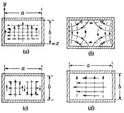
Fig. 7.9.—TE-modes in rectangular waveguides: (a)  $TE_{10}$ -mode  $[\lambda_{10}^{(c)} = 2a]$ ; (b)  $TE_{11}$ - $\operatorname{mode} \left[ \lambda_{11}^{(c)} = 2ab / \sqrt{a^2 + b^2} \right]; (c) \ TE_{20} - \operatorname{mode} \left[ \lambda_{20}^{(c)} = a \right]; (d) \ TE_{01} - \operatorname{mode} \left( \lambda_{01}^{(c)} = 2b \right),$ electric field; ---- magnetic field.
