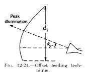
tipped so that the peak of the primary pattern makes some angle  $\psi_0$  with the paraboloid axis. The major portion of the lower section of the paraboloid is discarded. The dimension  $d_2$  is again determined from the secondary pattern beamwidth by Eq. (56). The offset feeding removes the horn and its supporting structure out of the way of the most intensely illuminated area of the aperture with resulting improvement in gain and in side-lobe characteristics.
