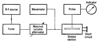
Fig. 15.5.—Block diagram for calibration of detector.
