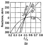
Fig. 8-8.—Input impedance of spheroidal dipoles with major axis L and minor axis D:
