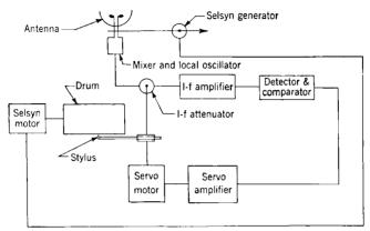
Fig. 16-18.- Antenna pattern recorder utilizing an r-f attenuator in a heterodyne circuit
