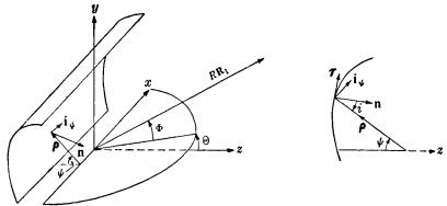
Fig. 5-9.—The cylindrical reflector with a line-source feed.
