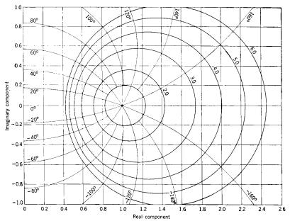
Fig. 2.9.—The bipolar impedance chart.
