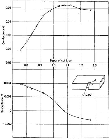
Fig. 9.22.—Admittance of a 15° inclined slot on narrow edge of rectangular waveguide. The waveguide dimensions are  $1\frac{1}{4}$  by  $2\frac{1}{4}$  in.,  $\lambda=10.7$  cm., and the width of the slot is  $\frac{1}{4}$  in. (From the work of J. W. Dodds, E. W. Guptill, and W. H. Watson by permission of the National Research Council of Canada.)
