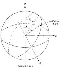
Fig. 15.9.—Coordinate system for primary patterns.
