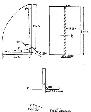
Fig. 12:27.—Half-beacon antenna.
