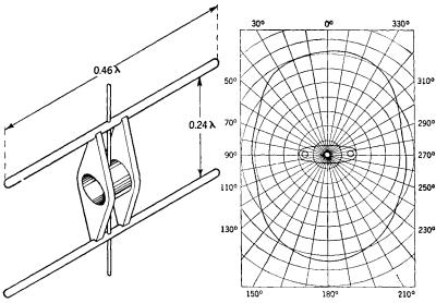
Fig. 9-40. — Longitudinally polarized streamlined radiator (*H*-element).
