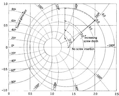
Fig. 15-4.—Admittance diagram for capacitive screw. Increasing screw depths correspond to increasing capacitance in parallel.
