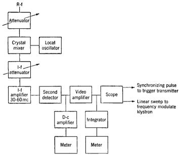
Fig. 16-14.—Block diagram of heterodyne receiver.
