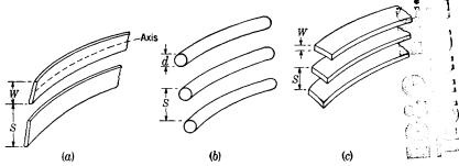
Fig. 12:17.—Grating reflectors: (a) broadside strips; (b) round bars; (c) edgewise strips.
