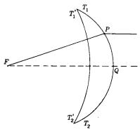
Fig. 11-4.—One-surface lens with elliptical contour,
