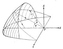
Fig. 13·33.—Double curvature surface and spherical coordinate system.
