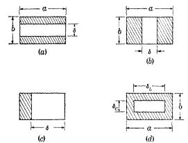
Fig. 7:11.—Windows for rectangular guides; (a) symmetrical capacitative; (b) symmetrical inductive; (c) asymmetrical inductive; (d) resonant.
