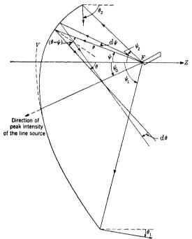
Fig. 13-30.—Geometry of ray reflection at surface of reflector.
