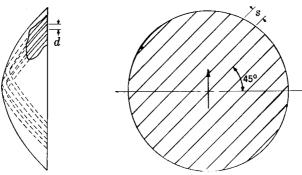
Fig. 12-15.—Quarter-wave grating to rotate the polarization of the electric vector and eliminate the mismatch.
