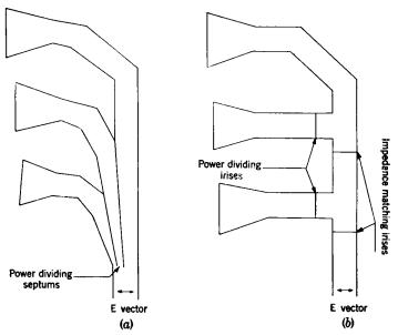
Fig. 13-27.—Multiple horn feeds for illuminating a cut paraboloid: (a) multiple Y-junction; (b) successive T-junctions.
