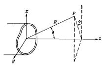
Fig. 10·1.—Coordinate system used in discussing radiation from open waveguide.
