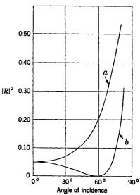
Fig. 11·10.—Fraction of incident power reflected from the surface of an infinite dielectric slab vs. angle of incidence: (a) electric vector perpendicular to the plane of incidence; (b) electric vector in the plane of incidence; n = 1.6.
