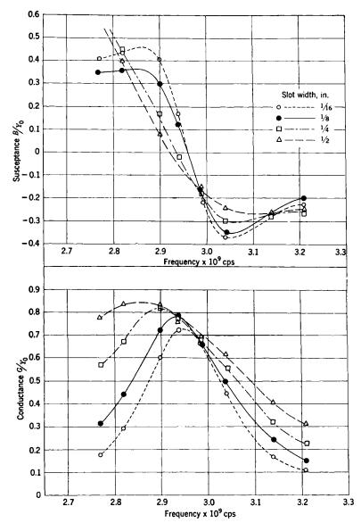
Fig 9-19.—Admittance of longitudinal slot as a function of frequency (center of slot is 1.98 cm from the center of the waveguide). (From the work of J. W. Dodds and W. H. Watson by permission of the National Research Council of Canada.)
