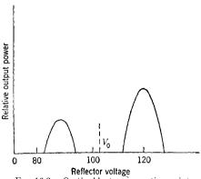
Fig. 16.3.—On the klystron operating point.
