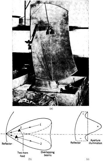
Fig. 13:10.—Two-element array and paraboloid for producing sector shaped beam: (a) antenna; (b) overlapping beams; (c) aperture illumination.
