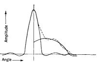
Fig. 13:32.—Superposition of barrel and paraboloidal amplitude patterns.
