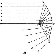
Fig. 13.9.—Reflector modifications for producing an asymmetrical flared beam:
