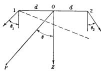
Fig. 10·32.—Phase distortion in the fields of primary feeds of low directivity.
