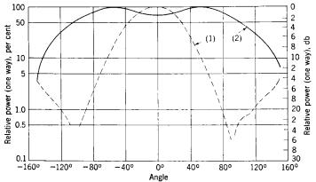
Fig. 10-31.—Primary patterns of (1) an open waveguide and (2) a cut corner waveguide  $(\phi = 63.4^{\circ} \text{ and } C = \frac{1}{3})$ .
