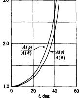
Fig. 11.5.— $A(\rho)/A(\theta)$  for a spherical lens and  $A(y)/A(\theta)$  for a cylindrical lens with elliptical contours; n = 1.6.
