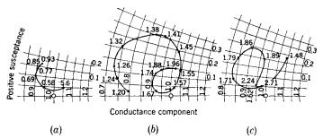
Fig. 10:21.—Admittances of three 15° electric plane horns of different lengths as a function of wavelength: (a)  $r_2-r_1=10.6$  cm,  $\lambda$  varied from 9.0 to 11.5 cm with best match at 11.4 cm; (b)  $r_2-r_1=22.8$  cm,  $\lambda$  varied from 9.1 to 11.5 cm with best match at 10.1 cm; (c)  $r_2-r_1=26.3$  cm,  $\lambda$  varied from 8.1 to 11.5 cm with best match at 10.9 cm.
