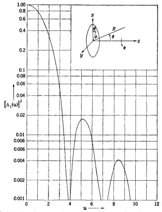
Fig. 6.7.—Secondary pattern from a uniformly illuminated circular aperture.
