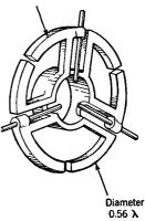
Fig. 9.28.—Tridipole radiator.
