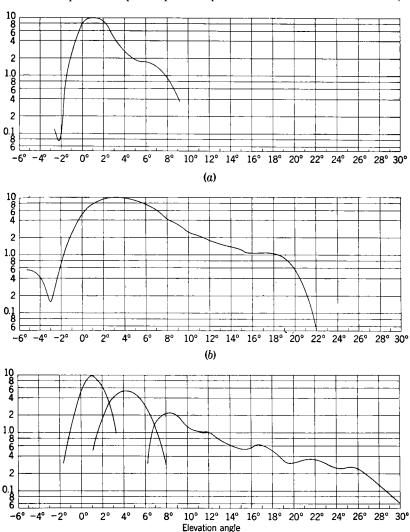
Fig. 13·16.—Elevation patterns obtained with cut paraboloid reflectors and linear-array feeds: (a) two-element array of Fig. 13·13; (b) four-element array of Fig. 13·14; (c) eleven-element, three-transmitter array of Fig. 13·15.
