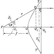
Fig. 11:2. - One-surface lens with hyperbolic contour.
