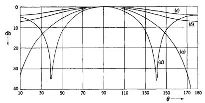
Fig. 9.8.—Array factors of four broadside arrays whose lengths are  $\lambda/2$ : (a) the two-element  $\lambda/2$ -spaced uniform array  $\cos^2\left(\frac{\pi}{2}\cos\theta\right)$ ; (b) the four-element  $\lambda/6$ -spaced uni-
