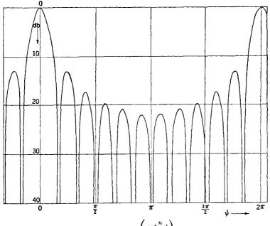
Fig. 9-5.—The function  $\frac{\left(\sin^2\frac{n}{2}\psi\right)}{\left(n^2\sin^2\frac{1}{2}\psi\right)}$  for n=12.
