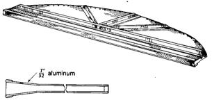
Fig. 12-30.- Structural design of a pillbox.
