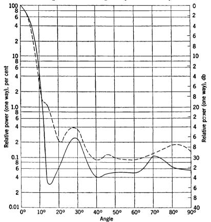
Fig. 12-10.—Principal plane patterns of 30-in.-diameter paraboloid (f/D = 0.354)illuminated by the dipole-disk feed;  $\lambda = 10 \text{ cm}$ ; —— E-plane; —— H-plane;  $\Theta_E = 10.2^\circ$ ;  $\Theta_H = 9.5^{\circ}$ .
