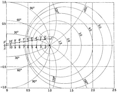
Fig. 9.48.—Input impedance of 10-element resonant array.
