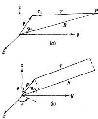
Fig. 3.5.—On the far-zone field: (a) arbitrary field point P; (b) simplifying relationships for a point in the far zone.
