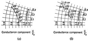
Fig. 10·18.—Throat admittance as a function of flare angle and frequency: (a)  $\lambda = 10$  cm,  $\theta_0$  varied; (b)  $\lambda$  varied for flare angles of 15° and 30°.
