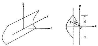
Fig. 12-25.--Parabolic cylinder and line source.
