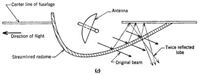
Fig. 14.9.—Mechanisms by which radome wall reflections can distort patterns: (a) secondary source produced by focused reflections; (b) wide-angle lobe produced by reflection from the upper portion of a radome; (c) wide-angle lobe produced by a double reflection involving the undersurface of the fuselage.
