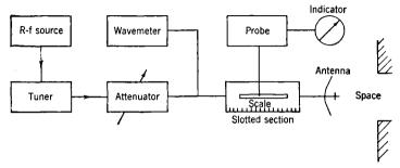
Fig. 15-1.—Block diagram of impedance-measurement apparatus.
