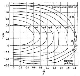
Fig. 12-22.—Constant intensity contours in paraboloid aperture (horn feed axis tilted 20° relative to paraboloid axis).
