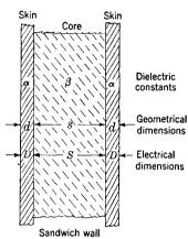
Fig. 14·15.—Sandwich-wall design. The figure serves to define symbols used in the text.
