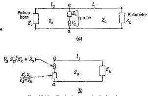
Fig. 15-12.-Equivalent circuit of r-f probe.
