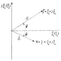
Fig. 2.8.— The relation between impedance and admittance.
