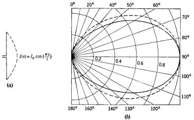
Fig. 3-12.—The half-wave dipole: (a) current distribution along the wire; (b) meridional polar diagram compared with that of the electric dipole:  $-\frac{\lambda}{2}$  dipole, --- infinitesimal dipole.
