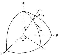
Fig. 3-3.—Spherical coordinates.
