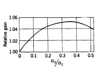
Fig. 10-26.—Relative gain of a box horn vs.  $a_3/a_1$ .
