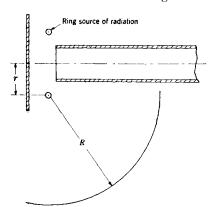
Fig. 10-6.—Circular waveguide and reflecting disk showing position of ring source of radiation.
