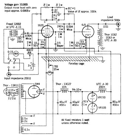
Fig. 16-12. - Tuned audio amplifier.
