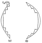
Fig. 11·7.—Zoning of nonrefracting lens surfaces.
