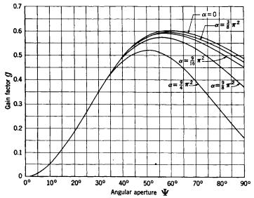
Fig. 12.6.—Phase-error effects on gain.
