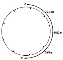
Fig. 9-3.—The location of the zeros of  $f(z) = 1 + z + z^2 + \cdots + z^8$ . The range of z for  $s = \lambda/4$  is also shown together with a few of the corresponding values of  $\theta$ .
