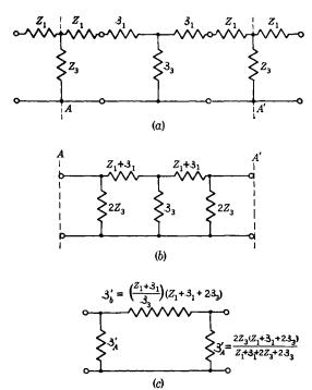
Fig. 9-42.—Network system equivalent to a loaded transmission line: (a) T-section replacements of radiators and line segments; (b) reduction to symmetrical networks; (c)  $\Pi$ -section equivalent of the network in (b).
