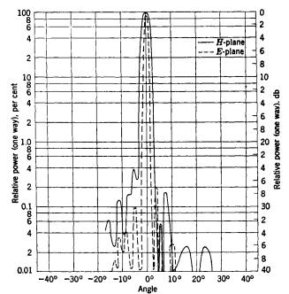
Fig. 12-24.—Principal E- and H-plane polar diagrams of the antenna shown in Fig. 12-23.
