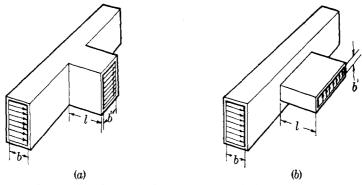
Fig. 9.25.—Waveguide radiators: (a) longitudinally polarized; (b) transversely polarized.
