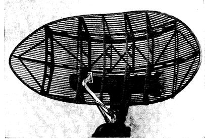
Fig. 12-23.—Fanned-beam antenna using the offset feed technique.
