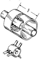
Fig. 9-34.—Longitudinally polarized axially symmetrical radiating unit.
