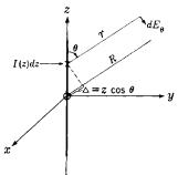
Fig. 3:11.—Far-zone field of a linecurrent distribution.
