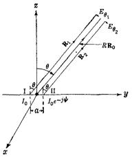
Fig. 3.14.—The double-dipole system.
