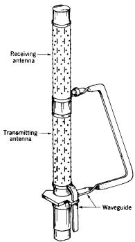
Fig. 9.53.—Beacon antenna with an external feed line.
