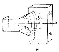
Fig. 10-23.—Box horn: (a) direct junction type; (b) sectoral guide junction type.
