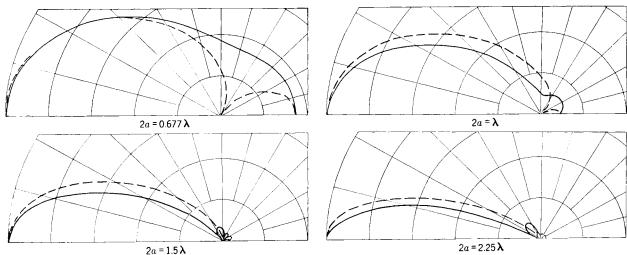
Fig. 10·2.—Circular waveguide radiation patterns for the TE<sub>11</sub>-mode as a function of aperture (—— E-plane; - - - H-plane); 2a is the inside diameter of the guide. (Courtesy of L. J. Chu and the American Institute of Physics.)
