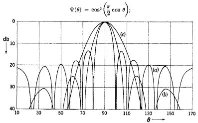
Fig. 9.7.—Array factors for three 11-element  $\lambda/2$ -spaced arrays: (a) the uniform array
