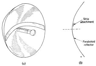
Fig. 13-19.—Strip-reflector antenna for low-altitude beam: (a) autenna; (b) central vertical section of reflector.
