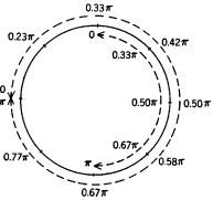
Fig. 9.9.—The range of  $\psi$ , the angle of z, as  $\theta$  varies from 0 to  $\pi$ . The outer ring of figures shows corresponding values of  $\theta$  at various points on the unit circle in the z-plane for  $s = \lambda/2$ . The inner set of figures shows values of  $\theta$  for  $s = \lambda/4$ .
