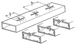
Fig. 9.23.—Probe-fed slots on rectangular waveguide. The arrows show lines of current flow.
