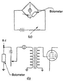
Fig. 16.9.—Common bolometer circuits.
