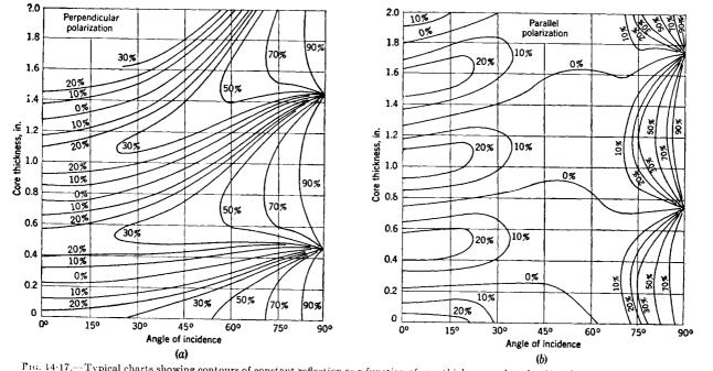
Fig. 14:17,--Typical charts showing contours of constant reflection as a function of core thickness and angle of incidence for the following conditions:  $\lambda_0 = 3.2 \text{ cm}$ ; core  $\epsilon'/\epsilon_0 = 1.4$ ; skin  $\epsilon'/\epsilon_0 = 3.7$ ; skin thickness = 0.050 in. (a) Polarization perpendicular to the plane of incidence; (b) parallel polarization.
