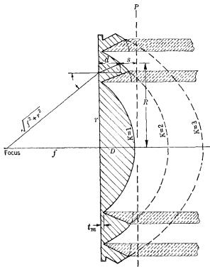
Fig. 11.8.—Zoned two-surface lens.
