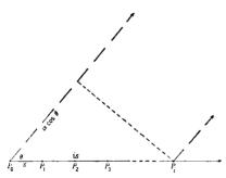
Fig. 9·1.—Difference in distance from the *i*th element and from the pole to a distant point in the direction  $\theta$ ,  $\phi$ .
