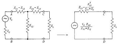
Fig. 2-4.—Thévenin's theorem and the maximum-power transfer condition.
