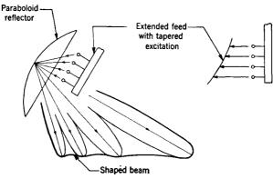
Fig. 13.8.—Formation of a shaped beam by means of a feed array in a paraboloid reflectorprocess; the rays emerging from the aperture will not all be collimated
