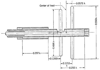
Fig. 8:13.—Double-dipole feed on coaxial line.
