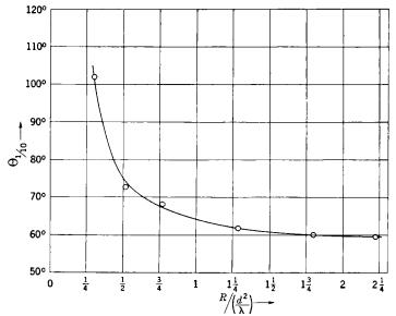
Fig. 15-8.—Tenth-power width  $\Theta_{30}$  as a function of the path distance R between test horn and pickup horn.
