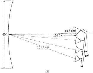
Fig. 13·14.—Cut paraboloid reflector with four-horn array feed: (a) antenna; (b) central vertical section.
