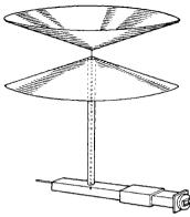
Fig. 1.3.—The biconical horn.
