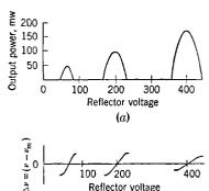
Fig. 16·2.—Operating characteristics of a reflex klystron: (a) variation in output r-f power with voltage; (b) change in output frequency with respect to the frequency  $\nu_m$  of the maximum power of the mode.
