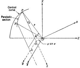
Fig. 13-34.—Surfaces of parabolic section.
