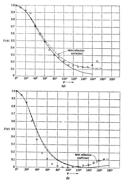
Fig. 10·4.—Theoretical and observed radiation patterns from rectangular waveguide;  $\lambda=3.2~{\rm cm}; \frac{a}{\lambda}=0.71; \frac{b}{\lambda}=0.32;$ ——calculated patterns;  $\bigcirc$  observed values; (a) *E*-plane; (b) *H*-plane.
