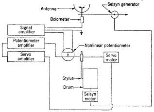
Fig. 16-15.—Audio antenna pattern recorder.
