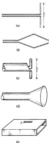
Fig. 1-2. -Transmission lines and radiating elements. (a) Center-driven half-wave dipole; (b) rhombic antenna terminating a two-wire line; (c) microwave dipole terminating a coaxial line; (d) conical horn fed by a circular waveguide; (c) slot radiator in the wall of a rectangular guide.
