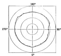
Fig. 9.32.—Pattern of circular array of seven slots on circular waveguide with 1¼ in. OD.
