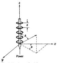
Fig. 9.26.—Array of axially symmetrical radiators.
