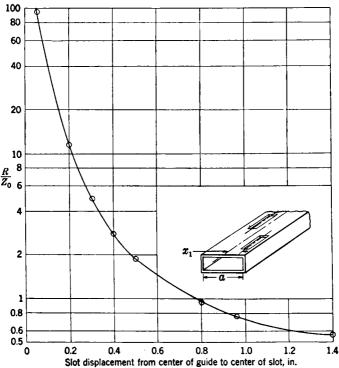
Fig. 9-18.—Resistance offered by a longitudinal slot as a function of its displacement from the center. The slot dimensions are  $\frac{1}{6}$  by 2 in., the waveguide is  $1\frac{1}{2}$  by 3 in.,  $\lambda=10.7$  cm. The data fit the relation  $G=Z_0/R=1.73 \sin^2{[(\pi x/a)1]}$ . (From J. W. Dodds, E. W. Guptill, and W. H. Watson by permission of the National Research Council of Canada.)
