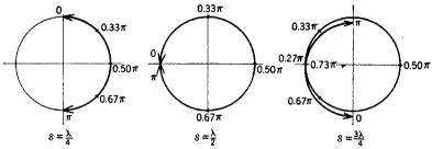
Fig. 9-2.—The portion of the unit circle in the complex plane that is the range of z. The real axis is horizontal. The figures on the perimeter show the corresponding values of  $\theta$  for certain values of z.
