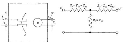
Fig. 2-11.—Four-terminal network representation of the coupled transmitter-receiver.
