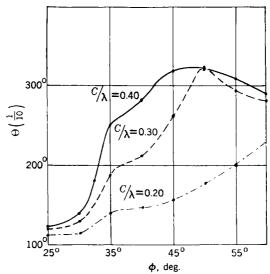
Fig. 10-30.—10-db widths of the pattern obtained with the device of Fig. 10-29 as a function of  $C/\lambda$  and  $\phi(\lambda=3.2 \text{ cm}, a=0.900 \text{ cm}, b=0.400 \text{ cm}, d=0.063 \text{ cm})$ .
