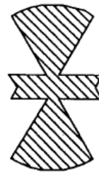
Shunt Radial Stub
