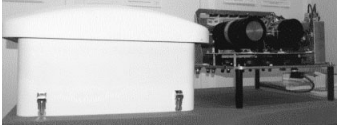
FIGURE 12.5 Tower-mounted transceiver with HTS microstrip duplexers and filters for mobile base station application.
