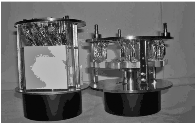
FIGURE 11.39 Inside views of the cryogenic rf housings (microenclosures) inside 2004 Dewar (left) and 2008 Dewar (right). The 2008 Dewar has been optimized to eliminate parts as compared to the 2004 design. (Taken from [114], ©2009 IEEE.)
