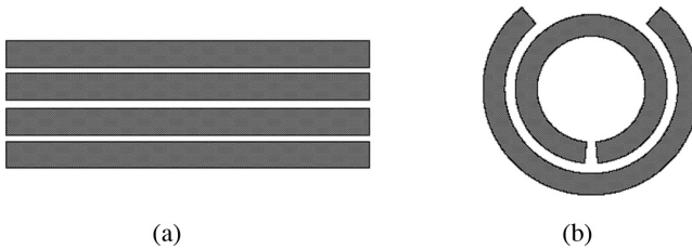
FIGURE 11.38 (a) Four-element split-line resonator. (b) Two-element split-ring resonator.
