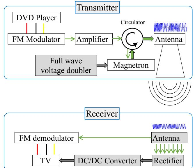
Fig. 1 Wirelessly-powered TV system diagram.
