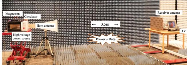
Fig. 5 Photo of the wirelessly-powered TV.
