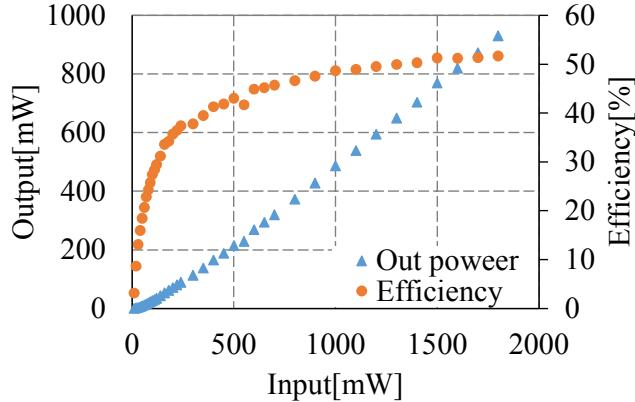
Fig. 4 Rectifier efficiency of the rectifier circuit with different input power(load:60Ω)
